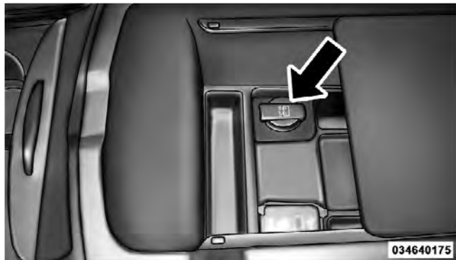
Center Console Power Outlet
