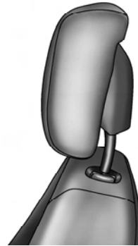
Active Head Restraint (Normal Position)
