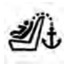
In addition, there are tether strap anchorages behind each rear seating position located in the panel between the rear seatback and the rear window. These tether strap anchorages are under a plastic cover with the tether anchorage symbol on it.
