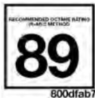
The 3.6L and 5.7L engine (with automatic transmission) is designed to meet all emissions regulations and provide satisfactory fuel economy and performance when using high-quality unleaded gasoline having an octane range of 87 to 89. The manufacturer recommends the use of 89 octane for optimum performance. The use of premium gasoline is not recommended, as it will not provide any benefit over regular gasoline in these engines.
