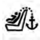
In addition, there are tether strap anchorages behind each rear seating position located in the panel between the rear seatback and the rear
