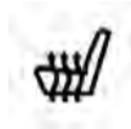
Press the “Driver” or “Pass” seat soft-key (located on the Uconnect® screen) once to select HI-level heating. Press the soft-key a second time to select LO-level heating. Press the soft-key a third time to shut the heating elements OFF.
