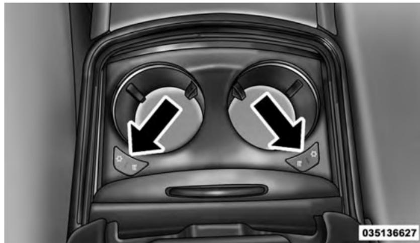
Heated And Cooled Cupholder Switches
