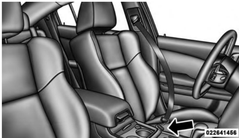
Inserting Latch Plate Into Buckle
