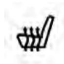
Press the switch once to select HI-level heating. Press the switch a second time to select LO-level heating. Press the switch a third time to shut the heating elements OFF.
