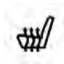
Press the “Driver” or “Passenger” seat soft-key once to select HI-level heating. Press the soft-key a second time to select LO-level heating. Press the soft-key a third time to shut the heating elements OFF.
