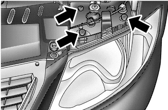
2. Turn the bulb socket retaining ring or the bulb assembly counterclockwise.
