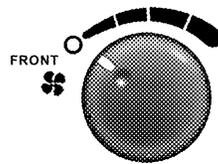
The fan speed increases as you move the control clockwise.
