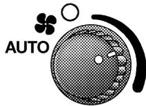
The rear blower control, located in the headliner near the center of the vehicle has an “OFF”, “AUTO” and a range of blower speeds.
