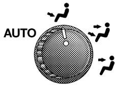
The Rear Mode Control, located in the headliner near the center of the vehicle can be used to select between Auto, Headliner, Bi-Level and Floor modes.
