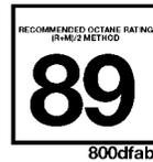
The 3.5L and 5.7L engines are designed to meet all emissions regulations and provide satisfactory fuel economy and performance when using high-quality unleaded gasoline with an octane rating of 87 to 89.
