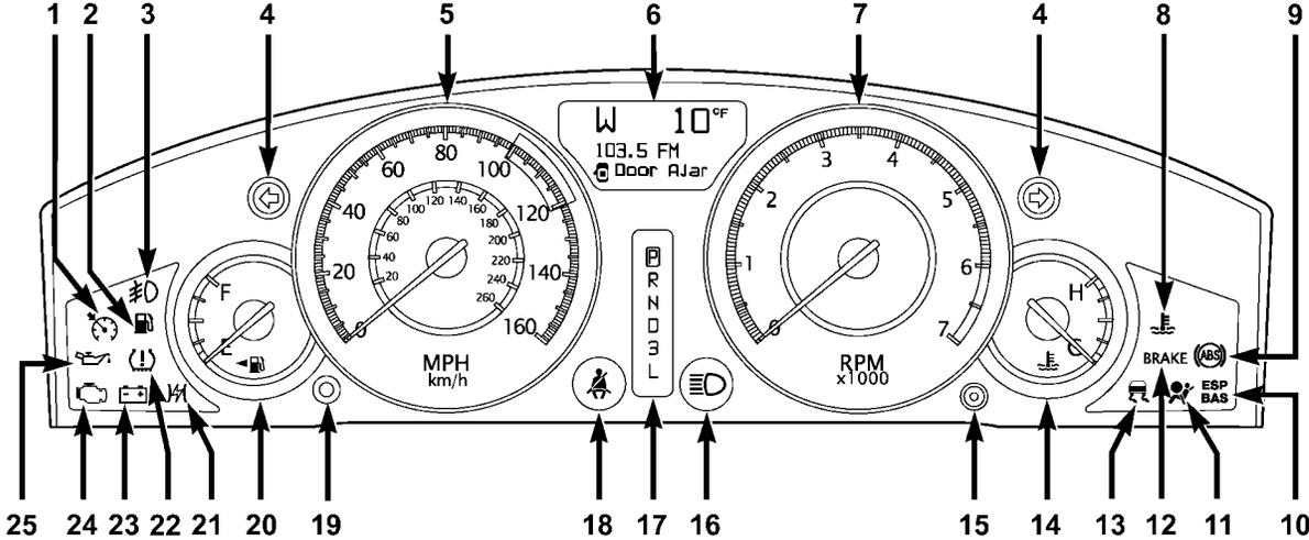
**INSTRUMENT CLUSTER DESCRIPTIONS****1. Electronic Speed Control Indicator Light — If Equipped**
