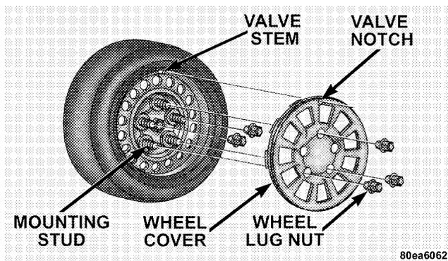
1. Tighten the two lug nuts on the mounting studs on each side of the stud which is in alignment with the valve stem.
