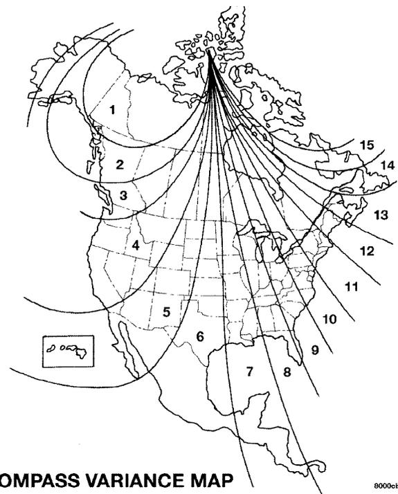
**To set the variance:** Turn the ignition switch ON. Then, press and hold the compass button for approximately 2 seconds. Then, press the SCROLL button until “Compass Variance” displays in the EVIC. Both the “Compass Variance” message and the last variance zone number will display in the EVIC. Then, press and release FUNCTION SELECT button until the proper variance zone is selected according to the map. Finally, press and release the compass button to exit.
