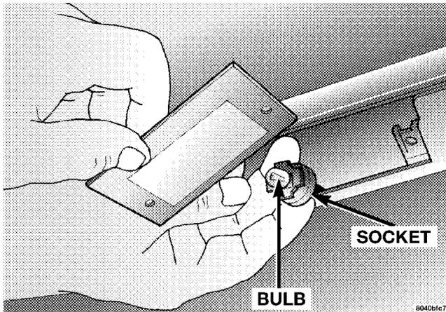
3. Replace the bulb and reinstall the bulb and socket assembly.
