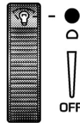
Rotate the dimmer control completely upward to the second detent to turn on the interior lights. The interior lights will remain on when the dimmer control is in this position.
