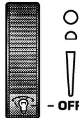
Rotate the dimmer control to the extreme bottom "OFF" position. The interior lights will remain off when the doors are open.
