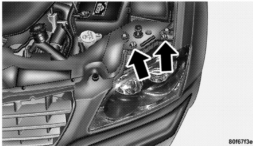
2. Twist the bulb socket to remove from the headlight module and pull the bulb from socket.
