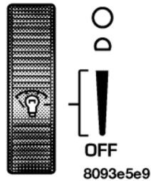
With the parking lights or headlights on, rotating the dimmer control for the interior lights on the Multi-Function Lever upward will increase the brightness of the instrument panel lights.
