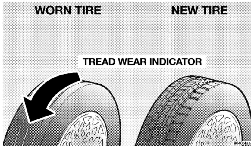
These indicators are molded into the bottom of the tread grooves and will appear as bands when the tread depth becomes 1/16 inch (2 mm). When the tread is worn to the tread wear indicators, the tire should be replaced.
