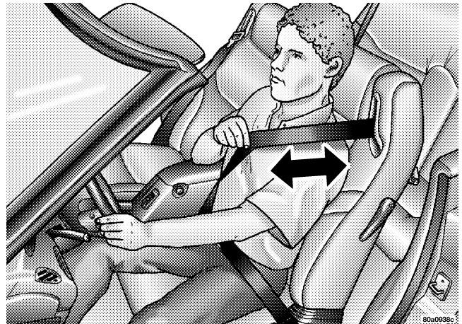
Removing Slack From Belt
