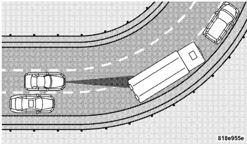
ACC may occasionally provide braking and/or a driver alert that you consider unnecessary. This may be the system's response to signs, guardrails, and other stationary objects in a curve. This may also occur at the base of dramatic hills. This is normal operation and your vehicle does not require service.
