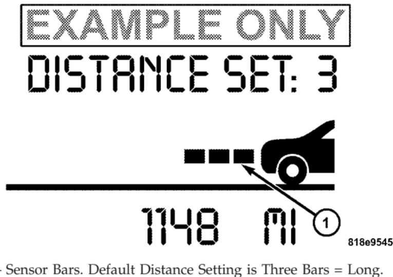
To change the distance setting, push the lever away from you (DISTANCE) and release. Each time this is done, the distance setting adjusts between long, medium, and short.
