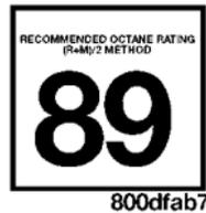
The 3.5L and 5.7L engines are designed to meet all emissions regulations and provide satisfactory fuel economy and performance when using high-quality unleaded gasoline having an octane range of 87 to 89. The manufacturer recommends the use of 89 octane for optimum performance. The use of
