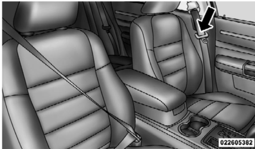
Pulling Out the Lap/Shoulder Belt Latch Plate
