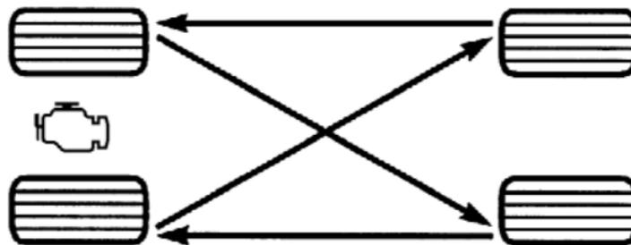
Follow the recommended tire rotation frequency for your type of driving found in the “Maintenance Schedules” section of this manual. More frequent rotation is permissible if desired. The reasons for any rapid or unusual wear should be corrected prior to rotation being performed.
