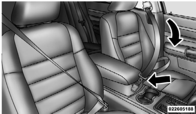
Inserting Latch Plate into Buckle
