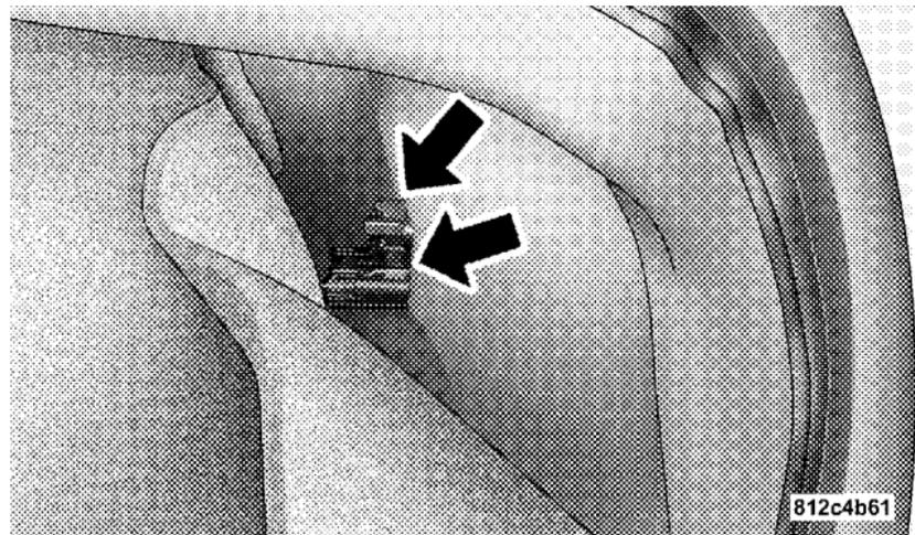
7. Pull the tail light assembly clear from the vehicle to access the bulbs. Turn bulb sockets counterclockwise to remove.
