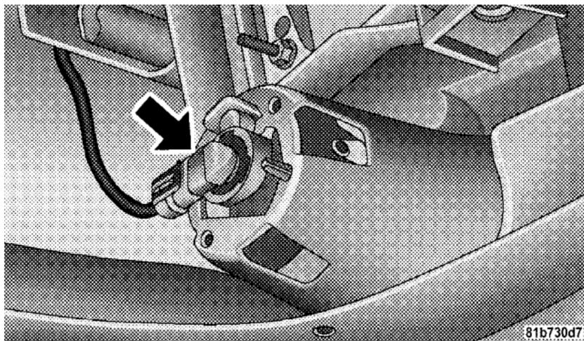
2. Remove the bulb from the connector socket and install the replacement bulb.
