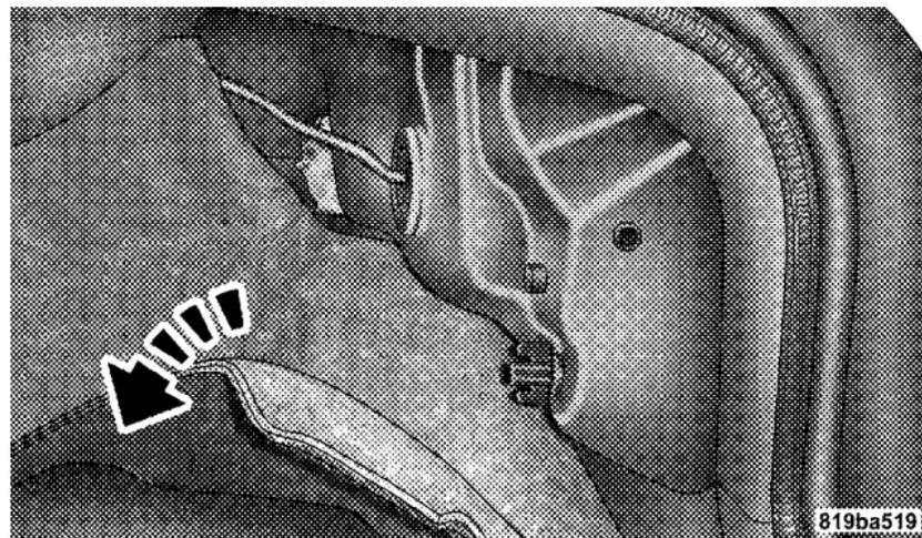
2. Remove the two plastic wing nuts from the taillight housing.
