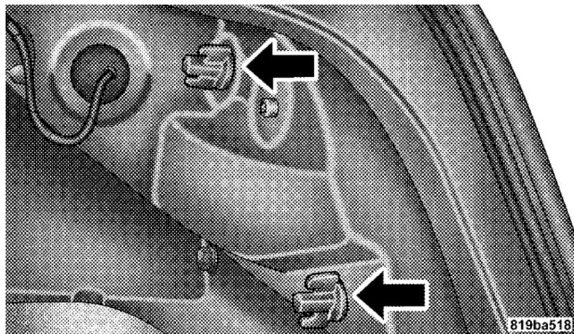
3. Grasp the taillight housing and pull it firmly outward while pushing gently on the studs from inside to disengage the housing from the vehicle.
