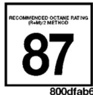
The 2.4L and 2.7L engines are designed to meet all emission regulations and provide excellent fuel economy and performance when using high quality unleaded “regular” gasolines having an octane rating of 87. The use of premium gasoline is not recommended. Under normal conditions, the use of premium gasoline will not provide a benefit over high quality unleaded “regular” gasolines, and in some circumstances may result in poorer performance.
