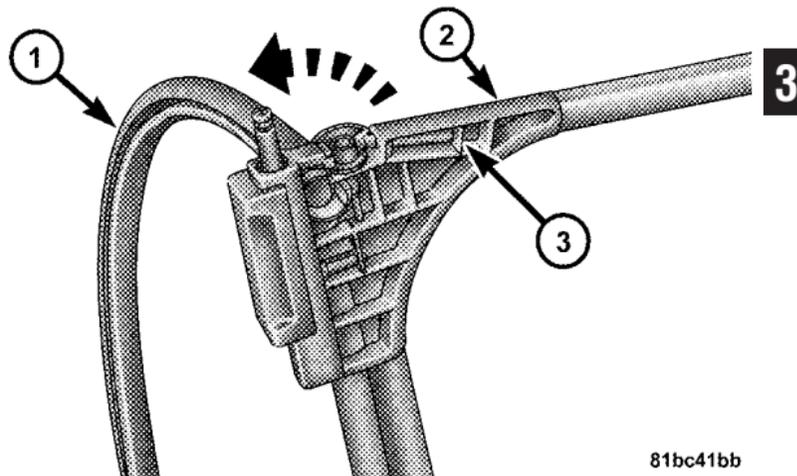
5. Unfold both stems at the rear of the large frame.
