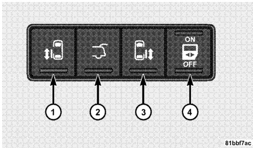
**Overhead Console Power Sliding Door Master Switch**
