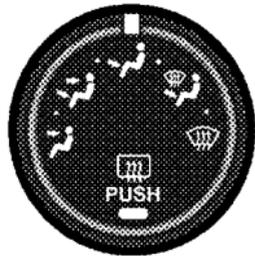
Mode control allows you to choose from several selections of air distribution. You can select either a primary mode, as identified by the symbols, or a blend of two of these modes. The closer the control is to a particular mode, the more air distribution you receive from that mode.
