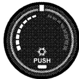
Use this control to regulate the temperature of the air inside the passenger compartment. Rotating the knob counterclockwise, from top center into the blue area indicates cooler temperatures. Rotating the knob clockwise, into the red area, indicates warmer
