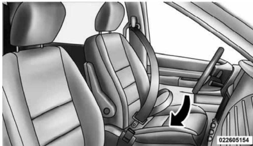
**Inserting Latch Plate into Buckle**
