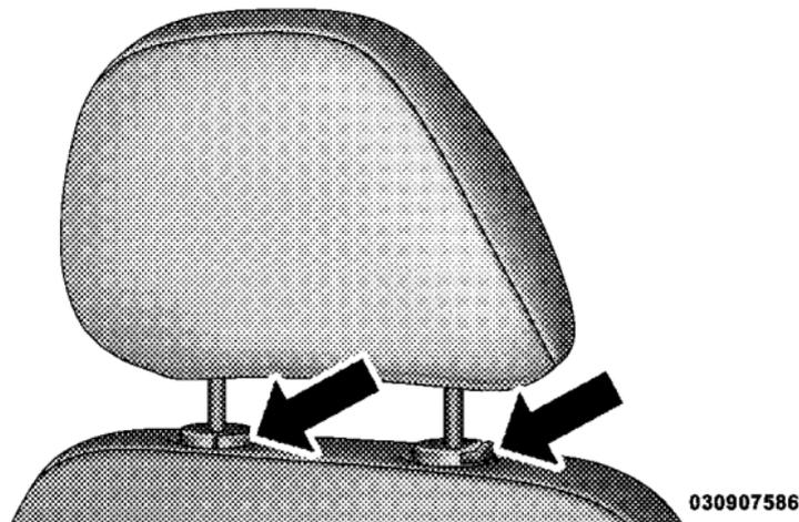
Removing Head Restraint
