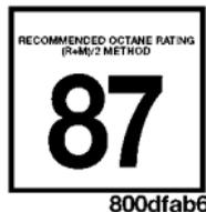
The 2.7L engine is designed to meet all emissions regulations and provide excellent fuel economy and performance when using high-quality unleaded “regular” gasoline having an octane rating of 87. The use of premium gasoline is not recommended, as it will not provide any benefit over regular gasoline in these engines.
