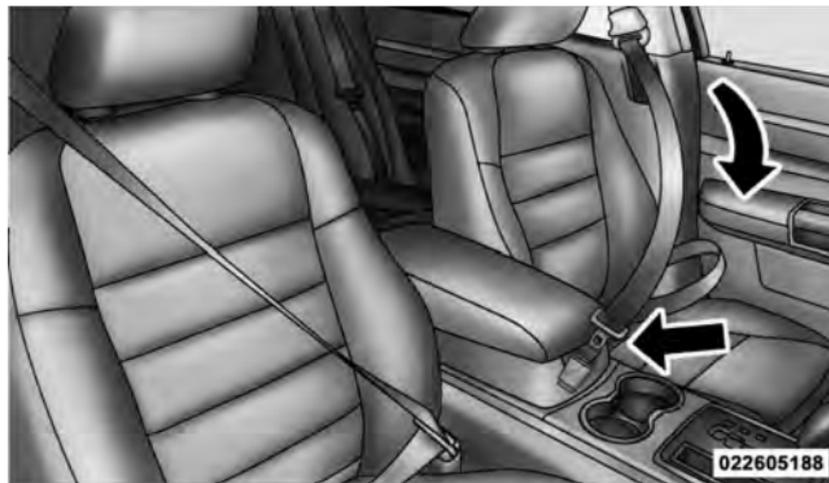
Inserting Latch Plate into Buckle
