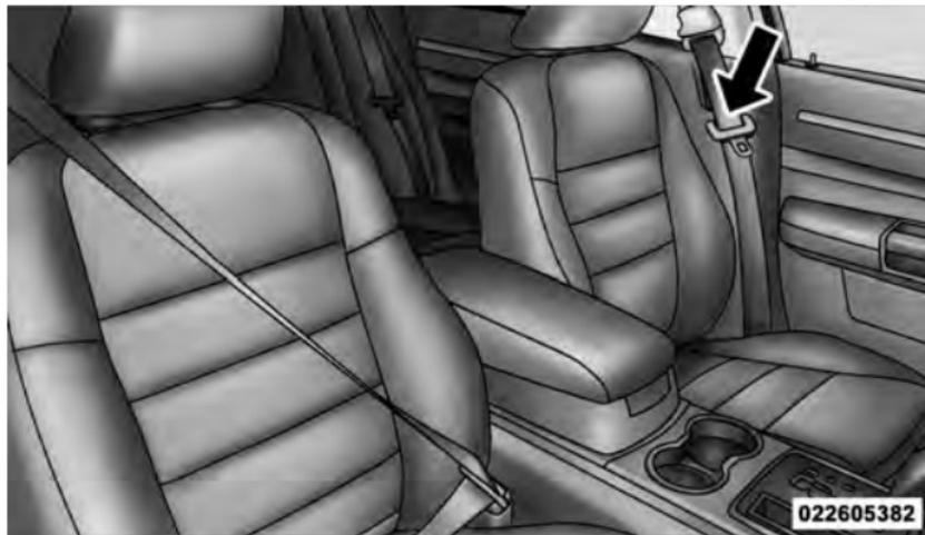
Pulling Out the Lap/Shoulder Belt Latch Plate
