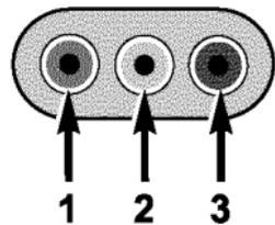
Audio/Video RCA Jacks (AUX Jacks) on the rear of the center console enable the monitor to display video directly from a video camera, connect video games for display on the screen, or play music directly from an MP3 player.
