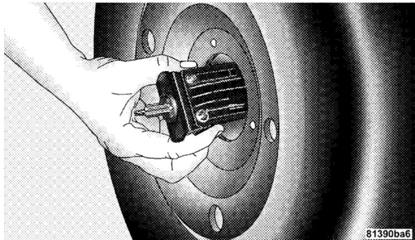
Squeezing Winch Retainer Tabs
