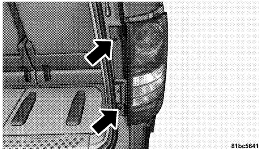
Tail Lamp Housing Fastener Removal
