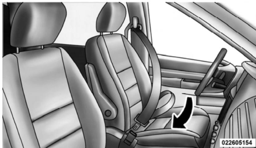
Inserting Latch Plate into Buckle
