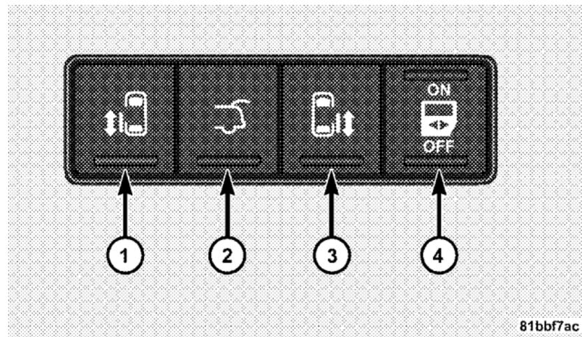
Overhead Console Power Sliding Door Master Switch
