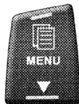
EVIC Menu / Step Control Button, as it appears on the left side of the steering wheel spoke.
