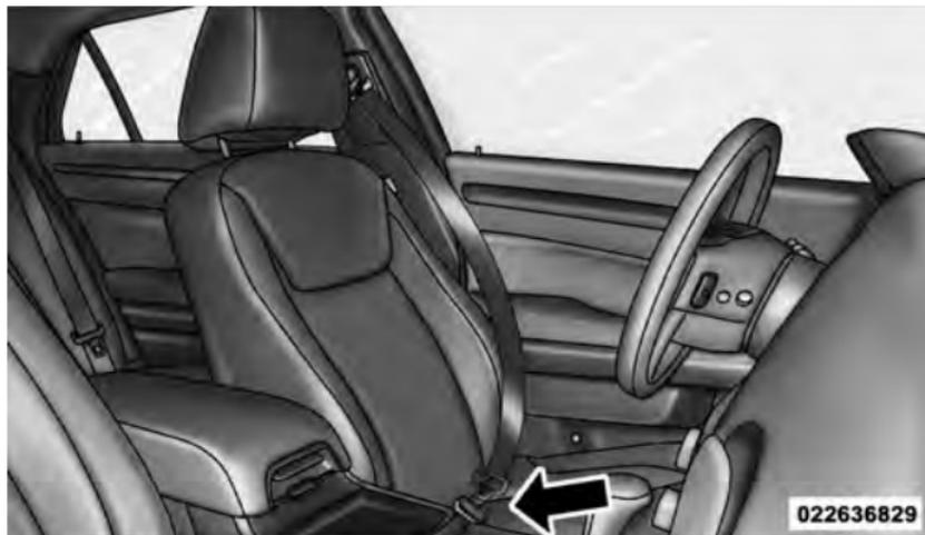
Inserting Latch Plate Into Buckle
