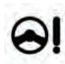
If the “SERVICE POWER STEERING SYSTEM” message and a flashing icon are displayed on the EVIC screen, it indicates that the vehicle needs to be taken to the dealer for service. It is likely the vehicle has lost power steering assistance. Refer to “Electronic Vehicle Information (EVIC)” in “Understanding Your Instrument Panel” for further information.
