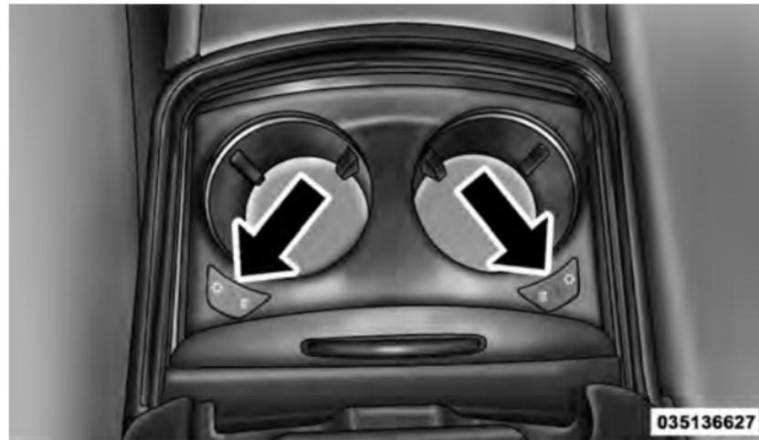
**Heated And Cooled Cupholder Switches**
