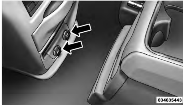
Instrument Panel Outlets
