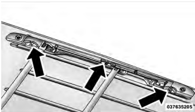
Rail Tie Loops
