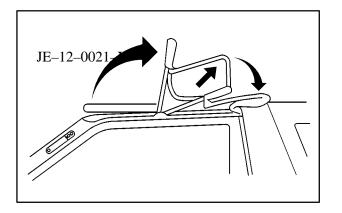
4. Swing the front top bow up and back while folding the canvas top out from between the top bow and the roof support. Be sure that you don't pinch the canvas top between the front top bow arms and the roof rails.
