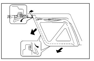
4. Unzip the zipper the rest of the way and remove the side window.
