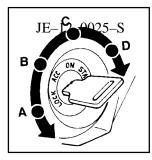
With the key in the ignition switch, you can turn the switch to four positions. **LOCK** (A): This is the only position in which you can remove the key. This locks your steering wheel, ignition and automatic transmission.
