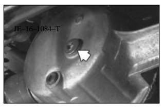
If the level is below the bottom of the filler plug hole, you may need to add some lubricant.
