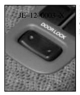
If you have power door locks, the switch is located on the driver's and passenger's door armrest.
