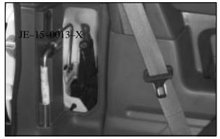
The jacking equipment you'll need is stored in the luggage compartment on the driver's side of the vehicle.
