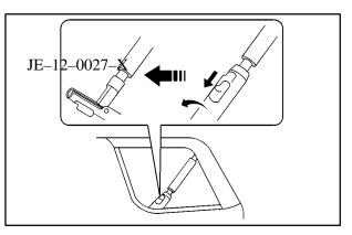
4. Push the release latches on both sides of the vehicle down to release the rear support arms. With the latches released, pull up on the arms at the hinges to release the tension on the canvas top.
