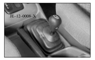
The transfer case shift lever is on the floor to the right of the driver. Use this lever to shift into and out of four-wheel drive. An indicator light comes on when the transfer case is in FOUR-WHEEL HIGH (4H) or FOUR-WHEEL LOW (4L). **TWO-WHEEL HIGH (2H):** This setting is for driving in most street and highway situations. Your front axle is not engaged in two-wheel drive.
