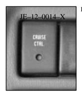
1. Press the CRUISE CTRL. switch on the instrument panel to turn the system on. The indicator light on the switch will come on.
