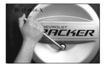
2. Using the wheel wrench, remove the wheel nut from the tire. Gently pry the spare tire cover off the wheel.
