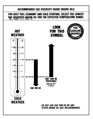
As shown in the chart, SAE 10W-30 is best for your vehicle. However, you can use SAE 5W-30 if it's going to be colder than  $60^{\circ}$ F ( $16^{\circ}$ C) before your next oil change. When it's very cold, you should use SAE 5W-30. These numbers on an oil container show its viscosity, or thickness. Do not use other viscosity oils, such as SAE 20W-50.
