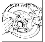
5. Remove any rust or dirt from the wheel bolts, mounting surfaces and spare wheel.
