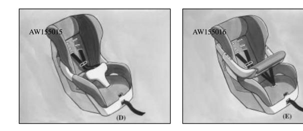
A forward-facing child restraint (C-E) positions a child upright to face forward in the vehicle. These forward-facing restraints are designed to help protect children who are from 20 to 40 lbs. (9 to 18 kg) and about 26 to 40 inches (66 to 102 cm) in height, or up to around four years of age. One type, a convertible restraint, is designed to be used either as a rear-facing infant seat or a forward-facing child seat.
