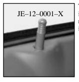
To lock the door from the inside, push down the lock rod on the door. To unlock it, pull up on the lock rod.
