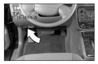
This fuse box is under the left side of the instrument panel. The fuses here protect each separate circuit including headlamps. If you have electrical failure, check here first.
