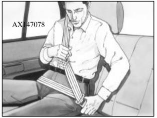
3. To make the lap part tight, pull down on the buckle end of the belt as you pull up on the shoulder part.
