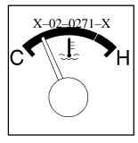
This gage shows the engine coolant temperature. If the gage pointer moves to the H (red) side, your engine is too hot.
