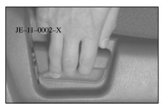
To adjust the seatback, lift the lever on the outer side of the seat. Release the lever to lock the seatback where you want it. Pull up on the lever, and the seat will go to its original upright position.
