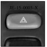
Press the button on the instrument panel to make your front and rear turn signal lamps flash on and off.
