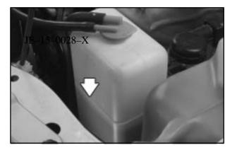
The coolant level should be at or above FULL. If it isn't, you may have a leak in the radiator hoses, heater hoses, radiator, water pump or somewhere else in the cooling system.
