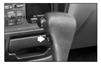
The Overdrive Off switch is located on the left side of the shifter. By operating the Overdrive Off switch, the four-speed automatic transmission (three-speed plus overdrive) can be converted to a three-speed automatic transmission. While in the three-speed mode, the transmission will not shift into the Overdrive position.
