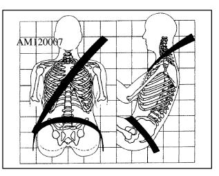
The lap part of the belt should be worn low and snug on the hips, just touching the thighs. In a crash, this applies force to the strong pelvic bones. And you'd be less likely to slide under the lap belt. If you slid under it, the belt would apply force at your abdomen. This could cause serious or even fatal injuries. The shoulder belt should go over the shoulder and across the chest. These parts of the body are best able to take belt restraining forces.
