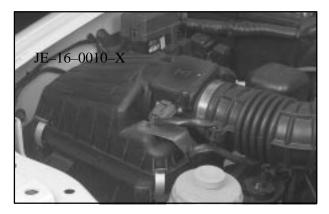
The engine air cleaner/filter is located on the passenger's side of the engine compartment toward the front of the vehicle.
