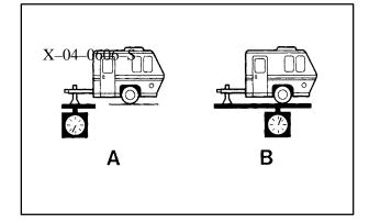
If you're using a weight-carrying hitch, the trailer tongue (A) should weigh 10 percent of the total loaded trailer weight (B). If you're using a weight-distributing hitch, the trailer tongue (A) should weigh 12 percent of the total loaded trailer weight (B).
