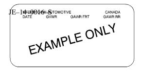
The other label is the Certification label, also found on the driver's door lock pillar. It tells you the gross weight capacity of your vehicle, called the Gross Vehicle Weight Rating (GVWR). The GVWR includes the weight of the vehicle, all occupants, fuel and cargo. Never exceed the GVWR for your vehicle, or the Gross Axle Weight Rating (GAWR) for either the front or rear axle.
