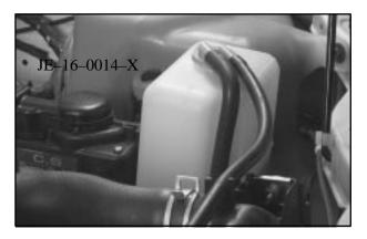
The vehicle must be on a level surface. When your engine is cold, the coolant level should be at LOW, or a little higher. When your engine is warm, the level should be up to FULL, or a little higher.
