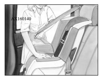
4. Pull the rest of the shoulder belt all the way out of the retractor to set the lock.
