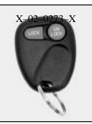
If your vehicle is equipped with this feature, you can lock and unlock your doors or unlock your rear door from about 3 feet (1 m) up to 30 feet (9 m) away using the remote keyless entry transmitter supplied with your vehicle.
