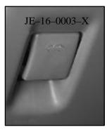
To open the hood, first pull the release handle located on the driver's side of the vehicle on the lower portion of the instrument panel.
