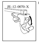
1. Turn the screw cover lock to the unlocked position and lower the cover.
