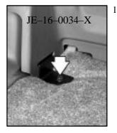
1. Remove the two attaching screws from each lower corner of the cargo area.
