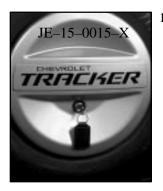
The spare tire is mounted on your tailgate. To remove the cover from the spare tire, insert your key into the wheel lock and pull the wheel lock off.
