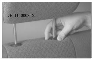
3. Remove the head restraint from the seatback by raising the head restraint fully. Push the release button and remove the head restraint from the seatback.
