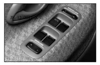
With power windows, switches on the driver's door control each window when the ignition is on. Push down the front of the switch to lower a window and lift the front of the switch to raise a window.
