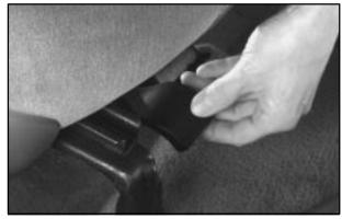
If your vehicle is equipped with easy entry seats, this is your front passenger seat adjuster. Pull up on the lever at the front of the passenger's seat up to unlock it. Slide the seat to a comfortable position. Then release the lever and try to move the seat with your body, to make sure the seat is locked into place.
