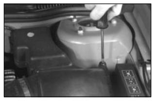
To check or replace the filter, remove the screws that hold the cover on and lift the cover. Be sure to reinstall the air cleaner filter and replace the cover tightly.
