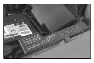
The engine compartment fuse block is located on the driver's side of the engine compartment. Lift off the cover to check the fuses.
