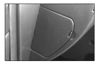
The fuse panel is located at the driver's side of the instrument panel. To open, push the tab on the access door to the left and pull the door forward. Make sure to insert the tabs when replacing the cover.
