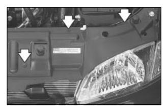
1. To rmove the six plastic fasteners from the shield use the flat-head screwdriver to pull up the center of the fastener. Be careful not to break the fasteners that hold the shield in place.
