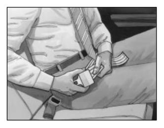
When you sit in the center seating position, you have a lap safety belt, which has no retractor. To make the belt longer, tilt the latch plate and pull it along the belt.
