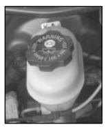
Your brake master cylinder reservoir is on the driver's side of the engine compartment. It is filled with DOT-3 brake fluid.
