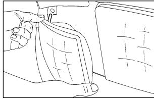
5. Align the outboard pin to the outboard tab in the bracket. Align the (2) inboard pins with the hole in the head lamp bracket.
