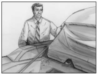
5. Pull the boot center cover from behind the rear seatback and place it over the inner sides of the boot side covers and the lowered top.
