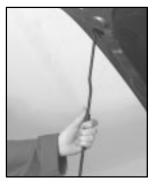
Release the hood prop from its retainer and put the hood prop into the slot in the hood marked "PROP ROD."
