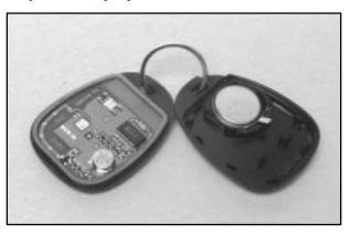
To replace the battery in the transmitter:
