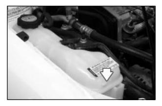
When the engine is cold, the coolant level should be at the FULL COLD mark. If it isn't, you may have a leak in the radiator hoses, heater hoses, radiator, water pump or somewhere else in the cooling system.
