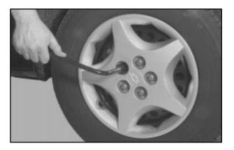
If your vehicle is equipped with wheel covers, use the wheel wrench to begin loosening the plastic wheel nut caps. Once you have loosened the plastic wheel nut caps with the wheel wrench you can finish loosening them with your fingers. Using the flat end of the wheel wrench, pry along the edge of the wheel cover until it comes off.
