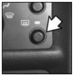
The rear window defogger uses a warming grid to remove fog from the rear window.
