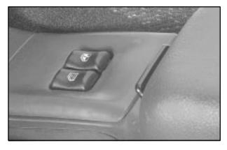
With power windows, switches on the center console control each of the windows when the ignition is on. In addition, on four-door models, each rear passenger door has a control switch for its own window.
