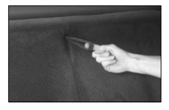
To open the fold-down rear seat, pull forward on the seat tab.
