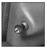
The power mirror control is located on the driver's door. Turn the control clockwise or counterclockwise to choose the mirror you want to adjust.
