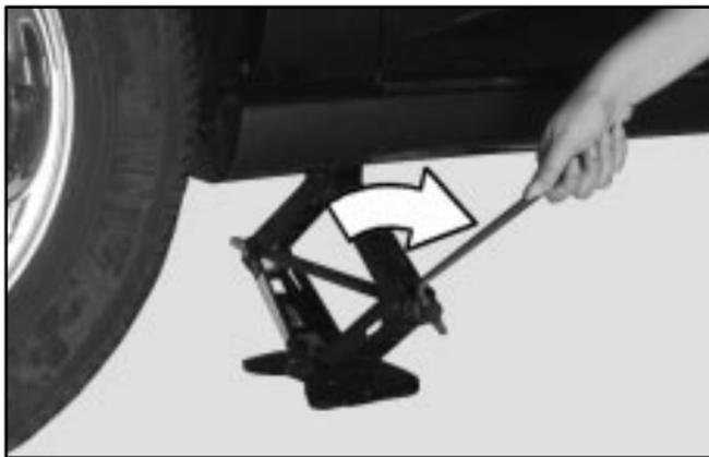
2. Raise the vehicle by turning the jack handle clockwise. Raise the vehicle far enough off the ground for the spare tire to fit under the vehicle. Remove all wheel nuts and take off the flat tire.
