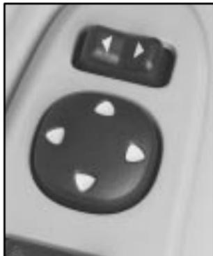
The power mirror switch is located near the driver's side window, on the armrest.
