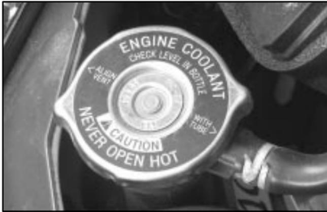
12. Then replace the pressure cap. At any time during this procedure if coolant begins to flow out of the filler neck, reinstall the pressure cap. Be sure the arrows on the pressure cap line up like this.
