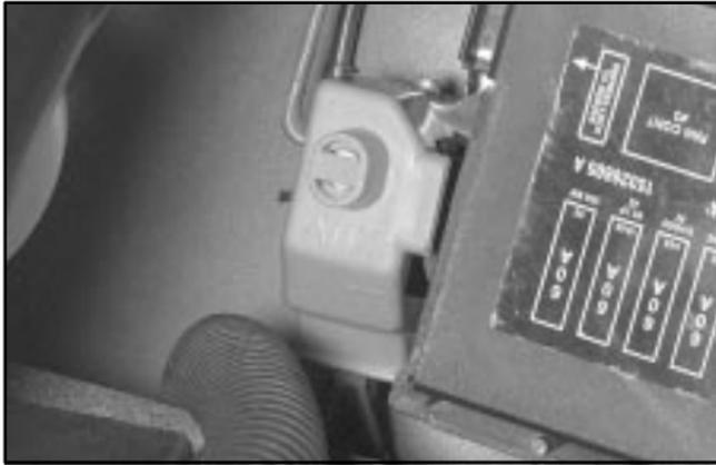
To uncover the remote positive (+) terminal, lift the plastic cap.
