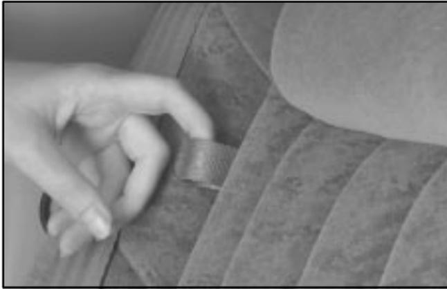
2. Pull forward on the seat tab to fold the seat cushion down. This will allow you direct access to the trunk.
