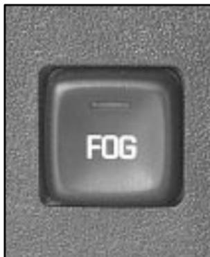
To turn the fog lamps on, press the fog lamps button located next to the exterior lamp control on the left side of the steering column. Your ignition must be in ON for the fog lamps to illuminate.
