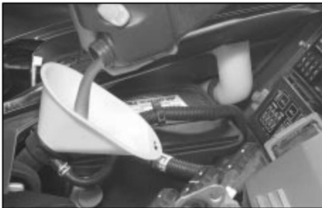
5. Fill the radiator with the proper DEX-COOL<sup>®</sup> coolant mixture, up to the base of the filler neck. See “Engine Coolant” in the Index for more information about the proper coolant mixture.
