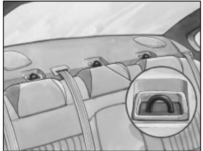
Anchor the top strap to one of these anchor points. Be sure to use an anchor point located on the same side of the vehicle as the seating position where the child restraint will be placed.
