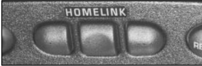
The HomeLink Transmitter allows you to consolidate the functions of up to three individual hand-held transmitters. It will operate garage doors and gates, or with the accessory package, other devices controlled by radio frequency such as home/office lighting systems and security systems.
