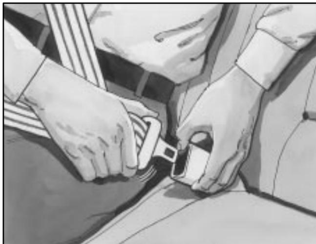
To unlatch the belt, just push the button on the buckle.
