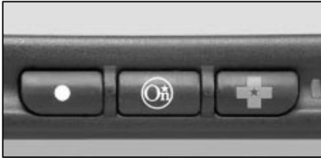
**OnStar Services Button:** Press this button once to contact an advisor who will be able to assist you with these services. If you are not quickly connected, the system will automatically reset and redial. This ensures connection to the center; there is no additional action required. Press the Call Answer/End button to cancel the automatic redial.
