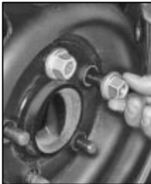
5. Reinstall the wheel nuts with the rounded end of the nuts toward the wheel. Tighten each nut by hand until the wheel is held against the hub.
