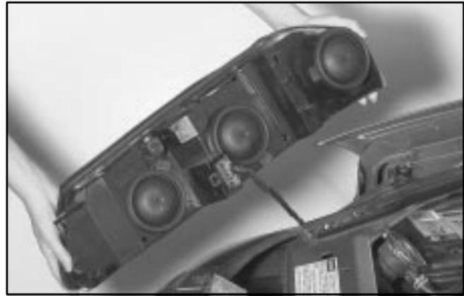
4. Gently pull the headlamp assembly away from the vehicle and remove the electrical connector.
