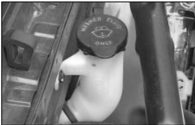
The windshield washer fluid reservoir is located on the passenger's side of the engine compartment near the diagonal cross brace. See "Engine Compartment Overview" in the Index for more information on location.
