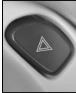
Press the switch located to the right of the instrument panel cluster to make the front and rear turn signal lamps flash on and off.
