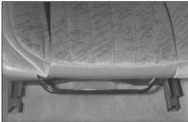
Lift the bar located under the front of the seat to unlock it. Slide the seat to where you want it and release the bar. Try to move the seat back and forth with your body to be sure the seat is locked in place.
