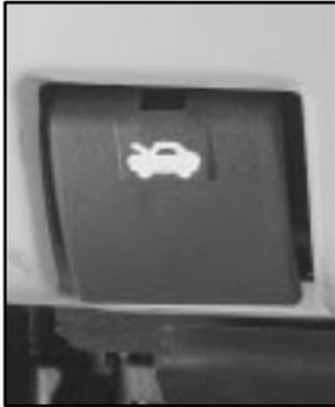
To open the hood, first pull the handle located inside the vehicle near the parking brake pedal.
