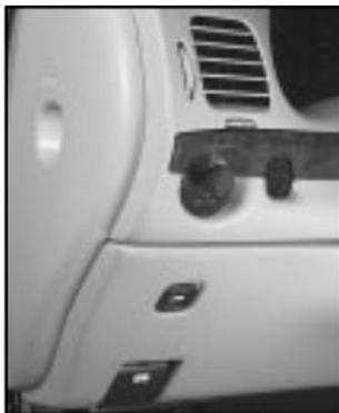
Some fuses are in a fuse block on the driver's side of the instrument panel. Pull off the cover labeled FUSES to expose the fuses.
