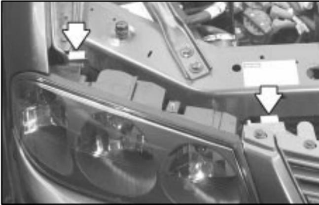
3. Remove the two headlamp fasteners by pulling up on them.
