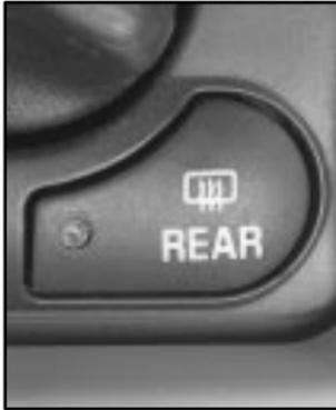
Press the button marked REAR to turn the defogger on. An indicator on the button will light.
