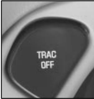
To turn the system on or off, press the TRAC OFF button on the left side of the instrument panel.
