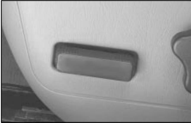
This switch is designed to control the movements of your seat cushion. It is located on the outboard side of the front seats toward the front of the seat cushion. To adjust the seat cushion, do any of the following:
