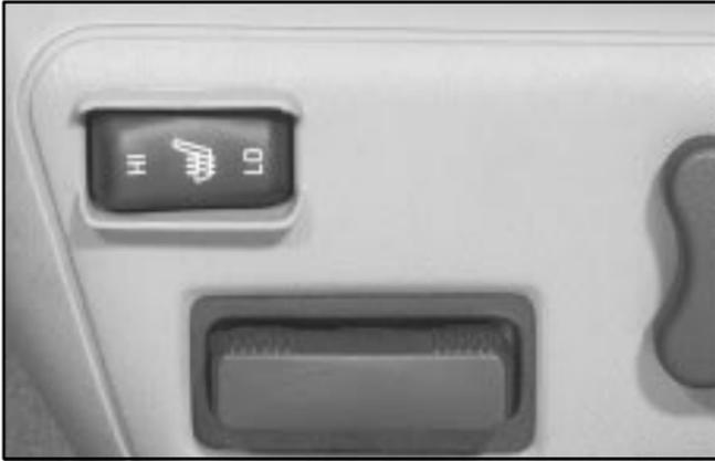
If your vehicle has heated seats, both the driver's and passenger's heated seat switches are on the outboard sides of the seats near the front.
