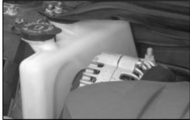
The coolant recovery tank is located between the power steering fluid reservoir and the underhood fuse block on the passenger's side of the engine compartment. See "Engine Compartment Overview" in the Index for more information on location.
