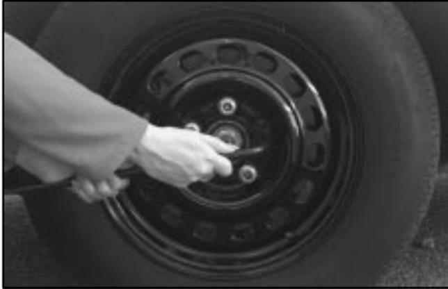
1. Using the wheel wrench, loosen all the wheel nuts. Don't remove them yet.
