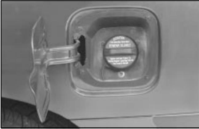
The tethered cap is behind a hinged door on the driver's side of your vehicle.
