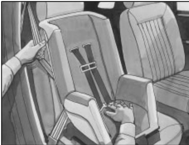
6. Push and pull the child restraint in different directions to be sure it is secure.
