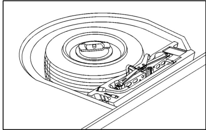
2. Lift and remove the cover. See “Compact Spare Tire” later in this section for more information about the compact spare tire.
