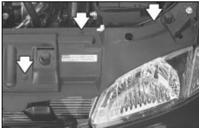
1. Remove the seven plastic fasteners from the shield. Use a screwdriver to pull up the center of the fastener. Be careful not to break the fasteners that hold the shield in place.
