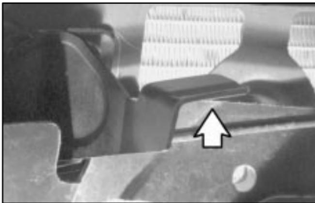
2. Then go to the front of the vehicle and lift up on the secondary hood release handle. The secondary hood release lever is located near the front center of the hood toward the driver's side.
