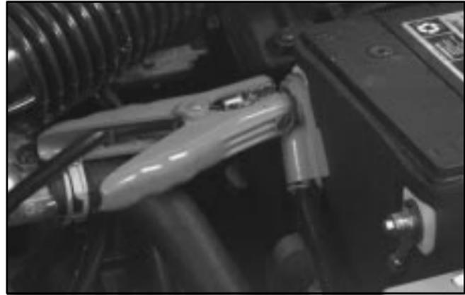
6. Remove the terminal cover and connect the red positive (+) cable to the positive (+) terminal of the dead battery. Use a remote positive (+) terminal if the vehicle has one.
