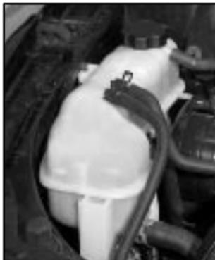
The surge tank is located on the passenger's side of the engine compartment. See "Engine Compartment Overview" in the Index for more information on location.
