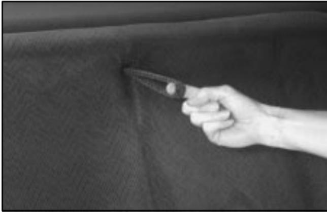
To fold down the rear seat, pull forward on the seat tab to unlatch the seatback.
