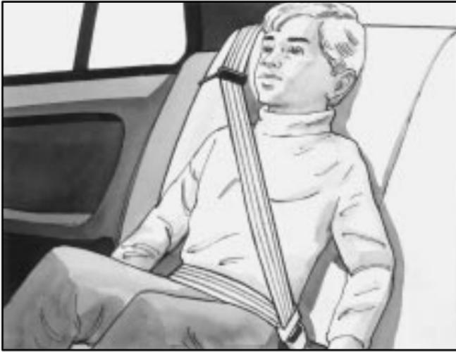
To remove and store the comfort guides, squeeze the belt edges together so that you can take them out of the guides. Pull the guide upward to expose its storage clip, and then slide the guide onto the clip. Turn the guide and clip inward and in between the seatback and the interior body, leaving only the loop of elastic cord exposed.
