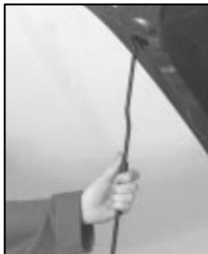
3. Lift the hood, release the hood prop from its retainer and put the hood prop into the slot in the hood marked "PROP ROD." Use the prop rod sleeve when handling the hood prop.
