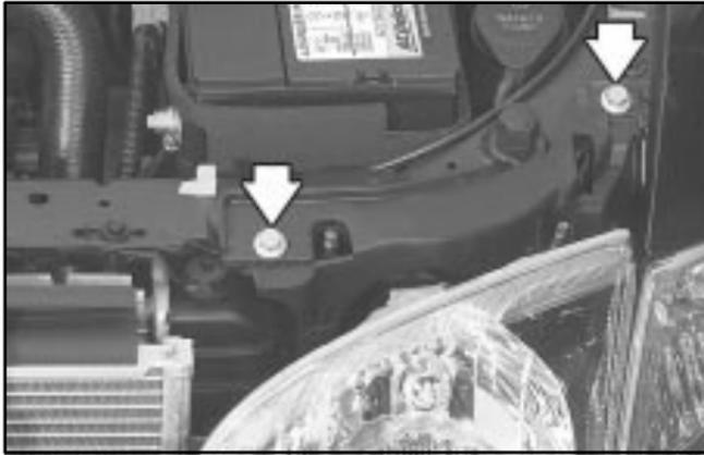
3. Remove the two bolts from the headlamp assembly. Pull the headlamp assembly up and toward the front of the vehicle to access the bulb assembly.
