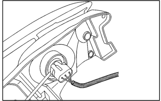
5. Disconnect the bulb base from the socket by lifting the plastic locking tab.
