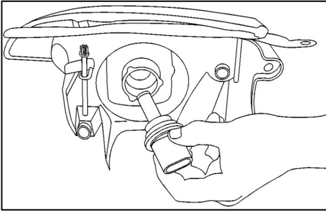
6. Remove the bulb by pulling the bulb straight out.
