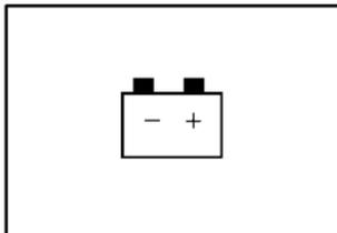
The charging system light will come on briefly when you turn on the ignition, and the engine is not running, as a check to show you it is working.
