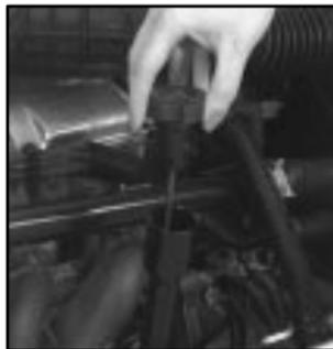
Check the oil here if you have a 2.2L L4 (LN2) engine. See “Engine Compartment Overview” in the Index for more information on location.
