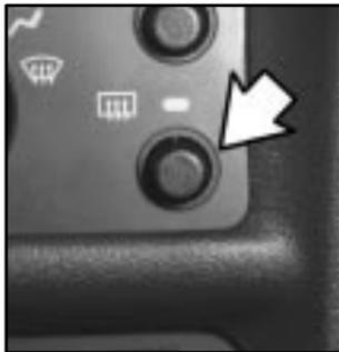
Press the button located under the air conditioning button to turn the defogger on. It will turn itself off after about 10 minutes.
