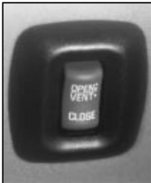
With the ignition on, press and release the rear of the switch and the glass panel will open to the vent position.
