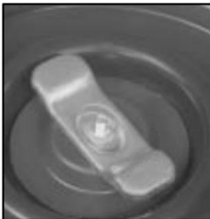
3. Turn the wing bolt counterclockwise and remove it. Then lift off the adapter and remove the compact spare tire.
