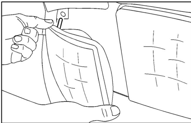
6. Push the front park and turn signal lamp straight in until you hear a snap. The snap feature is visible through the slot in the headlamp bracket.
