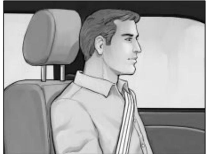
Slide the head restraint up or down so that the top of the restraint is closest to the top of your head. This position reduces the chance of a neck injury in a crash.
