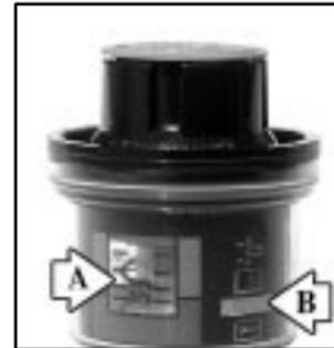
The service window (A) with the percentage scale shows the amount of engine air cleaner/filter life used. When both service window A and service window B turn orange, replace the engine air cleaner/filter.
