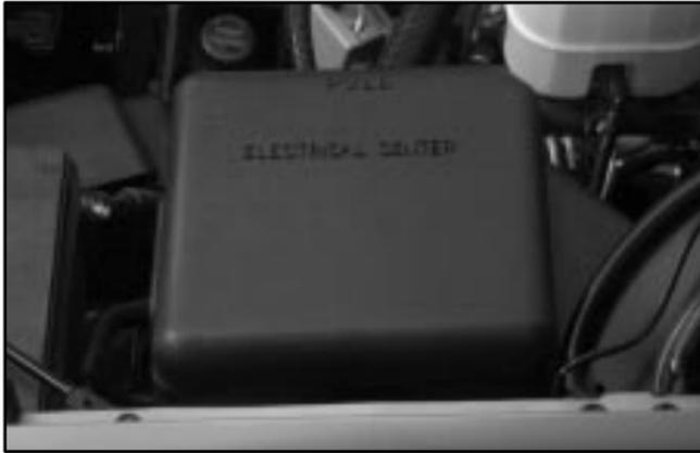
The underhood fuse block is in the engine compartment on the driver's side of the vehicle near the battery. Lift the cover for access to the fuse/relay block.
