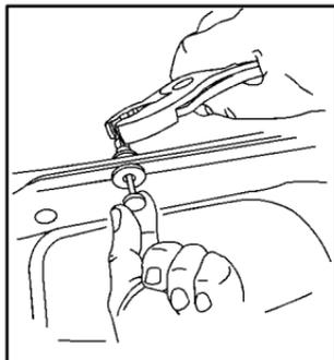
2. While continuing to pull downward on the push-pin, squeeze and turn the expandable end of the push-pin with a tool until it releases from the retainer.
