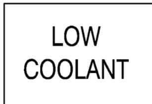
This message is displayed when the cooling system is low on coolant.
