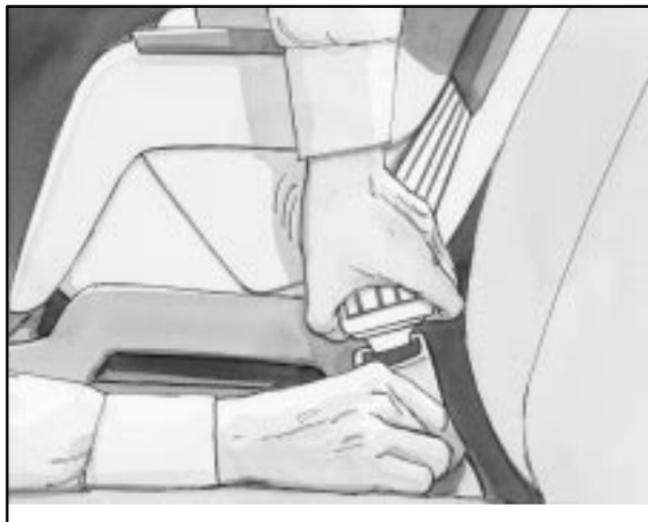
4. Buckle the belt. Make sure the release button is positioned so you would be able to unbuckle the safety belt quickly if you ever had to.
