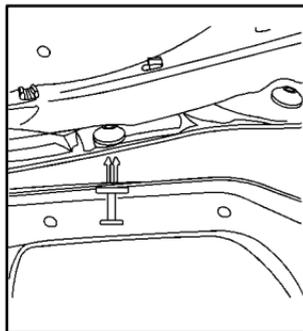
3. Pull the push-pins and lower air dam assembly away from the retainers until the lower air dam is free.
