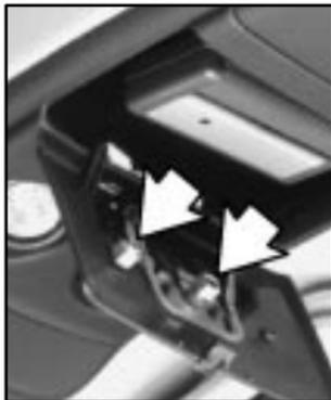
4. Add one peg at a time until, with the compartment door closed, the PUSH button on the compartment door will operate the garage door opener.
