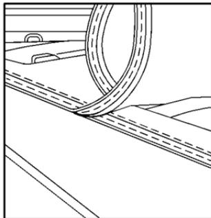
1. To remove, unsnap the cover. Roll up and stow using the buckle and the strap located at the front of the box.
