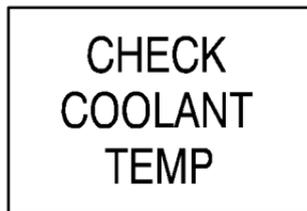
This message is displayed when the cooling system temperature gets hot.
