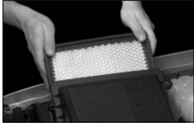
1. To remove the engine air cleaner/filter, loosen the screws on the housing cover. Lift the cover upward.
