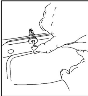
2. Push the flat end of the push-pin towards the retainer until it locks into place, making sure each is secure.
