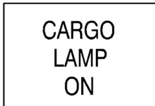
A message in the instrument panel cluster will come on and display CARGO LAMP ON when the cargo lamp is turned on and the ignition key is turned to RUN.
