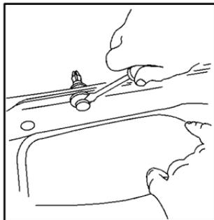
1. Insert a tool into the push-pin slot and pull downward until the push-pin snaps loose.
