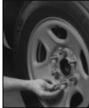
6. After mounting the spare, reinstall the wheel nuts with the rounded end of the nuts toward the wheel. Tighten each wheel nut by hand using the wheel wrench until the wheel is held against the hub.
