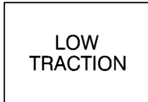
If you have the Traction Assist System, this light will come on when the system is limiting wheel spin. See "Traction Assist System" in the Index.
