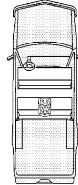
In order to use the system, you need either a forward-facing child restraint that has attaching points (B) at its base and a top tether anchor (C), or a rear-facing child restraint that has attaching points (B), as shown here.
