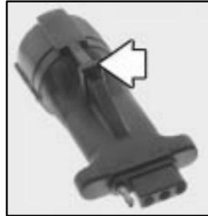
Connect the adapter with the tab (arrow) pointing towards the top. The cap on the wiring harness will lock onto the tab (arrow) and help hold the adapter in place.
