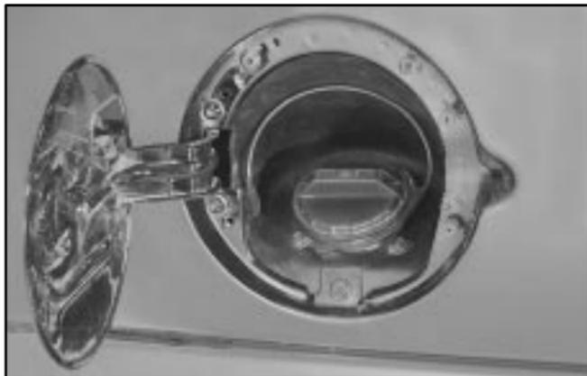
The fuel cap is located behind a hinged door on the driver's side of the vehicle. If your vehicle is a chassis cab, you will have a second fuel cap.
