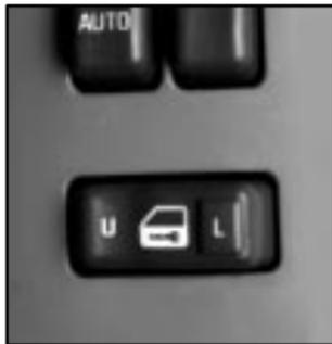
If your vehicle has this power door lock switch, press the raised side of the switch, marked L, on either front door to lock all the doors at once.
