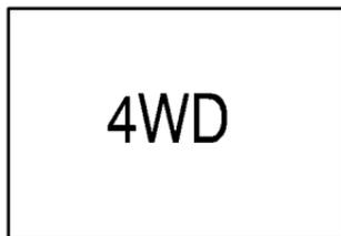
The 4WD indicator will light up when you shift a manual transfer case into four-wheel drive and the front axle engages.
