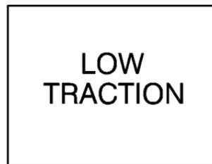
This light will come on when the TAS is limiting wheel spin. See "Low Traction Light" in the Index.
