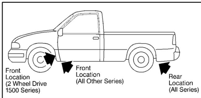
2. Position the jack under the vehicle. If the flat tire is on the front of the vehicle (Two-Wheel Drive 1500 Series vehicles), position the jack under the bracket attached to the vehicle's frame, behind the flat tire. If the flat tire is on the front of the vehicle (all other models), position the jack on the frame behind the flat tire.
