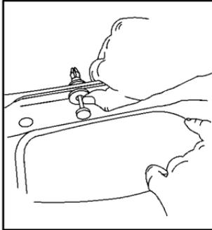
1. Line up each push-pin with its intended retainer and push the washer portion of the push-pin towards the retainer until it locks into place.
