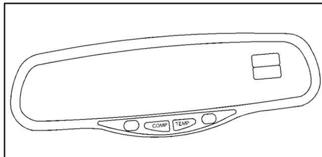
The mirror also includes a display in the upper right corner of the mirror face. The compass reading and the outside temperature will both appear in the display at the same time. The dual display can be turned on or off by briefly pressing either the TEMP or the COMP button.
