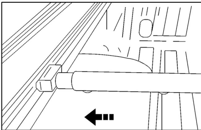
2. Remove the three bows by gently pushing them against the spring-loaded end. The three bows are labeled front/center/rear to remind you in which order to reinstall them.
