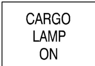
This message is displayed when the cargo lamp is turned on and the ignition key is turned to RUN.
