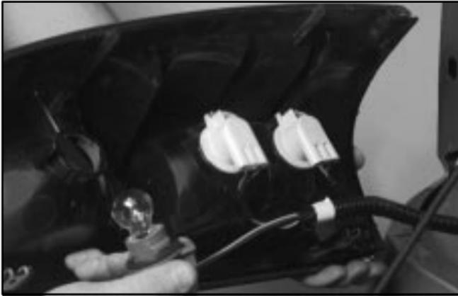
3. Press the release tab and turn the bulb socket counterclockwise to remove it from the taillamp housing.
