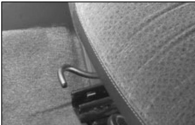
If your vehicle has this feature, you can raise or lower the front of the driver's or passenger's seat with this lever located at the inside edge of the seat. To raise or lower the front of the seat, move the lever up or down in a continuous motion until the cushion reaches the desired height.
