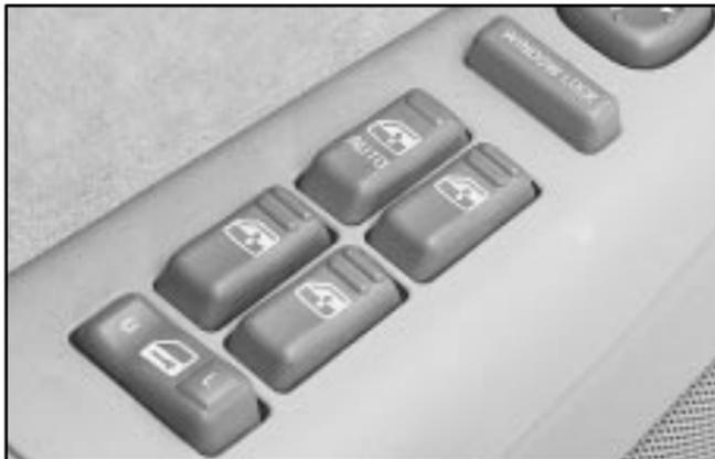
The driver's door has a switch for the passenger's windows as well. Your power windows will work when the ignition has been turned to ACCESSORY or RUN or when Retained Accessory Power (RAP) is active. See "Retained Accessory Power" in the Index.
