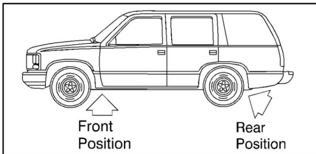
2. Position the jack under the vehicle. If the flat tire is on the front of the vehicle, position the jack on the frame behind the flat tire where the frame sections overlap.
