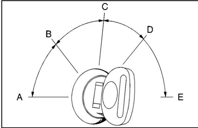
**A (ACCESSORY):** This position lets you use things like the radio, power windows and the windshield wipers when the engine is off. Push in the key and turn it toward you.
