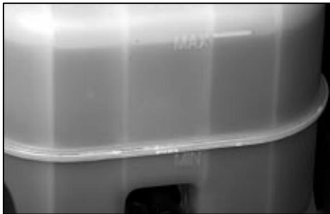
You can check the brake fluid without taking off the cap. Just look at the brake fluid reservoir. The fluid level should be above MIN. If it isn't, have your brake system checked to see if there is a leak.
