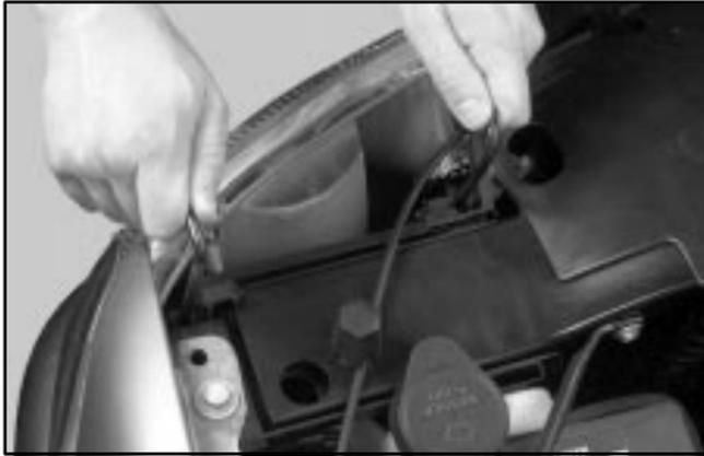
1. Remove the two pins on the top of the headlamp assembly. To remove the pins, turn the outer pin outward and pull it straight up. To remove the inner pin, turn it in and pull it straight up.
