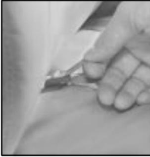
To fold, pull up on the strap loop at the rear of the seat cushion. Then, pull the seat cushion up and fold it forward.
