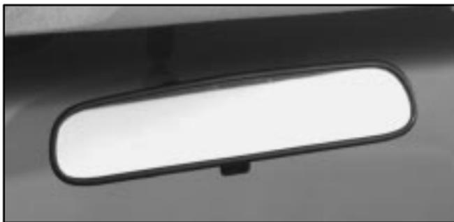
Pull the tab under the mirror toward you to reduce glare from headlamps behind you after dark. Push the tab away from you for normal daytime operation.
