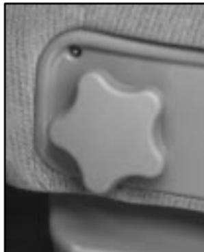
If your vehicle has a lumbar adjustment, the knob is located on the outboard side of the seat cushion.
