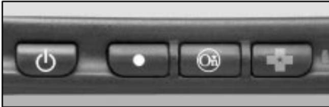
**OnStar Services Button:** Press this button once to contact an advisor who will be able to assist you with these services. If you are not quickly connected, the system will automatically reset and redial. This ensures connection to the center; there is no additional action required. Press the Communication button to cancel the automatic redial.
