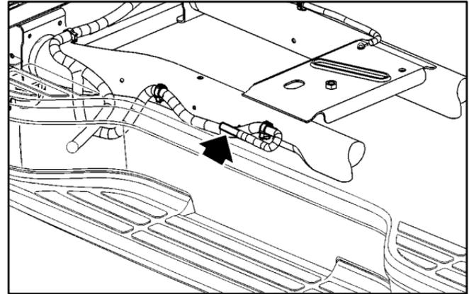
The trailer wiring harness, with a seven-pin connector, is located at the rear of the vehicle and is tied to the vehicle's frame. The harness connector can be plugged into a seven-pin universal heavy-duty trailer connector available through your dealer.
