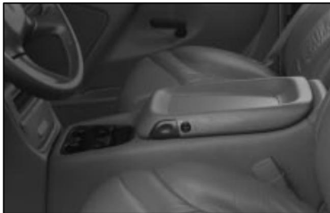
To open it, insert the console key into the lock and unlock the console. Press the button and swing the console lid open.
