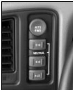
The transfer case buttons are located to the left of the instrument panel cluster.
