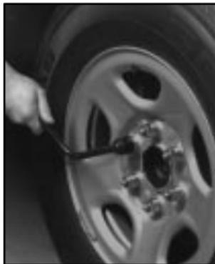
1. Use the wheel wrench to loosen all the wheel nuts. Turn the wheel wrench counterclockwise to loosen the wheel nuts. Don't remove the wheel nuts yet.
