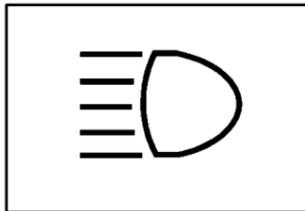
When the high beams are on, this light on the instrument panel cluster also will be on.
