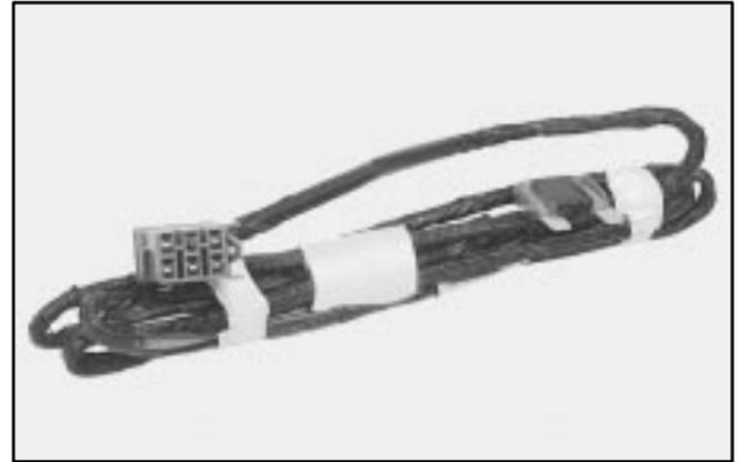
This harness is included with the heavy-duty trailer wiring package. The harness is for an electric trailer brake controller and includes a trailer battery feed fuse. This harness and fuse should be installed by your dealer or a qualified service center.
