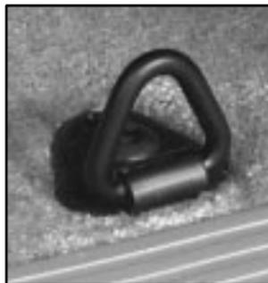
There are cargo tie downs in the rear cargo area that allow you to strap cargo in and keep it from moving inside the vehicle.
