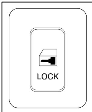
On the passenger side of the rear cargo door or liftgate opening trim there is a power lock switch which can be used to lock or unlock all of the doors.
