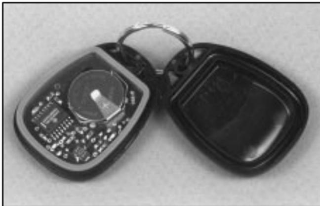
1. Insert a dime, or similar object, in the slot between the covers of the transmitter housing near the key ring hole. Remove the bottom by twisting the dime.
