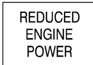
This message is displayed when the cooling system temperature gets too hot and the engine further enters the engine coolant protection mode.
