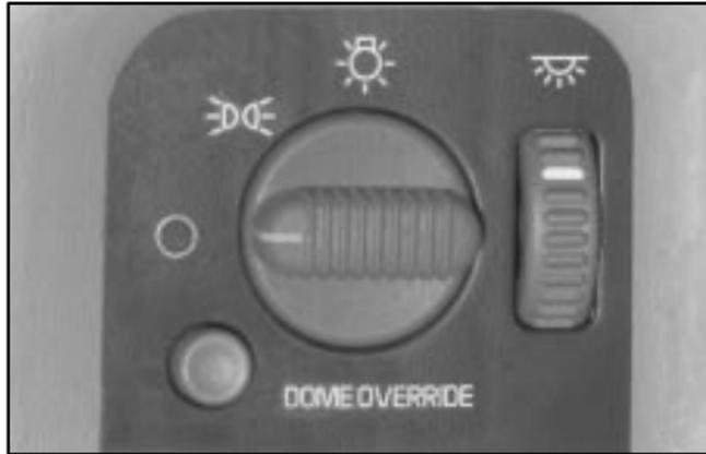
The control on the driver's side of your instrument panel operates the exterior lamps.
