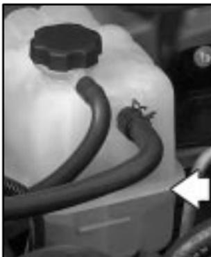
The coolant level should be at or above the **FILL COLD** mark. If it isn't, you may have a leak at the pressure cap or in the radiator hoses, heater hoses, radiator, water pump or somewhere else in the cooling system.
