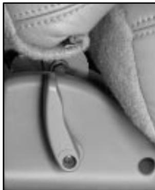
2. Push the seatback release lever rearward and pull the seatback forward. Then fold it until it is flat.
