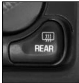
To turn on the rear window defogger, press this button next to the fan knob.
