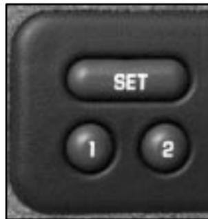
If your vehicle has this feature, the buttons used to program and recall the driver's seat and recliner position are located on the driver's door trim panel.
