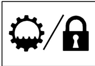
The red transmission dipstick handle with the TRANS/LOCK text or graphic is located at the rear of the engine compartment, on the passenger's side.
