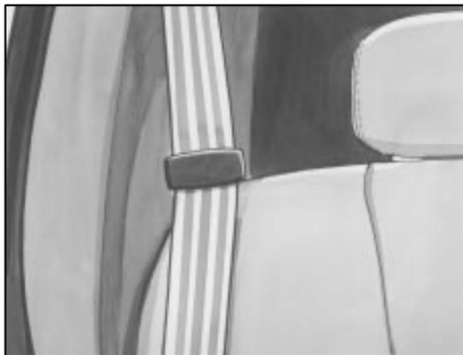
3. Be sure that the belt is not twisted and it lies flat. The guide must be on top of the belt.
