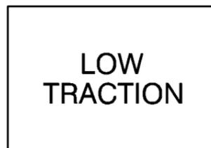
This light will come on when the TAS is limiting wheel spin. See "Low Traction Light" in the Index.
