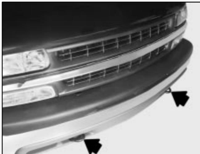
Your vehicle may be equipped with recovery hooks. The hooks are provided at the front of your vehicle. You may need to use them if you're stuck off-road and need to be pulled to some place where you can continue driving.
