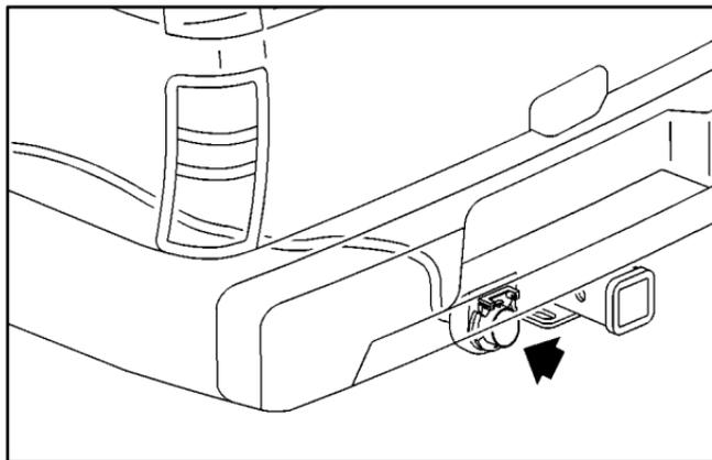
Your vehicle is equipped with the seven-wire trailer towing harness. This harness with a seven-pin universal heavy-duty trailer connector that is attached to a bracket on the hitch platform.
