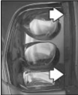
2. Remove the two screws from the lamp assembly.
