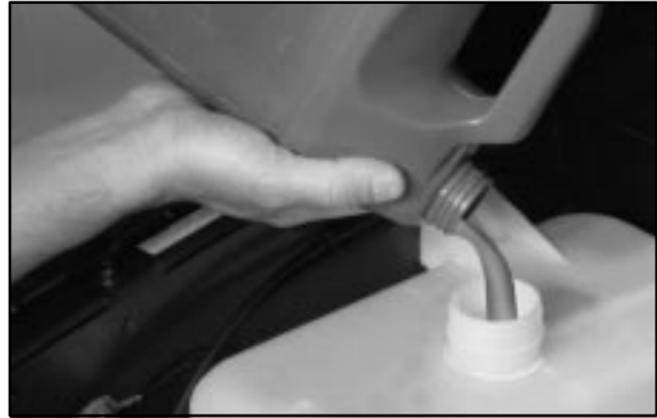
4. Then fill the coolant recovery tank to the FULL COLD mark.
