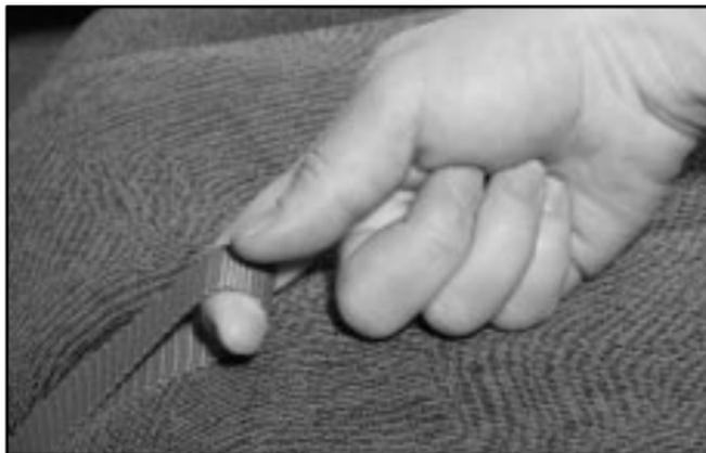
Pull up on the tab located where the seat cushion meets the seatback to fold the seat cushion up and out of the way. This will allow the seatback to fold flat and increase the cargo area.
