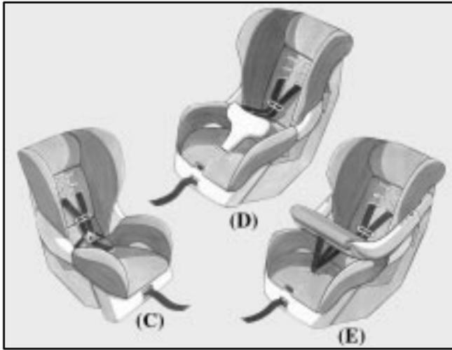
A forward-facing child seat (C-E) provides restraint for the child's body with the harness and also sometimes with surfaces such as T-shaped or shelf-like shields.
