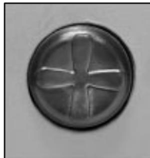
If your vehicle has this feature, the driver's and passenger's seatback lumbar support can be adjusted four ways by moving a single control located on the outboard side of the seat cushions.
