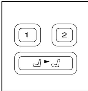
If your vehicle has this feature the controls are located on the driver's door, and are used to program and recall memory settings for the driver's seating and outside mirror positions.
