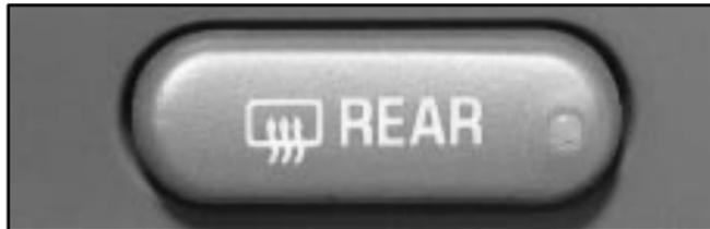
The lines you see on the rear window warm the glass. Press the button to start warming your window. A light will glow in the button while the defogger is working.
