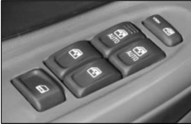
The controls for the power windows are located on the armrest on each of the side doors. With power windows, the switches operate the windows when the ignition is in RUN, ACCESSORY or when Retained Accessory Power (RAP) is active. (See “Retained Accessory Power” in the Index.) The driver’s door has a switch for each of the passenger’s windows as well.
