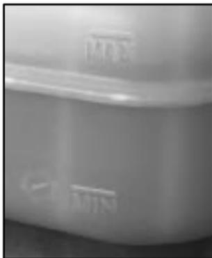
You can check the brake fluid without taking off the cap. Just look at the brake fluid reservoir. The fluid level should be above MIN. If it isn't, have your brake system checked to see if there is a leak.
