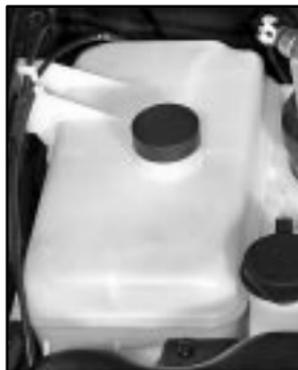
When the engine is cold, the coolant level should be at least up to the **FULL COLD** mark. If it isn't, you may have a leak in the radiator hoses, heater hoses, radiator, water pump or somewhere else in the cooling system.
