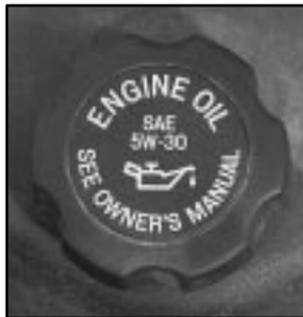
The engine oil fill cap is located in the engine compartment toward the passenger's side of the vehicle. See "Engine Compartment Overview" in the Index for more information on location.
