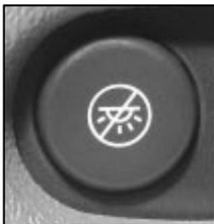
You can use the dome override button, located below the exterior lamps knob, to set the dome lamps to come on automatically when a door is opened, or to remain off.
