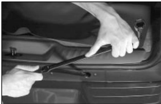
1. To remove the underbody-mounted spare, insert the socket end of the extension, on an angle, into the hole in the rear bumper. Be sure the socket end of the extension connects into the hoist shaft.
