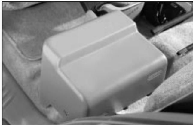
The rear underseat fuse block is located under the rear seat on the driver's side of the vehicle.
