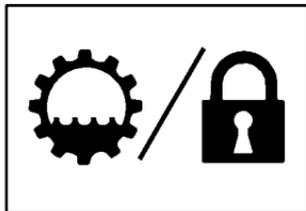
Locate the handle with the transmission and lock symbols for the automatic transmission dipstick in the engine compartment on the passenger's side of the vehicle.
