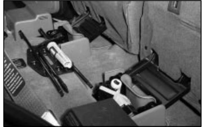
The jacking equipment you will need is stored under the rear seat of the vehicle. See “Rear Seats” in the Index for more information on accessing the jacking equipment under the rear seat.
