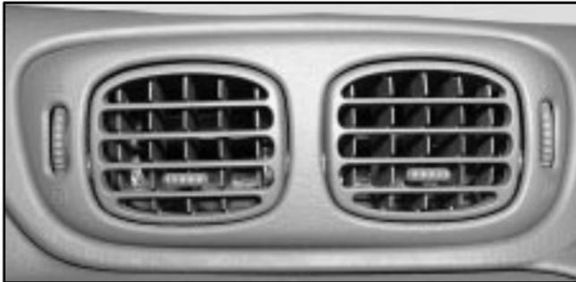
Your vehicle has air outlets that allow you to adjust the direction and amount of airflow inside the vehicle. Move the louvers up or down and move the control in the center of each outlet side-to-side to direct the air from the outlet. Use the thumbwheel next to or underneath the outlet to close the louvers. For the most efficient airflow and temperature control, keep the outlet in the fully opened position.
