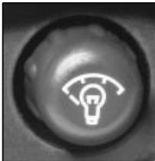
Press the knob located next to the exterior lamps knob to extend and turn it to make your instrument panel lights brighter. Turn the knob all the way up to turn on the interior lamps. Press the knob back into its stored position.
