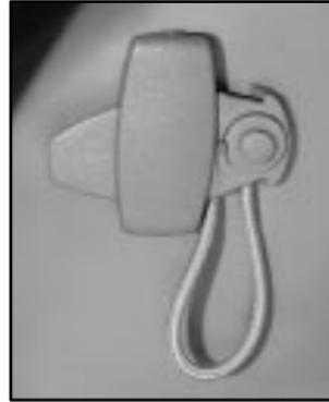
1. Slide the guide off of its storage clip located between the interior body and the seatback.
