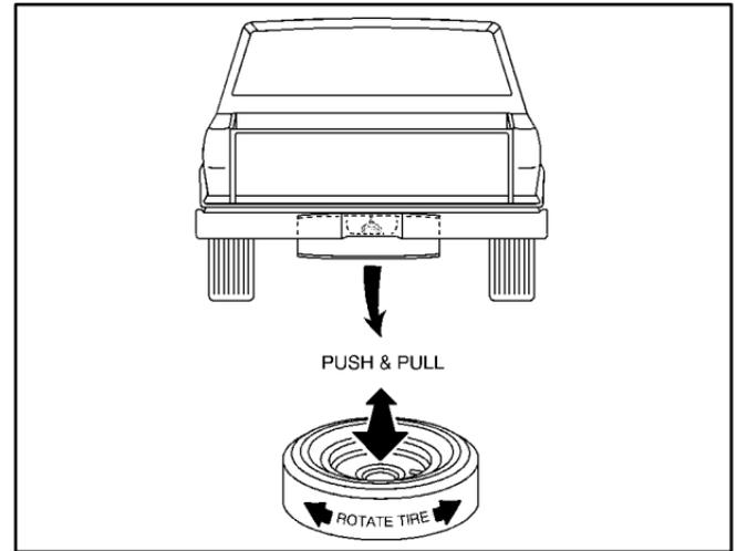
5. Make sure the tire is stored securely. Push, pull, and then try to rotate or turn the tire. If the tire moves, use the wheel wrench to tighten the cable.
