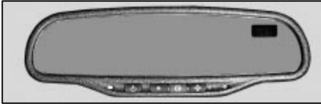
Your vehicle may have an automatic-dimming rearview mirror with a compass, temperature display and the OnStar system.
