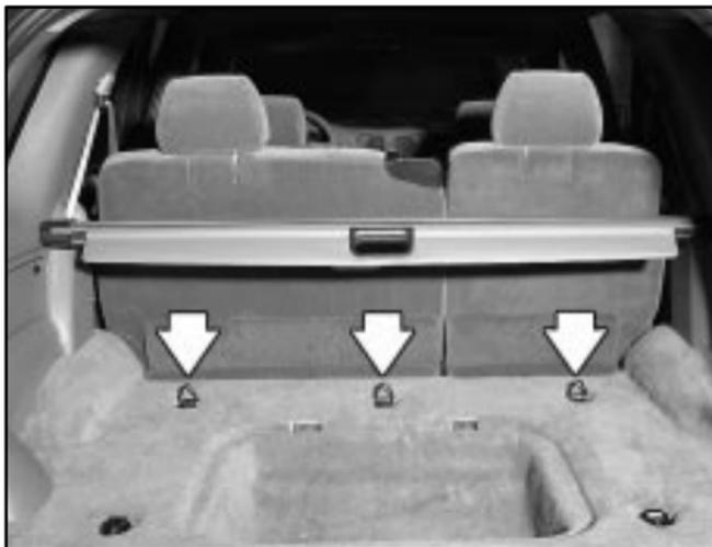
Anchor brackets for the rear seat positions are located on the floor in the cargo area of your vehicle. Do not use the rear tie-down brackets near the liftgate for top strap tethers.
