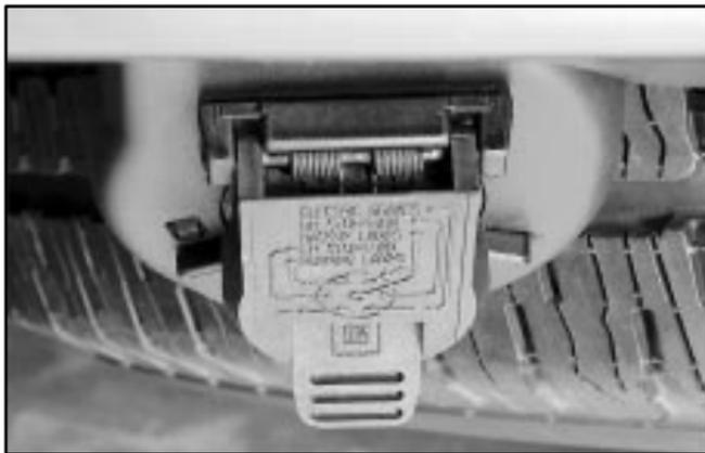
Your vehicle is equipped with the seven-wire trailer towing harness. This harness has a seven-pin universal heavy-duty trailer connector that is attached to a bracket on the hitch platform. The seven-wire harness contains the following trailer circuits:
