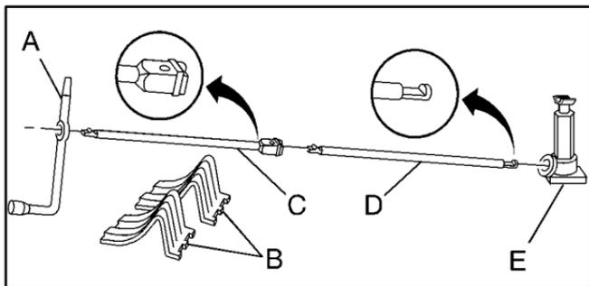
The tools you'll be using include the wheel wrench (A), tire blocks (B), extension (socket end) (C), handle (jack end) (D), and jack (E).
