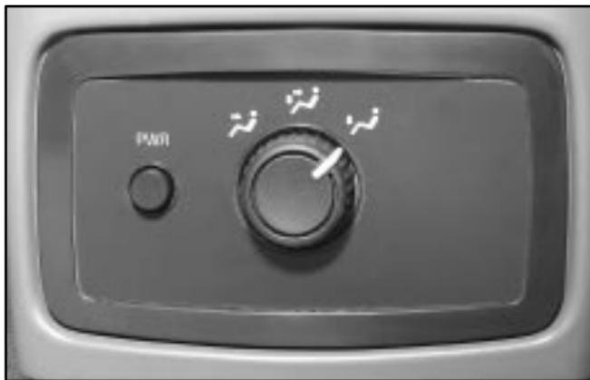
The temperature of the air coming through the rear outlets is determined by the front passenger's temperature setting. Press the PWR button to turn the rear comfort controls on and off. Use the mode knob to change the direction of airflow (upper, bi-level or floor) to the rear seat area.
