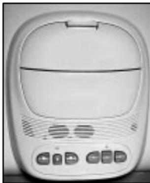
The overhead console includes sunglasses storage, a HomeLink<sup>®</sup> transmitter and a travel note recorder (if equipped).
