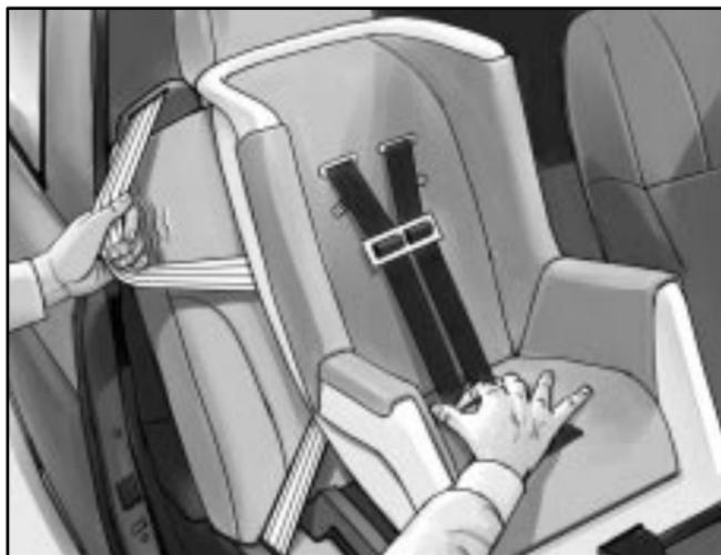
5. Pull the rest of the shoulder belt all the way out of the retractor to set the lock.
