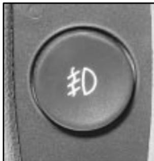
The fog lamp button is located on the instrument panel to the right of the exterior lamps knob. Press the button to turn the fog lamps on. Press the button again to turn them off. A light will glow near the button when the fog lamps are on.
