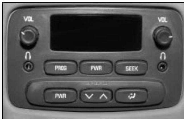
If your vehicle has the rear seat audio system the lower buttons are used to adjust the rear seat comfort controls. The temperature of the air coming through the rear outlets is determined by the front passenger's temperature setting. The button with the up and down arrows on it regulates the fan speed. The mode button can be used to change the direction of airflow (upper, bi-level or floor) to the rear seat area. To turn the rear comfort controls off, press the lower PWR button.
