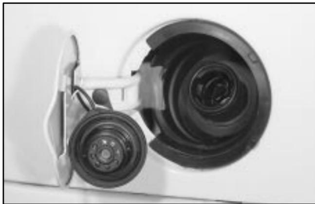
While refueling, hang the fuel cap by the tether using the hook located on the inside of the filler door.
