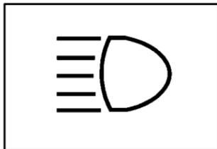
When the high beams are on, this indicator light on the instrument panel cluster will also be on.
