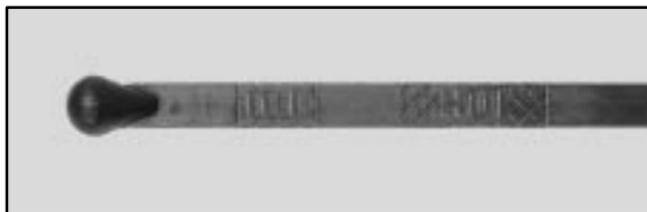
3. If the fluid level is in the acceptable range, push the dipstick back in all the way; then flip the handle down to lock the dipstick in place.
