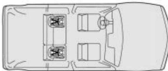
In order to use the system, you need either a forward-facing child restraint that has attaching points (B) at its base and a top tether anchor (C), or a rear-facing child restraint that has attaching points (B), as shown here.
