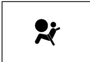
There is an air bag readiness light on the instrument panel, which shows the air bag symbol.
