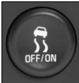
To turn the system on or off press the TAS on/off button located near the shift lever. If you used the button to turn the system off, the TRAC OFF light on the button will come on and stay on.
