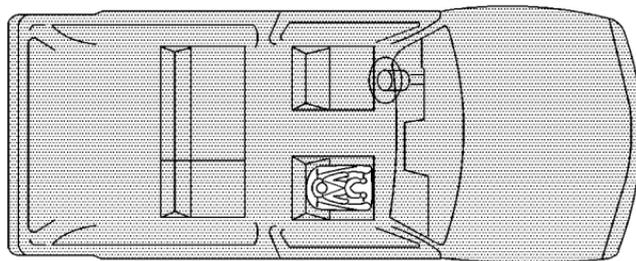
Your vehicle has a right front passenger air bag. *Never* put a rear-facing child restraint in this seat. Here's why:
