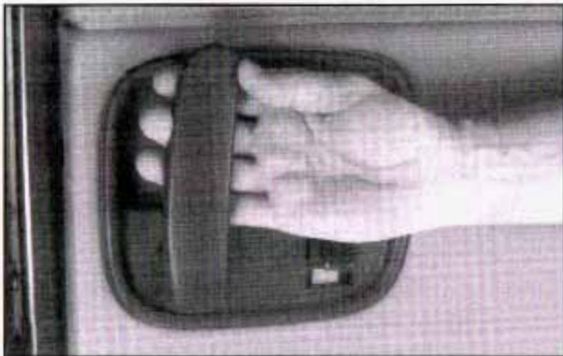
To open the sliding door from inside, turn the handle upward and toward the rear of the vehicle. Then, slide the door toward the rear of the vehicle to open it.
