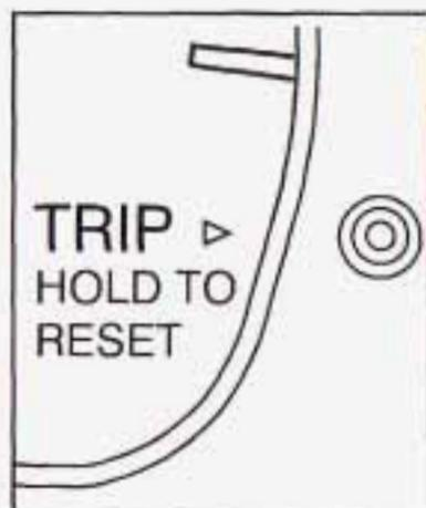
The trip odometer can tell you how far your vehicle has been driven since you last set the trip odometer to zero.
