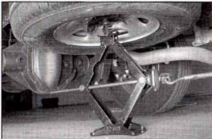
6. Place the jack under the vehicle, ahead of the rear bumper. Position the center lift point of the jack under the center of the spare tire and turn the handle clockwise to raise the jack until it lifts the secondary latch spring.
