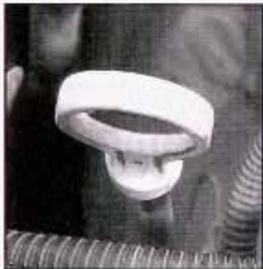
The engine oil dipstick has a yellow handle and is located near the center of the engine compartment. See *Engine Compartment Overview* on page 5-12 for more information on location.
