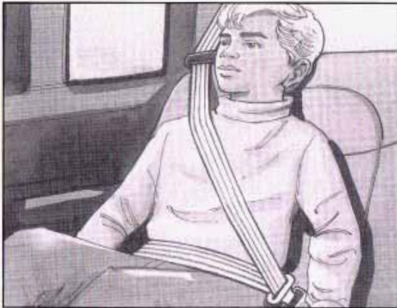
4. Buckle, position and release the safety belt as described in *Rear Seat Passengers on page 1-27*. Make sure that the shoulder belt crosses the shoulder.
