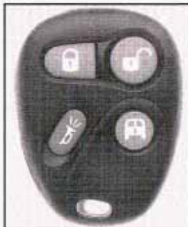
**🔒 (Lock):** Pressing this button once will lock all of the doors. The parking lamps will flash and the interior lamps will turn on briefly. Press LOCK again within five seconds and the parking lamps will flash and the horn will chirp briefly.
