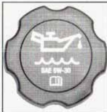
The engine oil filler cap is located between the coolant recovery tank and the engine air cleaner/filter. See *Engine Compartment Overview on page 5-12* for more information on location.
