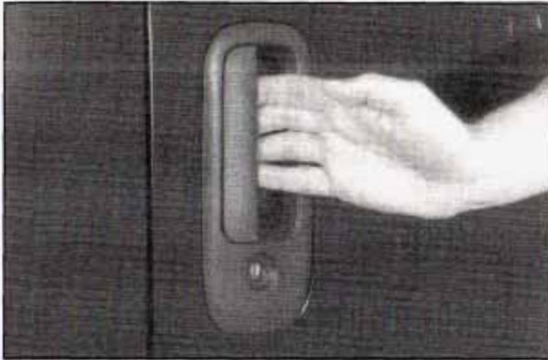
To open the front portion of a 60/40 door from the outside, pull out on the handle and pull it toward you.
