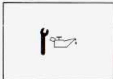
This light is displayed when the engine oil needs to be changed.
