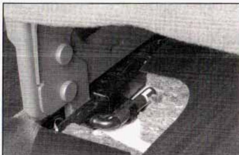
5. Push the pin with the black handle marked "L" down until it is in the retaining clip.
