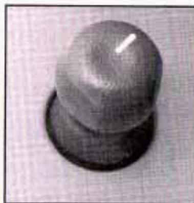
Select the mirror you want to move by turning the knob clockwise to adjust the passenger's side mirror and counterclockwise to adjust the driver's side mirror. The center position is neutral.
