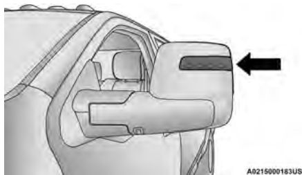
Forward Utility Light
