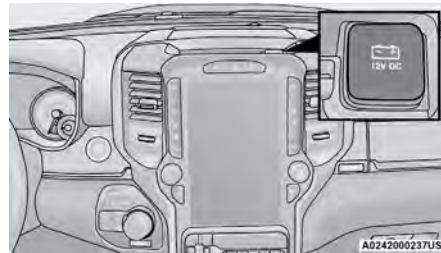
Power Outlet — Top Of Center Stack
