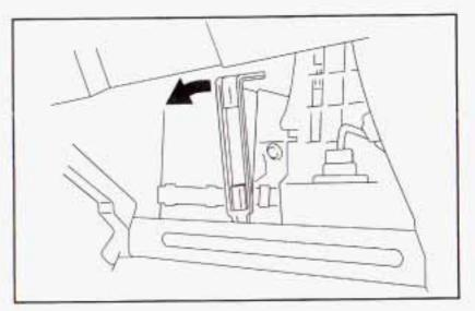
Lift the top tab on the cover to remove the filter cover.
