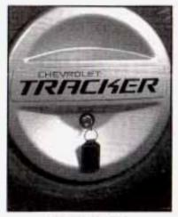
To remove the hard cover from the spare tire, insert your key into the wheel lock and pull the wheel lock off.
