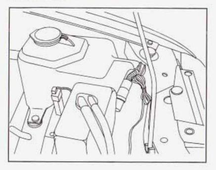
If your vehicle has this feature, in very cold weather, 0°F (18°C) or colder, the engine coolant heater can help. You'll get easier starting and better fuel economy during engine warm-up. Usually, the coolant heater should be plugged in a minimum of four hours prior to starting your vehicle. At temperatures above 32°F (0°C), use of the coolant heater is not required.
