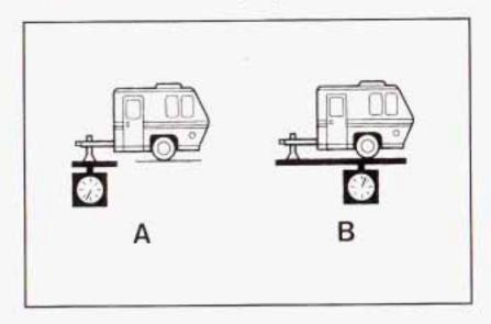
If you're using a weight-carrying or a weight-distributing hitch, the trailer tongue weight (A) should be 10 percent to 15 percent of the total loaded trailer weight (B). Do not exceed the maximum allowable tongue weight for your vehicle. After you've loaded your trailer, weigh the trailer and then the tongue, separately, to see if the weights are proper. If they aren't, you may be able to get them right simply by moving some items around in the trailer.
