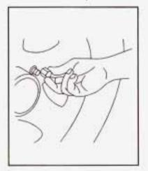
Reinstall the wheel nuts with the cone-shaped end of the nuts toward the wheel. Tighten each nut by hand until the wheel is held against the hub.
