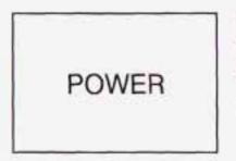
This light comes on when the power mode selector switch, if equipped, is turned to P (power) with the ignition switch in the ON position.
