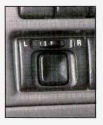
If your vehicle has power mirrors, the switch is located on the lower left side of the instrument panel.
