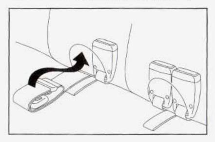
Fold the safety belt buckles and center safety belt (if equipped) into the pocket of the rear seatback.
