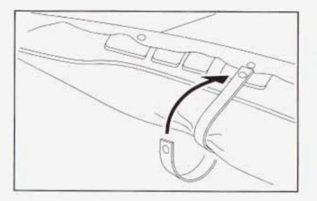
Wrap the holding strap around the canvas top and snap it to the front top bow retaining strap.
