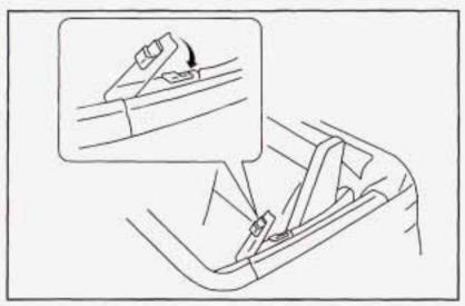
Engage the latches by pushing down on the support arms at the hinges.
