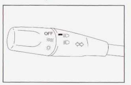
The lever on the left side of the steering column operates the exterior lamps.
