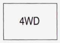
If you have four-wheel drive, this light comes on when the ignition switch is on and the transfer case lever is in one of the four-wheel drive positions.
