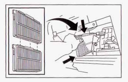
Install the lower filter by dropping it down into the slot.
