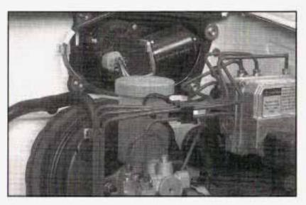
Your brake master cylinder reservoir is filled with DOT-3 brake fluid. See Engine Compartment Overview on page 5-12 for the location of the reservoir.
