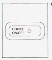
Press the CRUISE ON/OFF button on the instrument panel to turn the system on. The indicator light in the button will come on. Wait at least one second after turning the system on before setting a speed.
