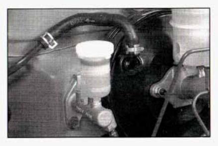
Refer to the Maintenance Schedule to determine how often you should check the fluid level in your clutch master cylinder reservoir and for the proper fluid. See *Part B: Owner Checks and Services on page 6-24* and *Part D: Recommended Fluids and Lubricants on page 6-30.*
