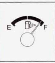
Your fuel gage shows about how much fuel is in your tank. When the gage first indicates E (empty), you still have about one or two gallons (4 to 8 L) of fuel left in your tank, but you need to get more right away.
