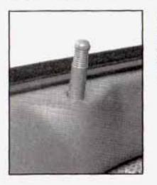
To lock the door from the inside, push down on the manual lock rod located on the door. To unlock it, pull up on the manual lock rod.
