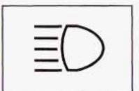
When the high beams are on, a light on the instrument panel cluster also will be on. It will go off when you switch to low beam.
