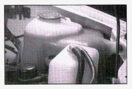
Open the cap with the washer symbol on it. Add washer fluid until the tank is full.
