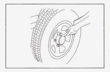
Using the wheel wrench, loosen all the wheel nuts but don't remove them yet.
