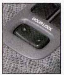
To lock all the doors and the tailgate, press the right side of the switch. To unlock the doors and the tailgate, press the left side of the switch.
