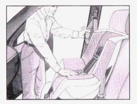
To tighten the belt, feed the shoulder belt back into the retractor while you push down on the child restraint. You may find it helpful to use your knee to push down on the child restraint as you tighten the belt. Push and pull the child restraint in different directions to be sure it is secure.
