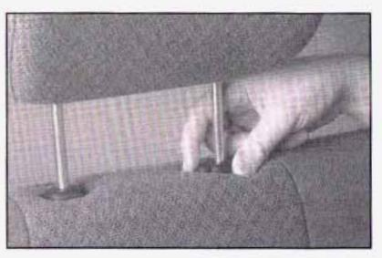
Remove the head restraint from the seatback by raising the head restraint fully. Press the release button and remove the head restraint from the seatback.
