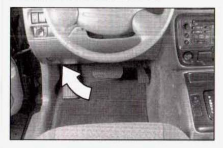
This fuse block is located under the driver's side of the instrument panel. The fuses here protect each separate circuit including headlamps. There are spare fuses inside the fuse box. If you have electrical failure, check here first.
