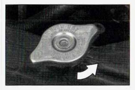
You can remove the radiator pressure cap when the cooling system, including the radiator pressure cap and upper radiator hose, is no longer hot. Turn the pressure cap slowly counterclockwise until it first stops. (Don't press down while turning the pressure cap.)
