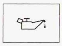
If the engine oil pressure light appears on the instrument cluster, it means you need to check your engine oil level right away.
