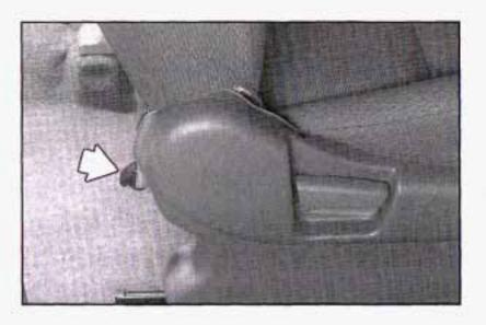
To get out of the rear seat area, push the release pedal on the rear of the front passenger's side front seat. Then tilt the seatback forward, and slide the whole seat forward.
