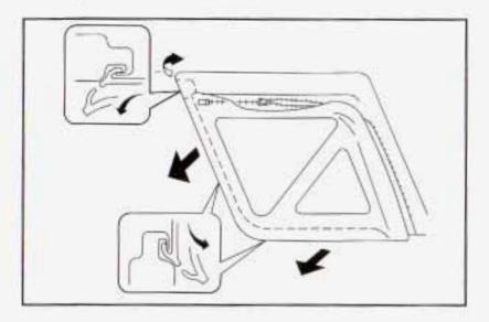
Unfasten the plastic clip, which is part of the canvas top, at the top front corner of each side window. Then unzip the zipper the rest of the way and remove the side window. To install the side window:
