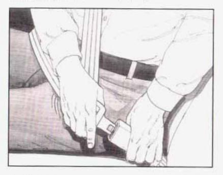
2. Push the latch plate into the buckle until it clicks. Pull up on the latch plate to make sure it is secure. When the shoulder belt is pulled out all the way, it will lock. If it does, let it go back all the way and start again. If the belt is not long enough, see Safety Belt Extender on page 1-29. Make sure the release button on the buckle is positioned so you would be able to unbuckle the safety belt guickly if you ever had to.
