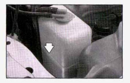
The coolant level should be at or above FULL. If it isn't, you may have a leak at the pressure cap or in the radiator hoses, heater hoses, radiator, water pump or somewhere else in the cooling system.
