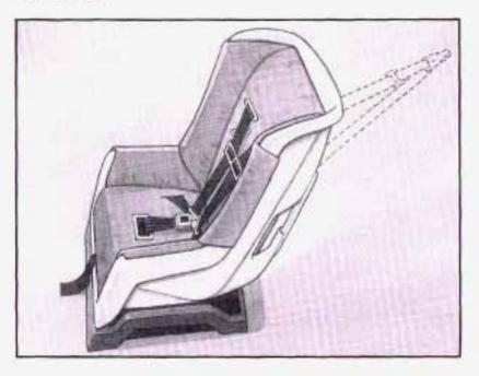
Anchor the top strap to one of the following anchor points. Be sure to use an anchor point located on the same side of the vehicle as the seating position where the child restraint will be placed.
