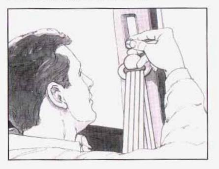
To move it down, pull the knob and move the height adjuster to the desired position. You can move the adjuster up just by pulling out the knob and sliding the adjuster up. After you move the adjuster to where you want it, try to move it down without pulling out the knob to make sure it has locked into position.
