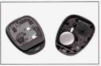
To replace the battery in the transmitter do the following:
