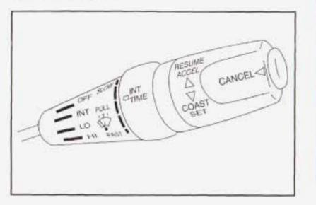
If your vehicle has cruise control, you can maintain a speed of about 25 mph (40 km/h) or more without keeping your foot on the accelerator. This can really help on long trips. Cruise control will not set at speeds below about 25 mph (40 km/h).
