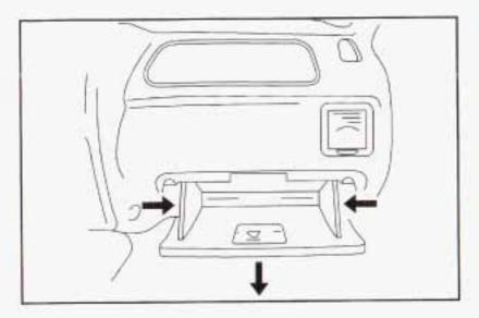
Lower the glove box door, then push in the sides of the glove box to completely lower the door to allow access to the slot where the air filters will be installed.
