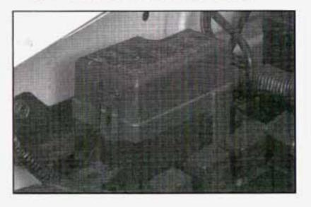
The engine compartment fuse block is located in the engine compartment on the passenger's side of the vehicle and protects all electrical loads. See Engine Compartment Overview on page 5-12 for more information on location.
