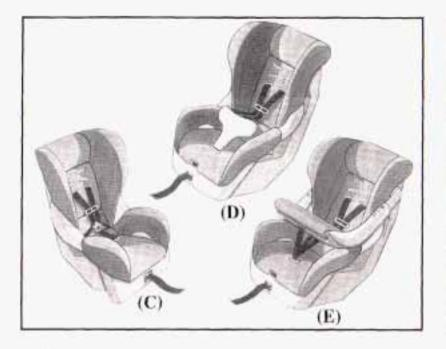
A forward-facing child seat (C-E) provides restraint for the child's body with the harness and also sometimes with surfaces such as T-shaped or shelf-like shields. A booster seat (F-G) is a child restraint designed to improve the fit of the vehicle's safety belt system. Some booster seats have a shoulder belt positioner, and some high-back booster seats have a five-point harness. A booster seat can also help a child to see out the window.
