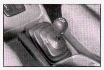
The transfer case shift lever is on the floor to the right of the driver. Use this lever to shift into and out of four-wheel drive. An indicator light comes on when the transfer case is in four-wheel drive.
