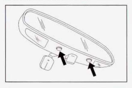
Push the buttons on the bottom of the mirror to turn the reading lamps on and off.
