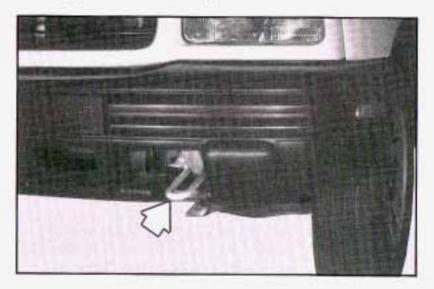
Your vehicle is equipped with recovery hooks. The hooks are provided at the front and rear of your vehicle. You may need to use them if you're stuck off-road and need to be pulled to some place where you can continue driving.
