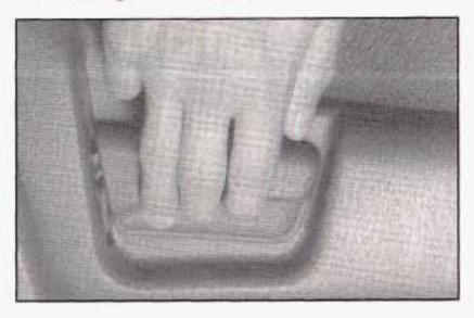
To adjust the seatback, lift the lever on the outboard side of the seat cushion. Release the lever to lock the seatback where you want it. Pull up on the lever, and the seat will go to its original upright position.
