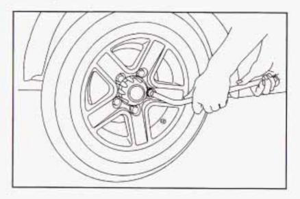
If your vehicle has wheel nut caps, remove them by turning the wheel wrench counterclockwise.
