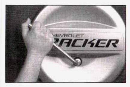
Using the wheel wrench, remove the wheel cover nut. Gently pry the spare tire cover off the wheel.
