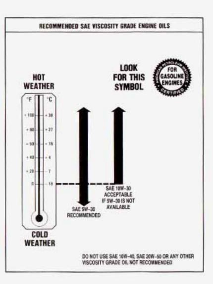
As in the chart shown previously, SAE 5W-30 is the only viscosity grade recommended for your vehicle. You should look for and use only oils which have the API Starburst symbol and which are also identified as SAE 5W-30. If you cannot find such SAE 5W-30 oils, you can use an SAE 10W-30 oil which has the API Starburst symbol, if it's going to be 0°F (-18°C) or above. Do not use other viscosity grade oils, such as SAE 10W-40 or SAE 20W-50 under any conditions.
