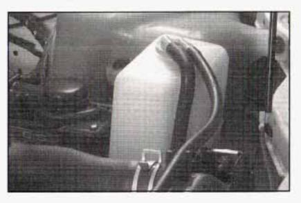
The coolant recovery tank is located toward the front of the engine compartment on the driver's side of the vehicle. See Engine Compartment Overview on page 5-12 for more information on location.
