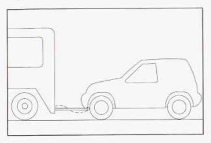
Notice: If your vehicle is a two-wheel drive model, do not tow it on all four wheels. If you do, your transmission could be damaged and the damage would not be covered by your warranty. Follow these steps:
