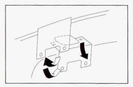
Unfasten the snaps that secure the canvas top to the roof. The snaps are located on both sides of the dome lamp. Reattach the snaps which hold the sunroof canvas in place.
