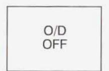
This light comes on when the automatic four-speed transmission, if equipped, has been converted to the three-speed mode and the overdrive is turned off.
