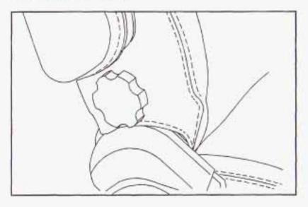
If your vehicle has this feature, turn the knob located on the driver's side seatback clockwise or counterclockwise to adjust support of the lower back.
