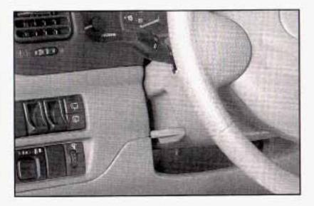
The lever that allows you to tilt the steering wheel is located on the left side of the steering wheel column.
