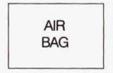
This light will come on when you start your vehicle, and it will flash for a few seconds. Then the light should go out. This means the system is ready.
