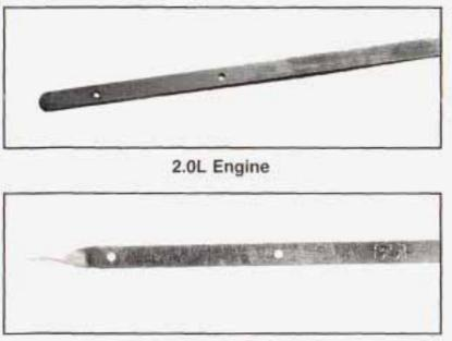
Notice: Don't add too much oil. If your engine has so much oil that the oil level gets above the upper mark that shows the proper operating range, your engine could be damaged.
