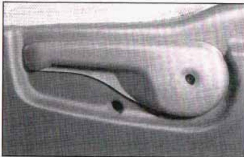
To adjust the seatback, pull up on the lever located on the outboard sides of both the driver's and the front passenger's seats. It is easier to recline the seat if you lean forward, taking your weight off the seatback.
