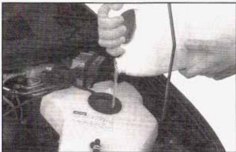
9. Then fill the coolant recovery tank to the FULL COLD mark.
