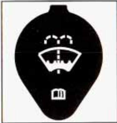
Open the cap with the washer symbol on it. Add washer fluid until the tank is full.
