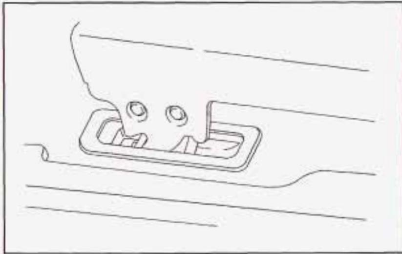
2. The seat can then be lifted off the front floor pins and removed from the vehicle.
