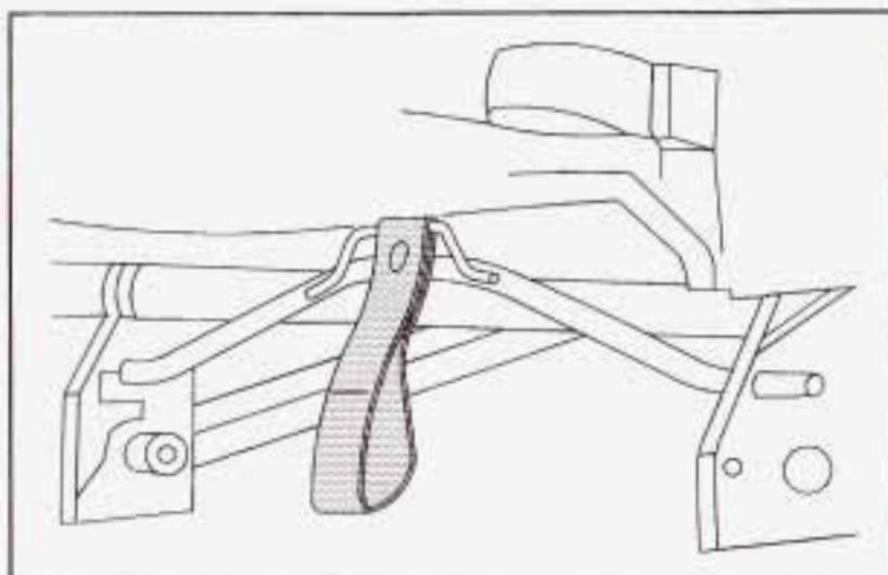
5. From behind the bench seat, pull the nylon strap at the center of the base of the seat to release the rear latches from the floor pins.
