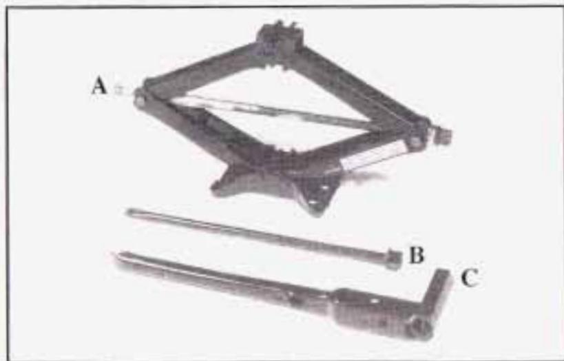
The tools you'll be using include the jack (A), extension (B) and folding wrench (C).
