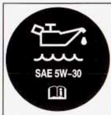
The engine oil fill cap is located behind the engine oil dipstick. See *Engine Compartment Overview on page 5-12* for more information on location.
