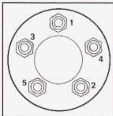
9. Tighten the wheel nuts firmly in a crisscross sequence, as shown.
