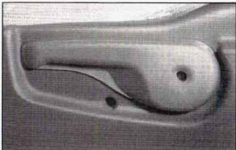
To recline the seatback, lift up on the recliner lever, located on the outboard side of the seat. Use the recliner lever to move the seatback to the desired position.
