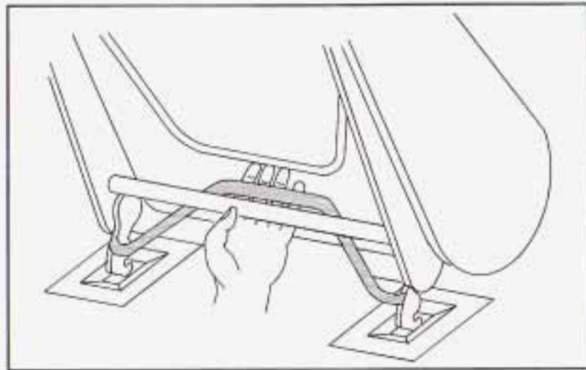
4. To unlatch the front latches, with the seat folded forward, squeeze the angled bar toward the straight crossbar.
