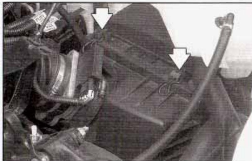
1. Remove the two clamps on the duct.
