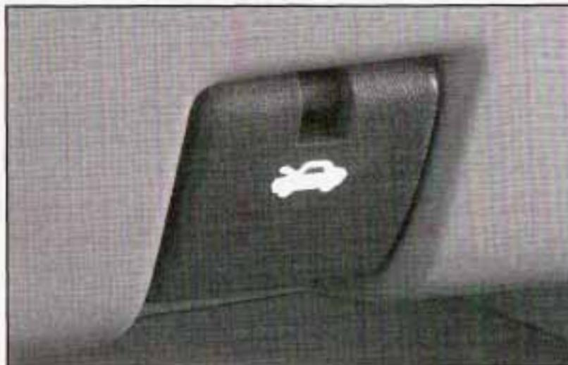
1. Pull the hood release handle, located on the driver's side under the instrument panel.
