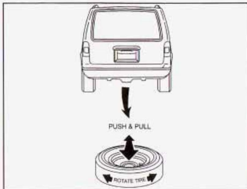
6. Make sure the tire is stored securely. Push, pull, and then try to rotate or turn the tire. If the tire moves, use the folding wrench to tighten the cable.
