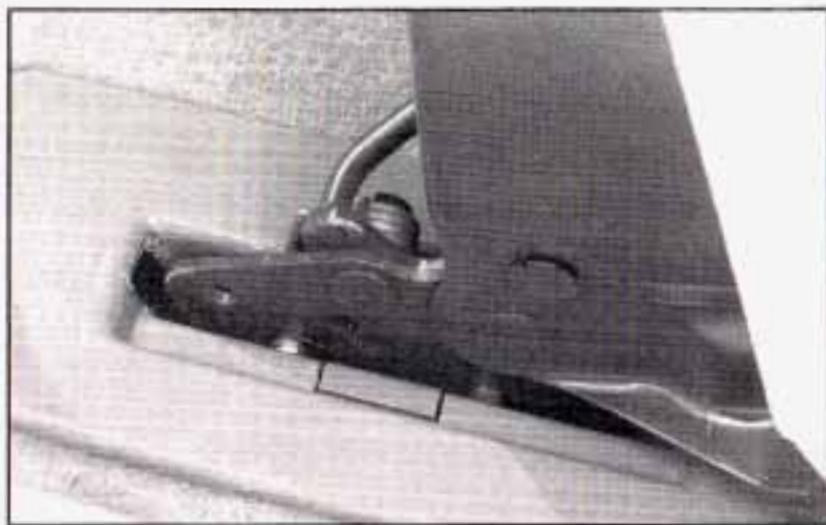
4. Firmly push the rear hooks onto the rear floor pins by pushing down the rear of the seat.
