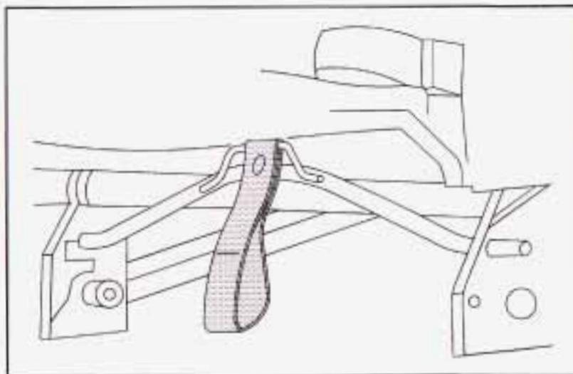
3. From behind the seat, pull the nylon strap, located at the base of the seat, to release the rear latches from the floor pins.
