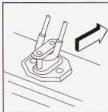
7. Make sure the metal tube is centered at the striker. Push the tube towards the front of the vehicle.
