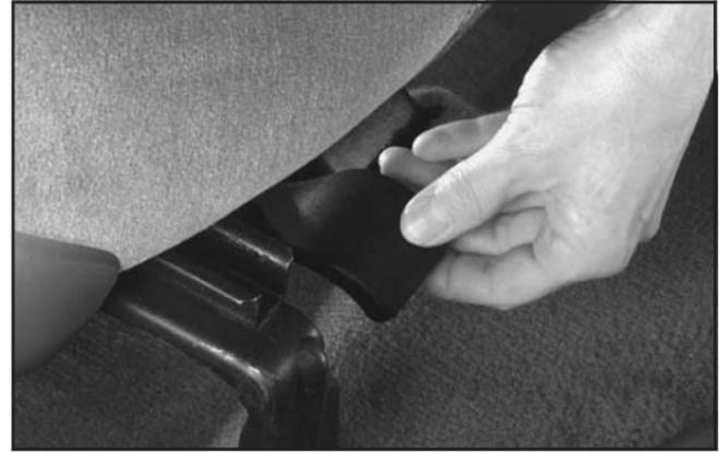
If your vehicle is equipped with easy entry seats, this is your front passenger seat adjuster. Pull up on the lever located at the front of the passenger's seat to unlock it. Slide the seat to a comfortable position and release the lever. Then try to move the seat with your body, to make sure the seat is locked into place.
