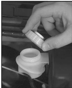
Refer to the Maintenance Schedule to determine how often you should check the fluid level in your master cylinder reservoir and for the proper fluid. See *Part B: Owner Checks and Services* on page 6-18 and *Part D: Recommended Fluids and Lubricants* on page 6-25.
