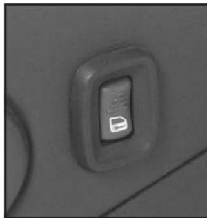
If your vehicle has this feature, you can lock or unlock all the doors on your vehicle from the driver's or front passenger's door lock switch.
