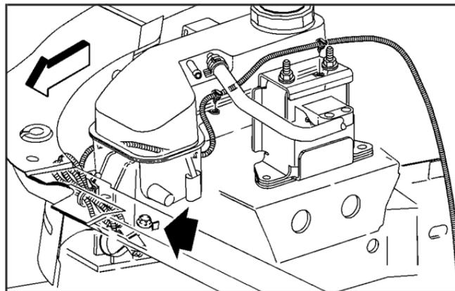
If your vehicle has this feature, in very cold weather 0°F (-18°C) or colder, the engine coolant heater can help. You'll get easier starting and better fuel economy during engine warm-up. Usually, the coolant heater should be plugged in a minimum of four hours prior to starting your vehicle. At temperatures above 32°F (0°C), use of the coolant heater is not required.
