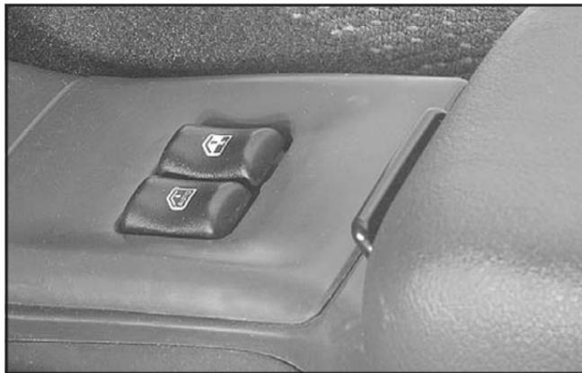
If your vehicle has this feature, the switches on the center console control each of the power windows when the ignition is on. In addition, on four-door models, each rear passenger door has a control switch for that window.
