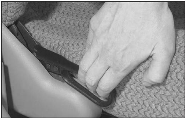
To adjust the seatback, lift the lever located on the outboard side of the seat and move the seatback to where you want it. Release the lever and push rearward on the seatback to make sure it is locked. Pull up on the lever without pushing on the seatback and the seatback will go to an upright position.
