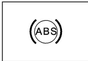
If your vehicle is equipped with the anti-lock brake system, the light will come on when your engine is started and may stay on for several seconds. That's normal.
