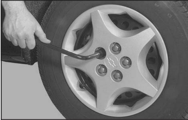
1. If your vehicle is equipped with wheel covers, use the wheel wrench to begin loosening the plastic wheel nut caps. Then you can finish loosening them with your fingers. Using the flat end of the wheel wrench, pry along the edge of the wheel cover until it comes off.
