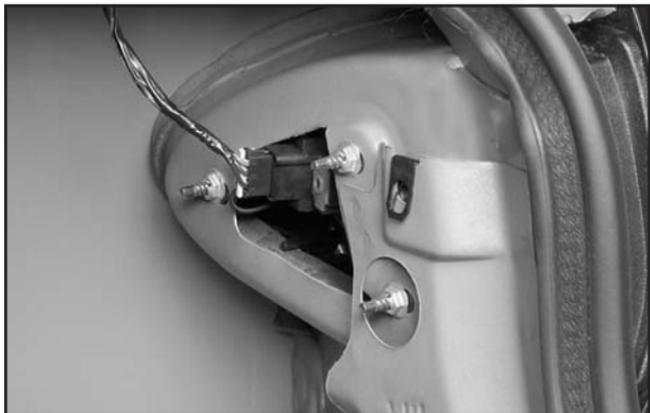
1. Remove the fastener which holds down the trunk trim. On vehicles without a convenience net, pry the fastener loose. On vehicles with a convenience net, remove the net and unscrew the fastener. Then pull down the trunk trim.
