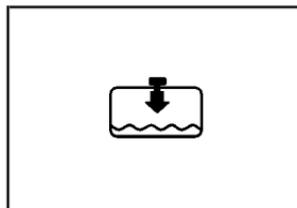
If the low coolant light comes on and stays on, it means you are low on engine coolant. See *Low Coolant Warning Light* on page 3-29.
