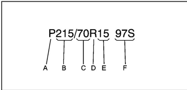
**(A) P-Metric Tire:** The United States version of a metric tire sizing system. The letter “P” as the first character in the tire size means a passenger vehicle tire engineered to standards set by the U. S. Tire and Rim Association.
