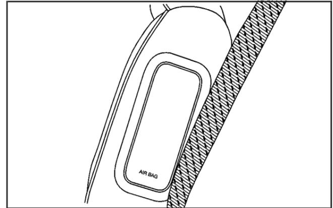
If your vehicle has a side impact air bag for the driver and/or right front passenger, the words AIR BAG will appear on the air bag covering on the side of the seatback closest to the door.
