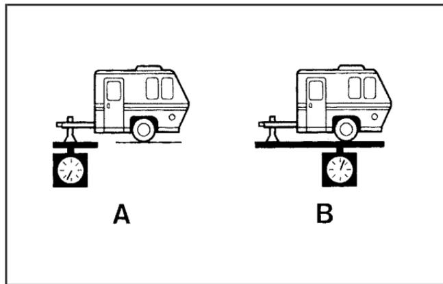
If you are using a weight-carrying hitch, the trailer tongue (A) should weigh 10 to 15 percent of the total loaded trailer weight (B).
