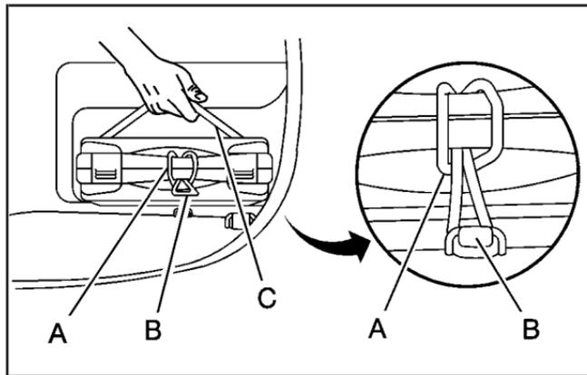
1. Remove the elastic cord (A) from around the retaining hook (B) and slide the kit out from under the elastic band (C) that is secured to the floor of the hatch/trunk area.
