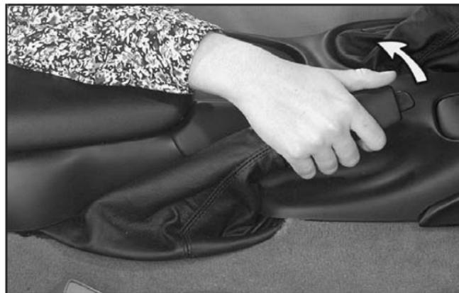
To set the parking brake, hold the brake pedal down. Pull the parking brake lever up. If the ignition is on, the brake system warning light will come on.
