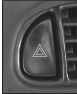
The hazard warning flasher button is located on the instrument panel above the audio system.
