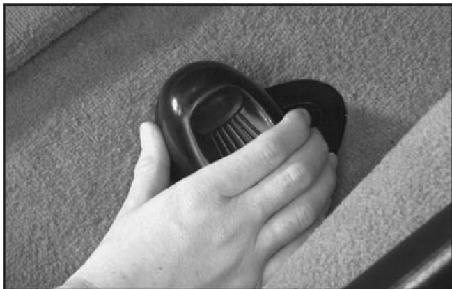
4. Make sure to install the two egg-shaped storage receivers into the floor of the rear storage compartment. Secure both receivers into their proper positions by turning them counterclockwise.
