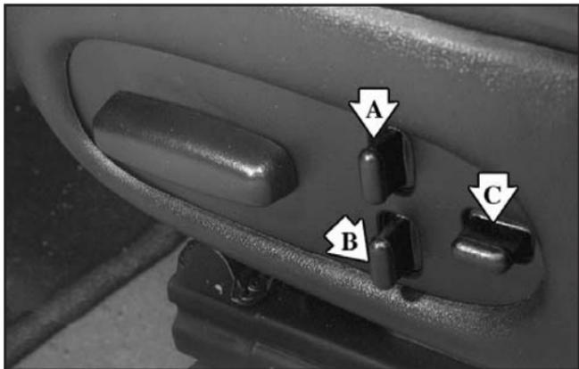
If your vehicle has this feature, there are three other controls that help you change the shape of the seat in addition to the power seat control. There are two lumbar supports for the middle (A) and lower (B) back. There is also a side bolster control (C) that adjusts the sides of the seat around you to give you more lateral support.
