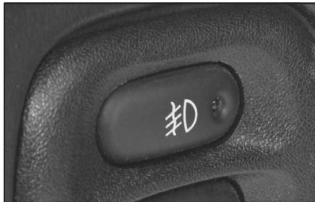
Your vehicle may have this feature. Use the fog lamps for better vision in foggy or misty conditions. Your parking lamps or low-beam headlamps must be on or the fog lamps will not work.
