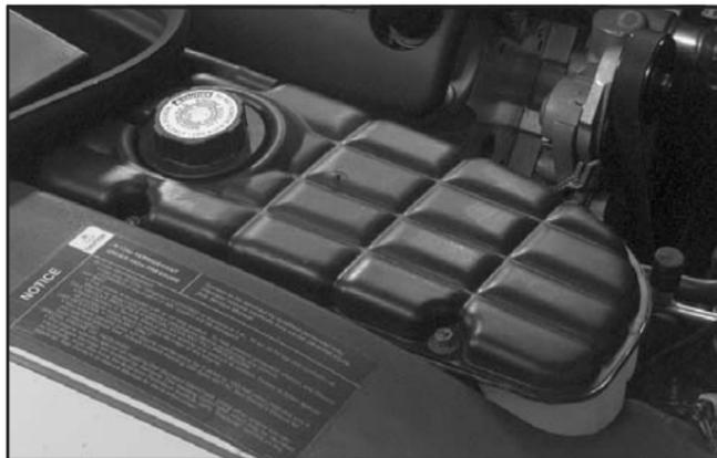
The coolant surge tank is located in the engine compartment behind the passenger's side headlamp. See *Engine Compartment Overview* on page 5-12 for more information on location.
