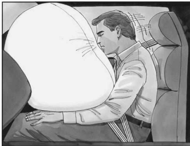
The passenger's air bag is in the instrument panel on the passenger's side.
