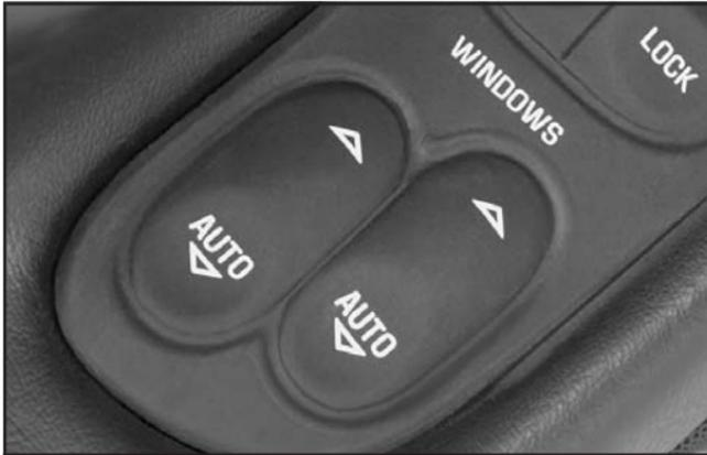
Both driver's and passenger's window switches have the express-down feature. Tap AUTO and immediately release. The window will lower completely. To stop the express-down feature from lowering the window completely, simply tap the switch again.
