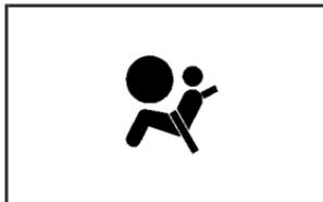
There is an air bag readiness light on the instrument panel, which shows the air bag symbol.
