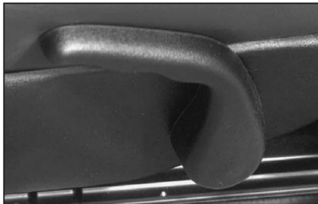
The lever for the reclining seatback is located on the outboard side of each seat, near the base.
