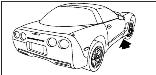
The front lifting point can be accessed for either the driver's or passenger's side of the vehicle, behind the front tires.
