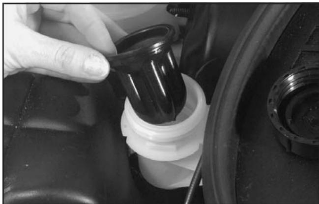
Fluid should be added if the fluid level is below the step on the inside of the reservoir. There are additional instructions on the reservoir cap. Put the rubber seal and cap back on. See *Engine Compartment Overview* on page 5-12 for more information on location.
