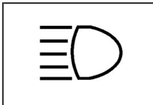
While the high beams are on, this light on the instrument panel cluster also will be on. To change the headlamps from high to low, pull the lever rearward.
