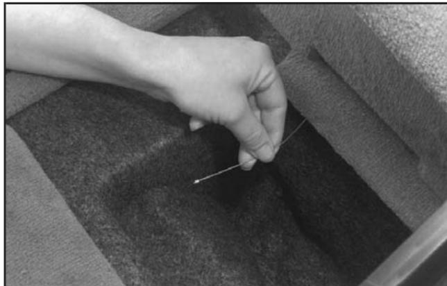
Pull each cable straight down for each latch to release the hatch.
