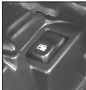
The fuel filler door release button is located inside of the center console storage compartment.
