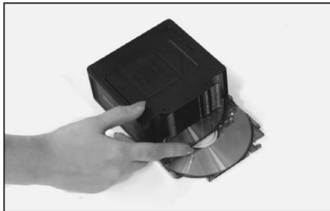
You must first load the magazine with CDs before you can play a CD. Each of the 12 trays holds one CD. Press the button on the back of the magazine and pull gently on one of the trays. Load the trays from bottom to top, placing a CD on the tray label side down. If you load a CD label side up, the CD will not play and an error will occur. Gently push the tray back into the magazine slot. Repeat this procedure for loading up to 12 CDs in the magazine.
