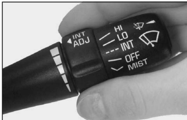
Use this lever located on the right side of the steering column to operate the windshield wipers.
