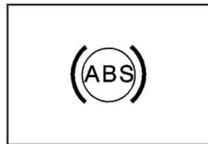
If there is a problem with the anti-lock brake system, this warning light will stay on. See *Anti-Lock Brake System Warning Light* on page 3-39.
