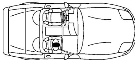
Your vehicle has the LATCH system. You will find anchors (A) for the passenger seat.
