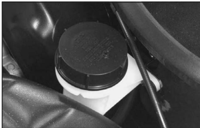
The clutch master cylinder reservoir is located at the rear of the engine compartment on the driver's side. See *Engine Compartment Overview* on page 5-12 for more information on location.
