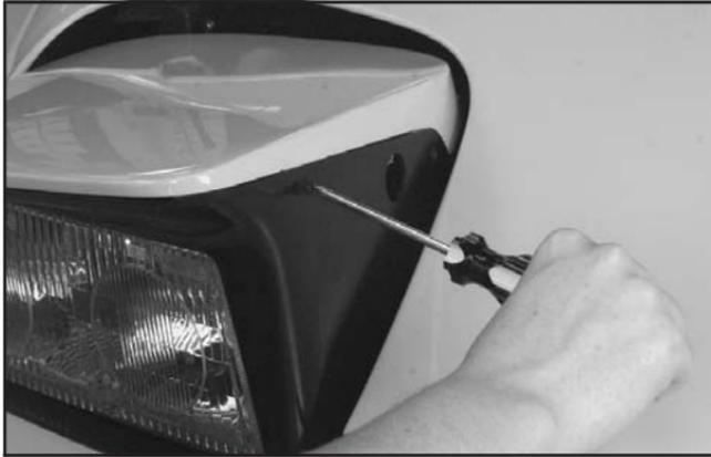
2. Remove the screws on each side of the headlamp bezel.
