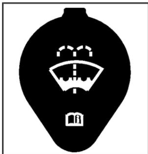
Open the cap with the washer symbol on it. See *Engine Compartment Overview* on page 5-12 for reservoir location. Add washer fluid until the tank is full.
