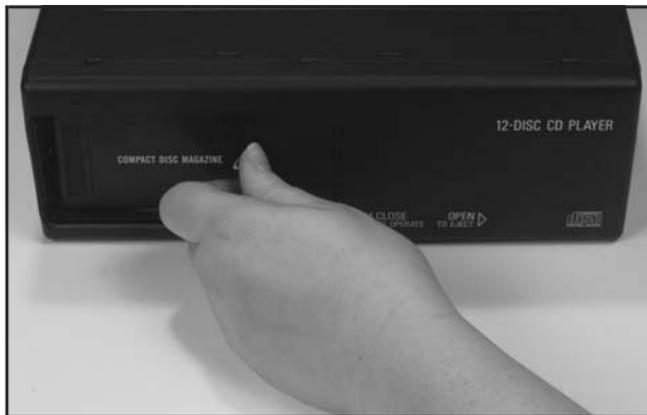
Close the door by sliding it all the way to the left. If the door is left partially open, the changer will not operate and an error will occur. When the door is closed, the changer will begin checking for CDs in the magazine. This will continue for up to two minutes depending on the number of CDs loaded.
