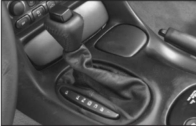
2. Move the shift lever into PARK (P) by holding in the button on the lever and pushing the lever all the way toward the front of the vehicle.
