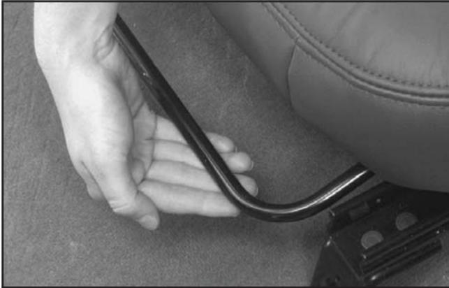
To move a manual seat, pull up on the lever located in front of the seat to unlock it. Slide the seat to where you want it and release the lever. Then try to move the seat with your body to make sure the seat is locked into place.
