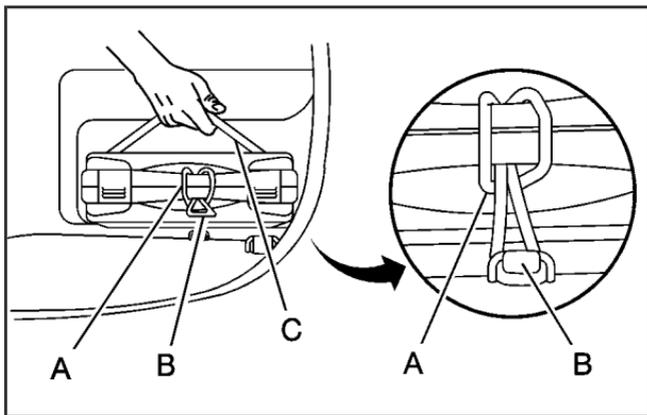
2. Insert the tire inflator kit under the elastic band (C) that is secured to the floor of the hatch/trunk area of your vehicle.
