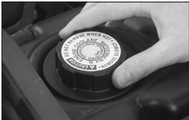
1. Park the vehicle on a level surface. You can remove the coolant surge tank pressure cap when the cooling system, including the coolant surge tank pressure cap and upper radiator hose, is no longer hot. Turn the pressure cap slowly counterclockwise about one-quarter turn and then stop.
