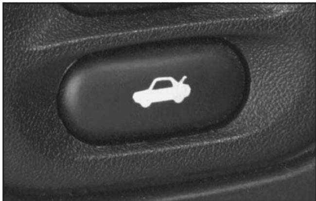
To use the hatch/trunk lid release on vehicles with an automatic transmission, your vehicle must be in PARK (P) or NEUTRAL (N). For manual transmissions, set the parking brake. See *Parking Brake* on page 2-31.
