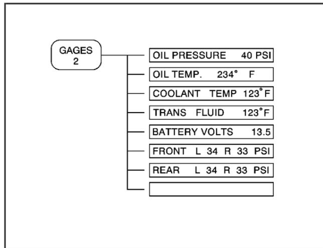
Press the GAGE button to display the oil pressure, such as:
