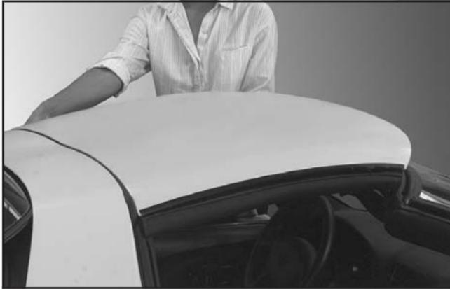
9. Stand on one side of the vehicle and, if necessary, have your helper stand on the other side. Together, carefully lift the front edge of the panel up and forward, and out of the vehicle opening.
