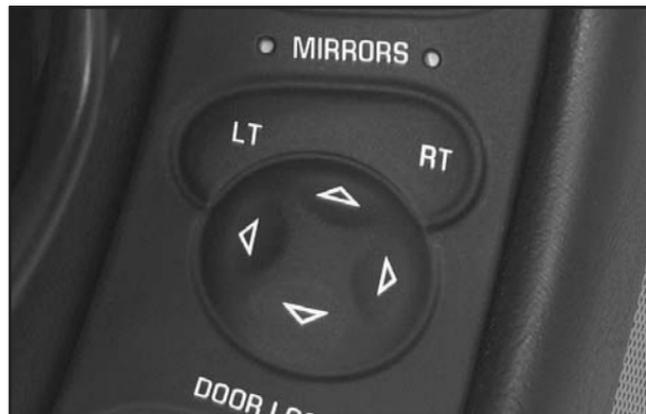
The power mirror control is on the driver's door. It controls the driver's and passenger's mirrors.
