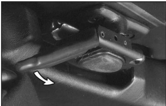
3. Unlock the front of the convertible top by lowering the latch handles and turning them inward. Push the latch handles back to the up position.
