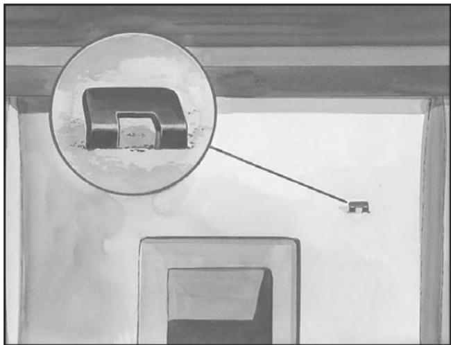
If your vehicle is a Z06, an anchor bracket for a top strap is located behind the passenger's seat in the cargo area. Anchor the top strap to the bracket.
