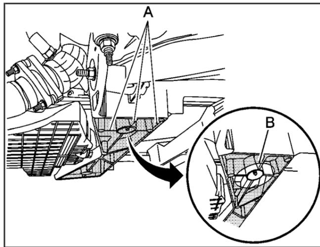
1. Locate the lifting point (B) on either side of your vehicle to jack the vehicle according to the illustration shown.
