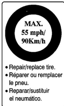
The maximum speed label reminds you to drive cautiously and not to exceed 55 mph (90 km/h) until you have the damaged tire inspected and repaired.
