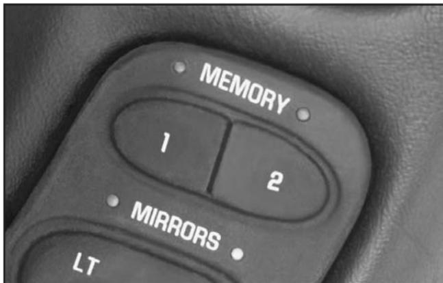
If your vehicle has this feature, MEMORY can store and recall the settings for the driver's seat position, the outside rearview mirror positions, telescopic steering column (if equipped), radio presets, tone, volume, playback mode (AM/FM, tape or CD), last displayed station, compact disc position and tape direction and the last climate control setting.
