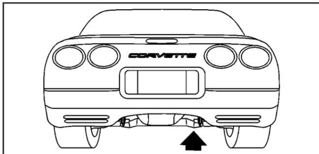
The rear lifting point can be accessed from the rear of the vehicle, on either the driver's or passenger's side.
