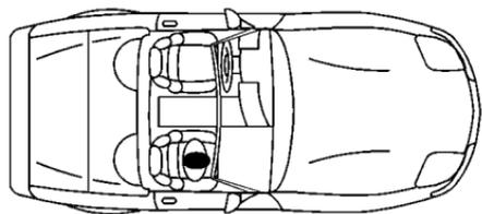
Your vehicle has a passenger air bag. There is an air bag off switch in the glove box you can use to turn off the passenger's air bag when you need to secure a child restraint in the passenger position. See *Air Bag Off Switch* on page 1-46 for more on this including important safety information.
