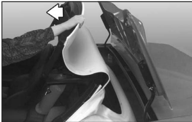
2. Tilt the driver's seat forward and press the storage compartment release button, or use the manual release cable if battery power has been lost. Lift the storage compartment lid (C).
