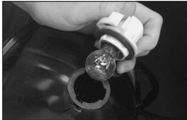
4. Remove the bulb from the socket.
