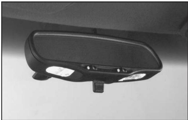
Your inside rearview mirror includes two reading lamps. The lamps will go on when a door is opened. When the doors are closed, each lamp can be turned on individually by pressing the switch for that lamp.
