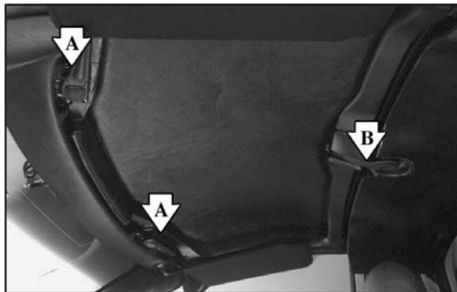
There are two latches on the front of the roof panel near each door (A), and one rear latch (B).
