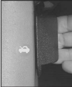
1. Pull the handle located inside the vehicle below the instrument panel on the driver's side.
