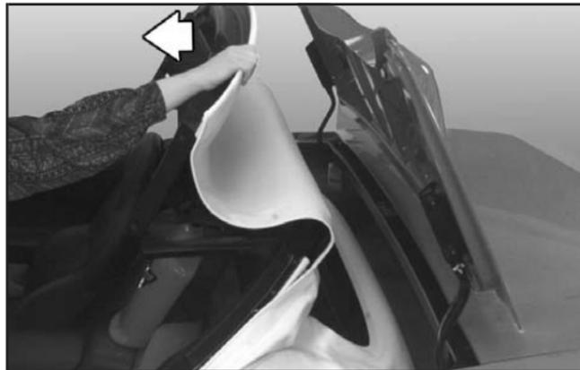
3. Pull the top up by firmly gripping the front edge (A) of the convertible top with your hand and applying a brisk, firm upward and forward motion to get the top in the full-up position.
