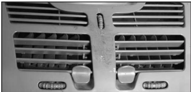
Use the horizontal thumbwheels on the air outlets, located in the center and on the sides of the instrument panel, to change the direction of the airflow. Airflow can be shut off at the center upper outlet by turning the vertical thumbwheel. The other outlets can be shut off by closing the outlet vanes.
