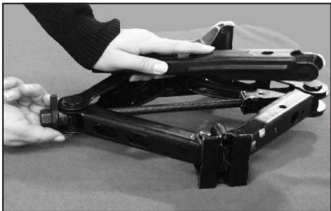
2. Turn the plastic wing nut counterclockwise to loosen wheel wrench.
