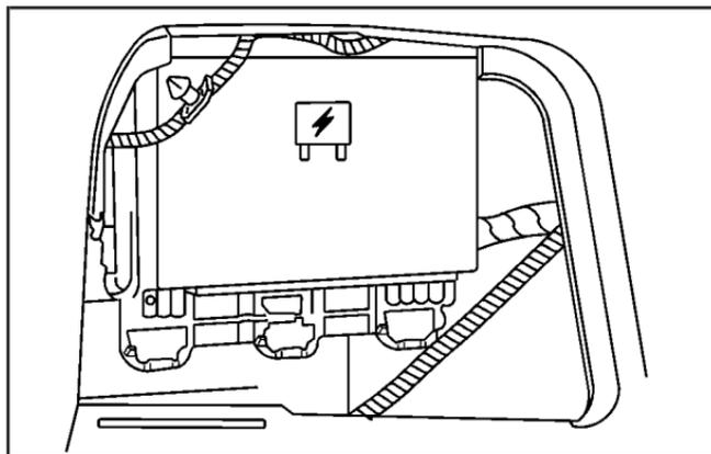
The rear compartment fuse block is located in the trunk of the vehicle. Access the fuse block through the trunk panel on the driver's side of the rear cargo area.
