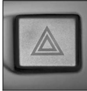
The hazard warning flasher is located near the center of the instrument panel.
