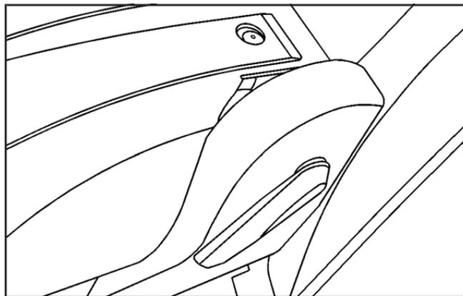
2. Once a lever is pulled, the seatback can be pushed into the down position.
