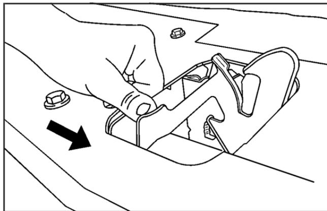
2. Then go to the front of the vehicle and push the secondary hood release handle toward the driver's side of the vehicle before lifting the hood.
