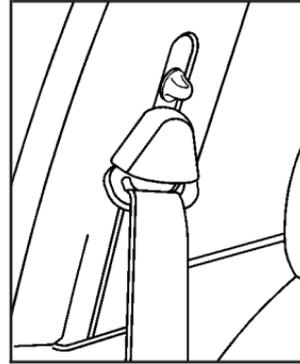
To move it down, push down the release button and move the height adjuster to the desired position. You can move the adjuster up by pushing the release button up. After you move the adjuster to where you want it, try to move it without pushing the release button to make sure it has locked into position.
