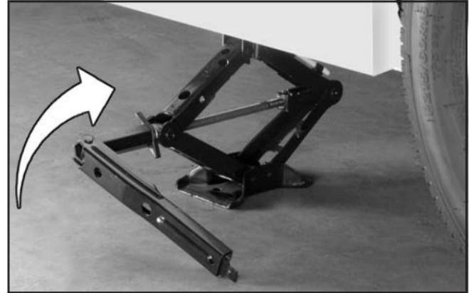
5. Raise the vehicle by turning the wrench clockwise. Raise the vehicle far enough off the ground so there is enough room for the compact spare tire to fit.
