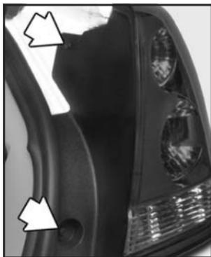
2. Unscrew the two fasteners located on the inside of the trunk at the rear of the vehicle.
