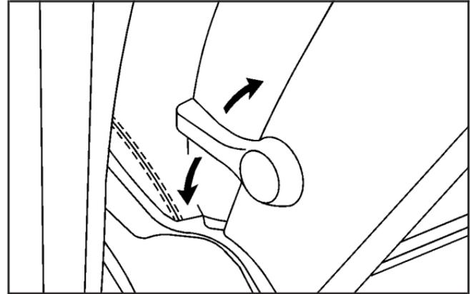
If your vehicle has this feature, the handle is located on the outboard side of the driver's seat. Push the handle down to increase lumbar support. Pull the handle up to decrease lumbar support.
