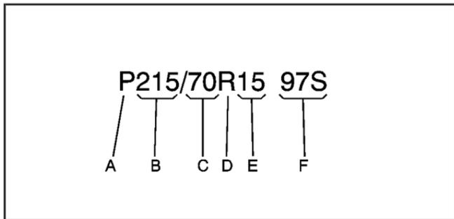
**(A) P-Metric Tire:** The United States version of a metric tire sizing system. The letter "P" as the first character in the tire size means a passenger vehicle tire engineered to standards set by the U. S. Tire and Rim Association.
