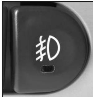
If your vehicle has this feature, the button for the fog lamps is located on the instrument panel, to the left of the steering wheel.
