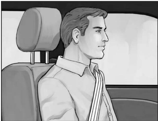
The head restraints are adjustable. Press the button on the side of the post to adjust the head restraint. Slide the head restraint up or down so that the top of the restraint is closest to the top of your head. This position reduces the chance of a neck injury in a crash.
