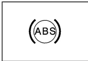
If your vehicle has the anti-lock brake system, the light will come on when your engine is started and may stay on for several seconds. That's normal.
