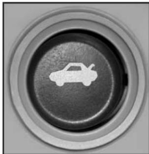
Press the remote release button, located on the lower edge of the driver's door, to open the trunk lid or the liftgate.
