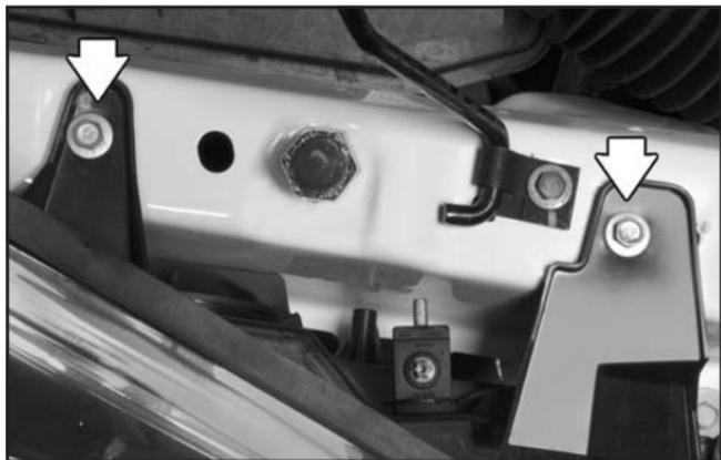
2. Carefully remove the two bolts attaching the headlamp assembly to the vehicle.
