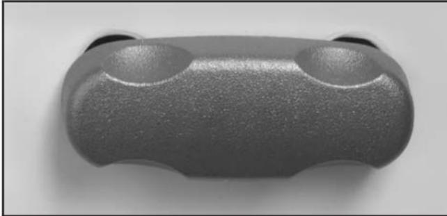
If your vehicle has this feature, the power seat control is located on the outboard side of the driver's seat.
