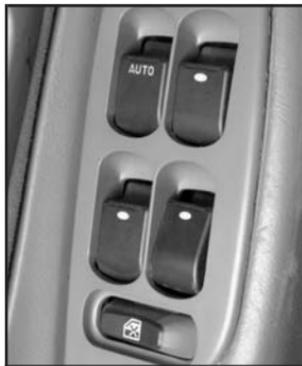
The power window switches are located on the armrest on the driver's door. In addition, each passenger door has a switch for its own window.
