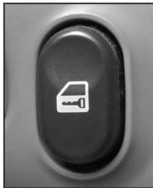
With the power door locks, you can unlock or lock all the doors and the liftgate on your vehicle using either the driver's or front passenger's door lock switch.
