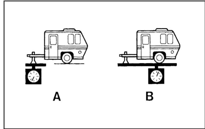
If you're using a weight-carrying hitch or a weight-distributing hitch, the trailer tongue (A) should weigh 10 to 15 percent of the total loaded trailer weight (B).
