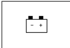
The charging system light will come on when you turn on the ignition, but the engine is not running, as a check to show you it is working.
