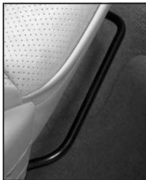
If your vehicle has a manual seat adjustment, lift the bar located under the front of the seat to unlock it.
