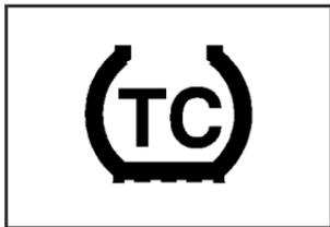
If your vehicle has the Enhanced Traction System (ETS), this light will come on when the system is limiting wheel spin.
