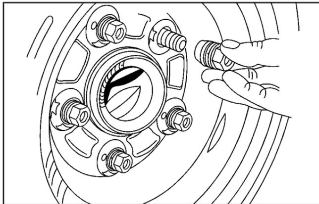
9. Install the compact spare tire. Put the wheel nuts back on with the cone end of the nuts toward the wheel. Tighten each nut by hand or with the wrench until the wheel is held against the hub.
