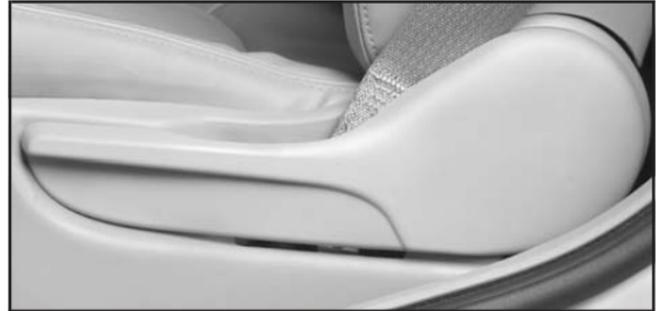
To adjust the seatback, lift the lever located on the outboard side of the seat and move the seatback to the desired position. Release the lever to lock the seatback. Pull up on the lever without pushing on the seatback, and the seatback will return to the upright position.
