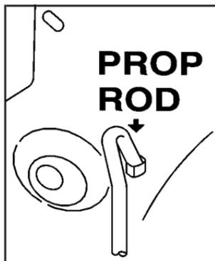
4. Release the hood prop rod from its retainer and put the hood prop into the slot marked with an arrow.
