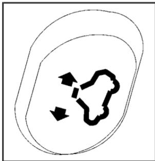
If your vehicle has this feature, the switch is located on the overhead console between the sun visors. The sunroof will only operate when the ignition is in ACC or ON or while in retained accessory power.
