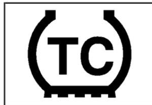
This light will come on when your Enhanced Traction System is engaged and limiting wheel spin.
