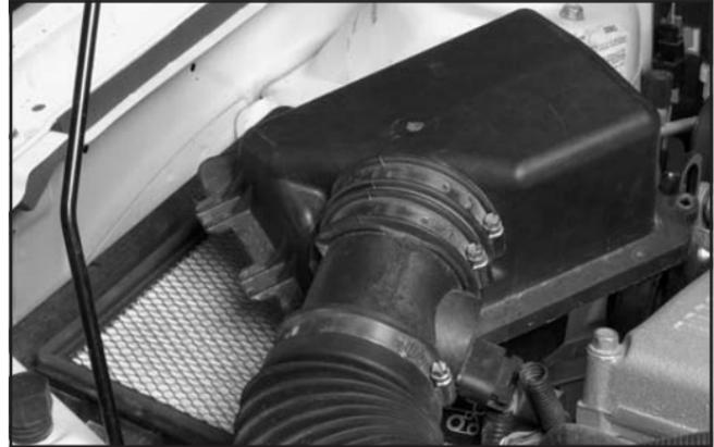
1. Remove the screws that hold the cover on.
