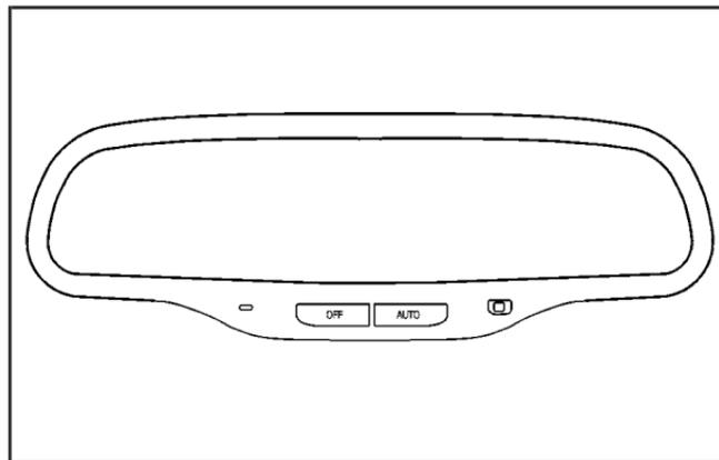
Your vehicle may have an automatic dimming rearview mirror. This feature enables the mirror to sense nighttime glare from vehicle headlamps from behind and automatically dim to reduce the glare to a safe level.
