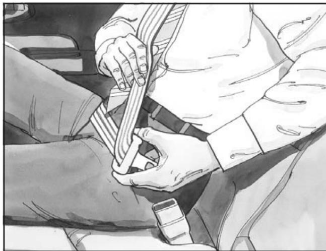
If the belt stops before it reaches the buckle, tilt the latch plate and keep pulling until you can buckle it. Pull up on the latch plate to make sure it is secure. If the belt is not long enough, see *Safety Belt Extender on page 1-30*.
