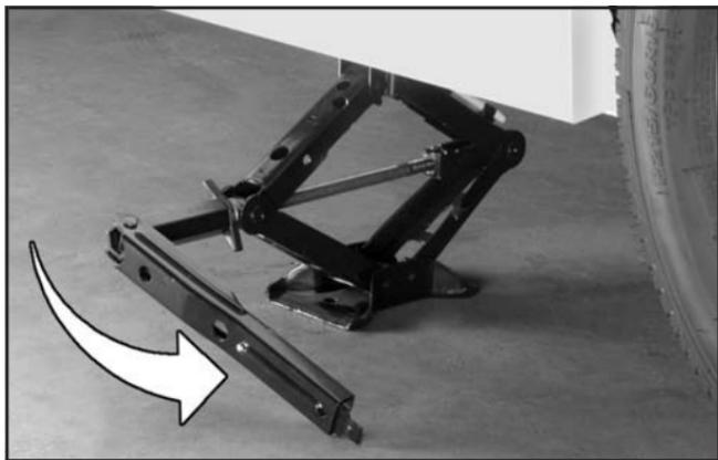
10. Lower the vehicle by turning the wrench counterclockwise. Lower the jack completely.
