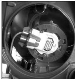
5. Unclip the wiring harness and twist the socket less than one-quarter turn counterclockwise and remove it.
