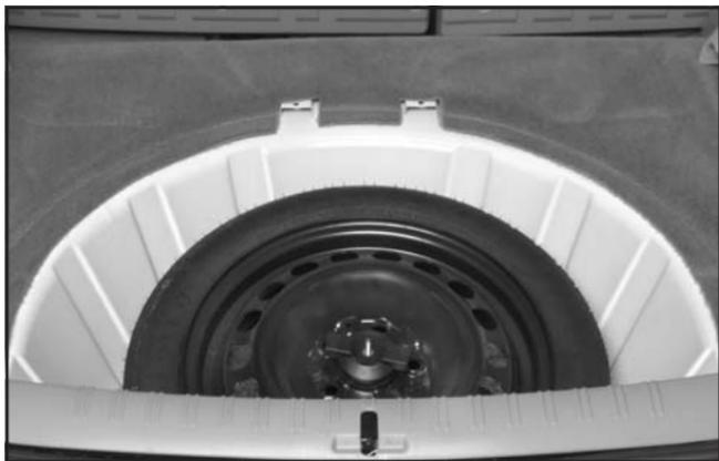
1. For the sedan model, lift the handle on the spare tire cover. The handle may hook on the trunk front edge weatherstrip to hold the cover out of the way. For the MAXX model, lift the handle to release the latch on the spare tire cover.
