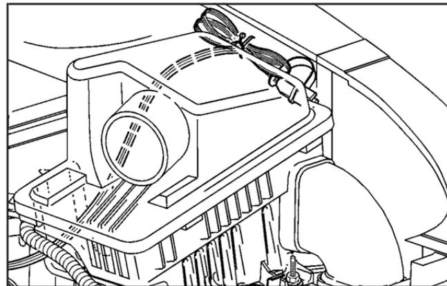
In very cold weather, 0°F (-18°C) or colder, the engine coolant heater, if your vehicle has this feature, can help. You'll get easier starting and lower fuel usage during engine warm-up. Usually, the coolant heater should be plugged in a minimum of four hours prior to starting your vehicle. At temperatures above 32°F (0°C), use of the coolant heater is not required.
