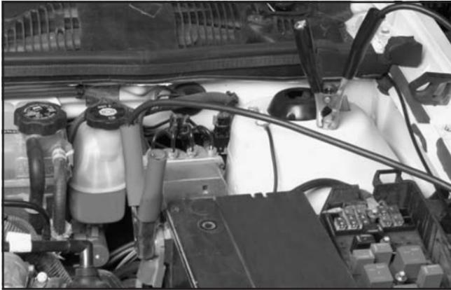
9. Connect the other end of the negative (-) cable at least 18 inches (45 cm) away from the dead battery, but not near engine parts that move. The electrical connection is just as good there, and the chance of sparks getting back to the battery is much less. If the THEFT SYSTEM light flashes, wait until the light stops flashing.
