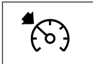
If your vehicle has cruise control, this light appears on your instrument panel cluster whenever the cruise control is engaged.
