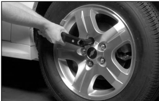
1. If your vehicle has a wheel cover or hubcap that has plastic wheel nut caps, loosen the plastic nut caps. You may need to use the wheel wrench to loosen them. Do not pry off wheel covers or center caps that have plastic wheel nut caps.
