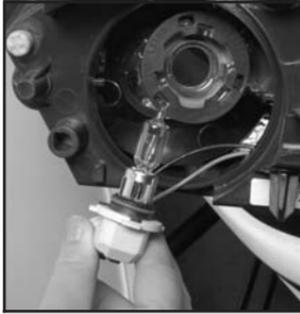
6. Gently wiggle the bulb from the socket. Replace the old bulb with a new bulb.
