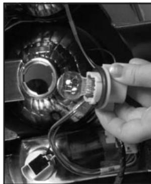
6. Gently wiggle the bulb to remove it from the socket. Replace the bulb.
