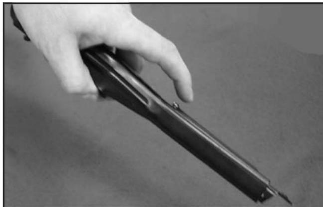
4. Before using the wheel wrench, you must extend the handle.
