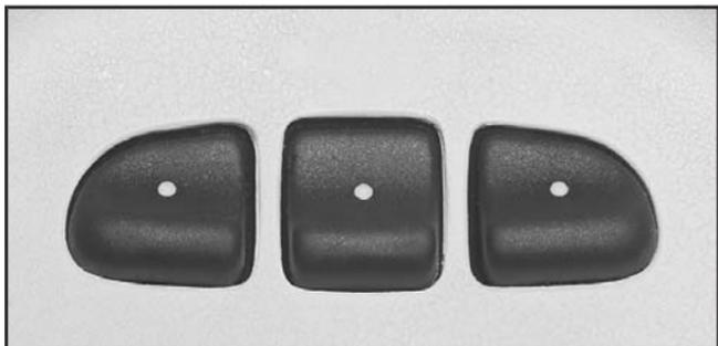
HomeLink, a combined universal transmitter and receiver, provides a way to replace up to three hand-held transmitters used to activate devices such as gate operators, garage door openers, entry door locks, security systems and home lighting. Additional HomeLink information can be found on the internet at [www.homelink.com](http://www.homelink.com) or by calling 1-800-355-3515.
