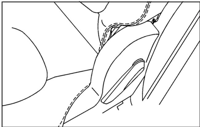
1. Pull up on and hold the lever located on the side of either rear seat.
