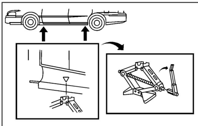
4. Position the lift head at the jack location nearest the flat tire. Make sure all of the jack lift head is touching the jacking flange under the body. Do not place the jack under a body panel. The lower body panel has an arrow to aid in locating the jacking location. Put the compact spare tire near you.
