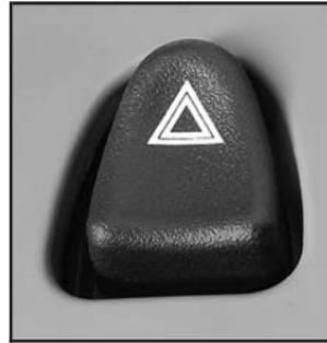
The hazard warning flasher is located at the top of the steering column.
