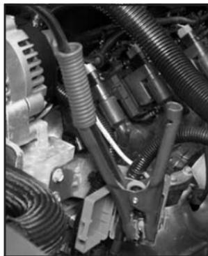
6. Connect the red positive (+) cable to the positive (+) terminal of the vehicle with the dead battery. Use a remote positive (+) terminal if the vehicle has one.
