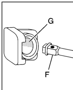
3. Insert the hoist end (F) of the extension through the hole (G) in the rear bumper.
