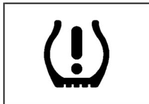
If your vehicle is equipped with the Tire Pressure Monitor system, this light will come on if the system detects low tire pressure.
