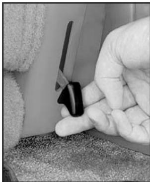
2. Fold the seatback forward onto the seat cushion by using the lever labeled 1. The seat cannot be removed unless the seatback is folded.
