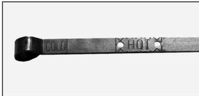
3. Check both sides of the dipstick, and read the lower level. The fluid level must be in the COLD area, below the cross-hatched area, for a cold check or in the HOT area or cross-hatched area for a hot check. Be sure to keep the dipstick pointed down to get an accurate reading.
