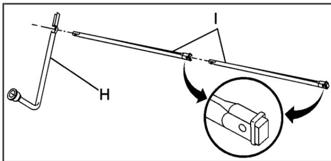
3. Attach the wheel wrench (H) and extensions (I) together.
