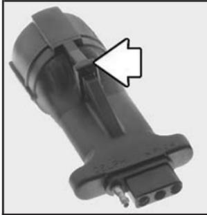
This adapter is included with your vehicle as part of the heavy-duty trailer wiring package.
