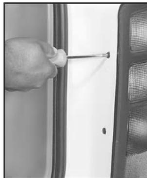
1. Use a tool to remove the two screws from the lamp assembly.
