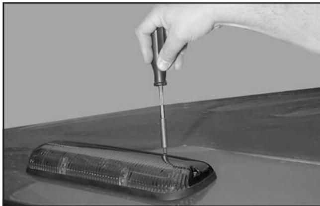
2. Remove the six screws on the center roof marker lamps.
