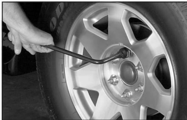
1. Remove the center cap by placing the chisel end of the wheel wrench in the slot on the wheel and gently prying the cap out.
