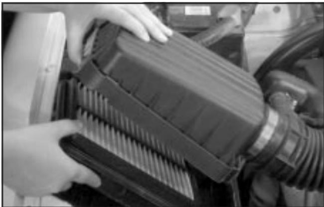
3. Pull out the engine air cleaner/filter and check or replace it.
