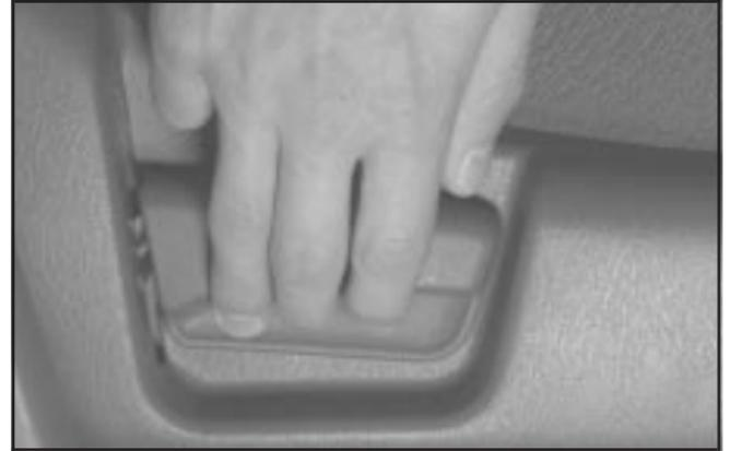
To adjust the seatback, lift the lever on the outboard side of the seat cushion. Release the lever to lock the seatback where you want it. Pull up on the lever, and the seatback will go to the upright position.
