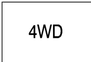
If you have four-wheel drive, this light comes on when the ignition switch is on and the transfer case lever is in one of the four-wheel drive positions.
