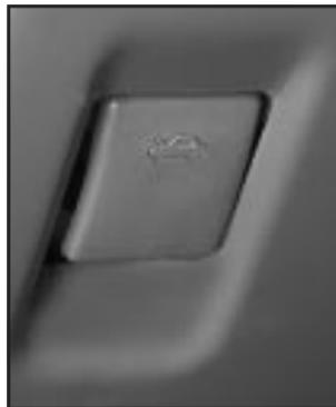
1. Pull the release handle located on the driver's side of the vehicle on the lower portion of the instrument panel.
