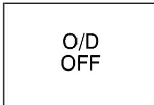
This light comes on when the automatic four-speed transmission, if equipped, has been converted to the three-speed mode and the overdrive is turned off.
