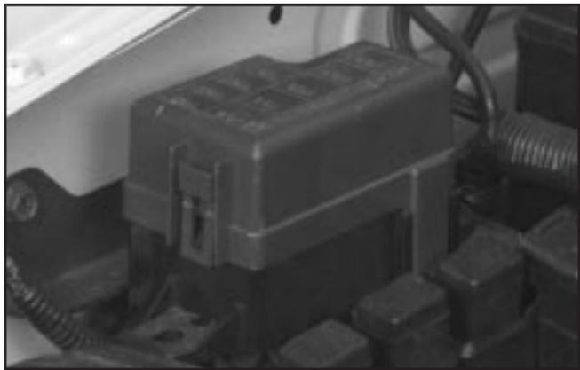
The engine compartment fuse block is located in the engine compartment on the passenger's side of the vehicle and protects all electrical loads. See *Engine Compartment Overview* on page 5-12 for more information on location.
