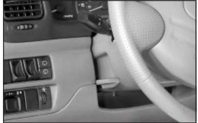
The lever that allows you to tilt the steering wheel is located on the left side of the steering wheel column.
