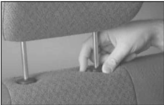
3. Remove the head restraint from the seatback by raising the head restraint fully. Press the release button and remove the head restraint from the seatback.
