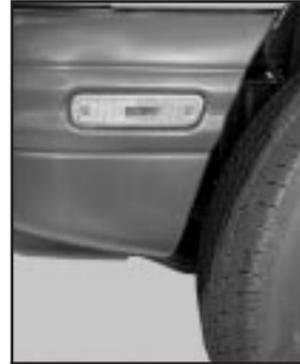
1. Remove the two screws holding the sidemarkers lamp assembly. The assembly should pull away from the vehicle.
