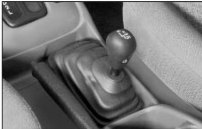
The transfer case shift lever is on the floor to the right of the driver. Use this lever to shift into and out of four-wheel drive. An indicator light comes on when the transfer case is in four-wheel drive.
