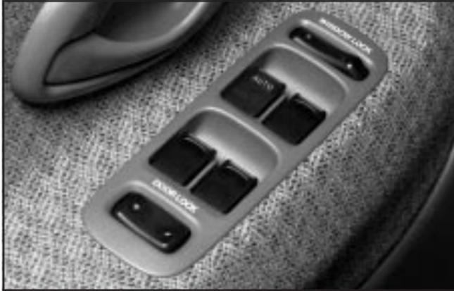
With power windows, switches on the driver's door operate each window while the ignition is on. Push down on the front of the switch to lower a window and lift up the front of the switch to raise a window.
