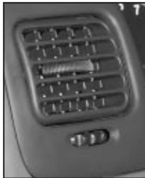
Use the air outlets located in the center and outboard sides of the instrument panel, to change the direction and amount of the air flowing through the vents.
