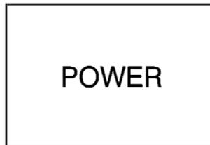
This light comes on when the power mode selector switch, if equipped, is turned to P (power) with the ignition switch in the ON position.
