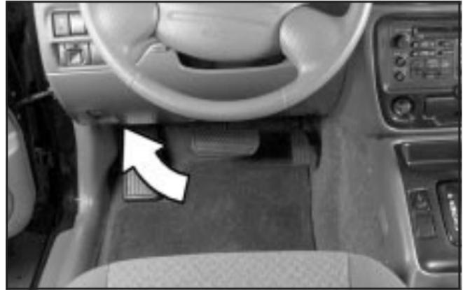
This fuse block is located under the driver's side of the instrument panel. The fuses here protect each separate circuit including headlamps. There are spare fuses inside the fuse box. If you have electrical failure, check here first.
