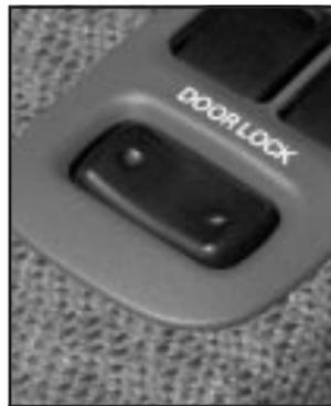
To lock all the doors and the tailgate, press the right side of the switch. To unlock the doors and the tailgate, press the left side of the switch.
