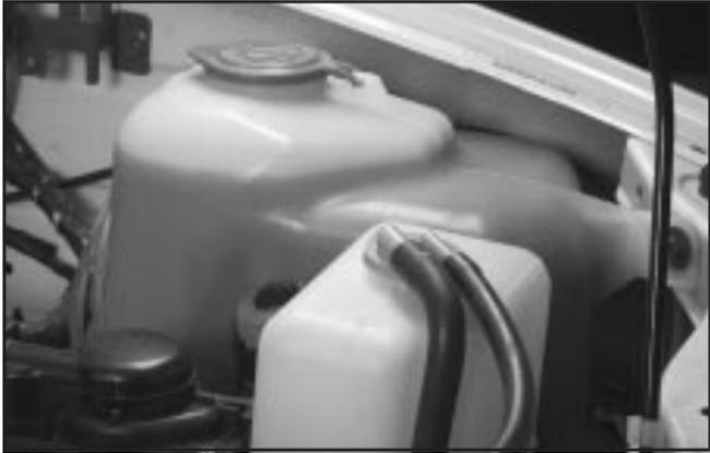
Open the cap with the washer symbol on it. Add washer fluid until the tank is full.
