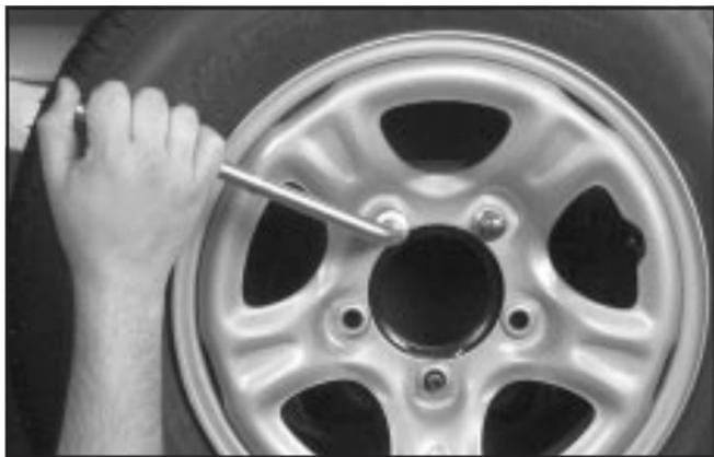
7. Remove the remaining wheel nuts with the wheel wrench.
