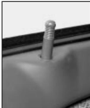
To lock the door from the inside, push down on the manual lock rod located on the door. To unlock it, pull up on the manual lock rod.
