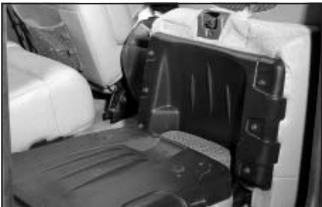
3. Grasp the seatback and pull it toward the front of the vehicle. Push it down until it is flat. You may have to move the front seats forward slightly to do this.
