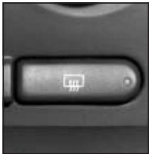
If the vehicle has heated mirrors, the button to turn this function on or off is located on the climate control panel.
