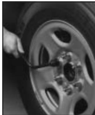
2. Use the wheel wrench to loosen all the wheel nuts. Turn the wheel wrench counterclockwise to loosen the wheel nuts. Don't remove the wheel nuts yet.
