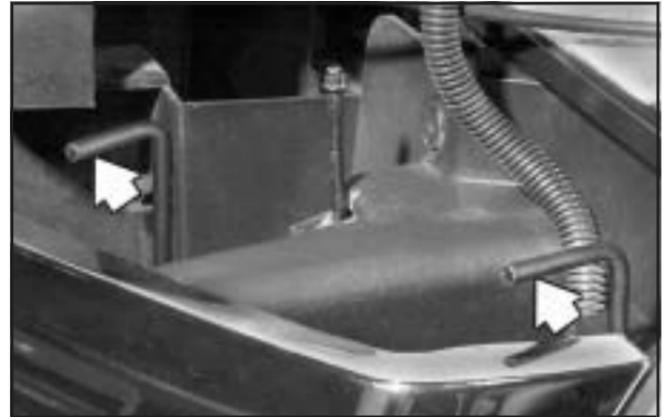
3. Pull the pins away from their clips and pull them up until they completely release from the vehicle.
