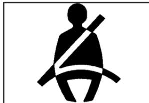
If your vehicle is not equipped with the passenger sensing system, this chime and light will be repeated if the driver remains unbuckled and the vehicle is in motion.
