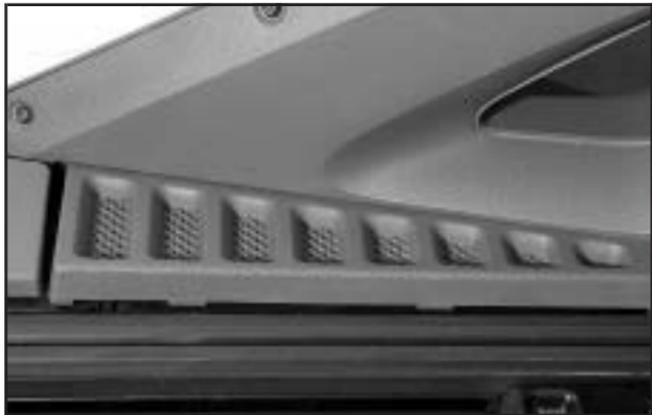
The top drain grates are located near the rear glass on both sides of the vehicle. You may need to clean the grates and drains if there seems to be blockage.
