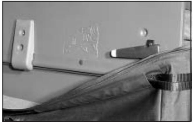
3. Store cargo panel 2 by loading the cargo panel with latches down and facing toward you.
