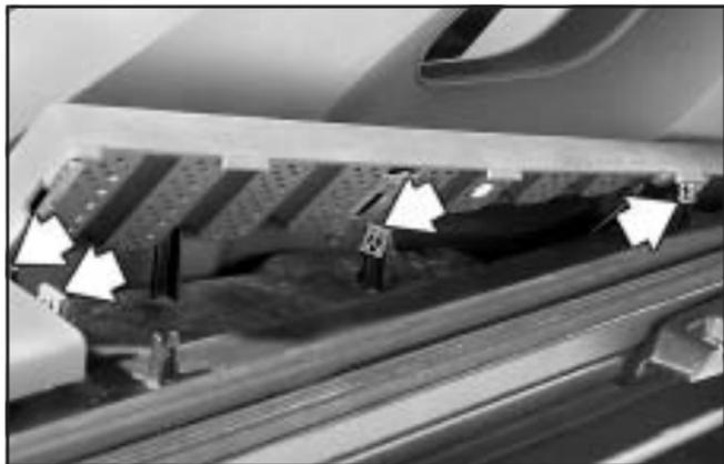
1. Line up the clips on the vehicle with the slots in the grate.
