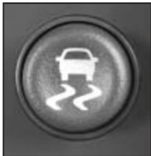
StabiliTrak<sup>®</sup> and part of the traction control system can be turned off or back on by pressing the StabiliTrak<sup>®</sup> button on the instrument panel.
