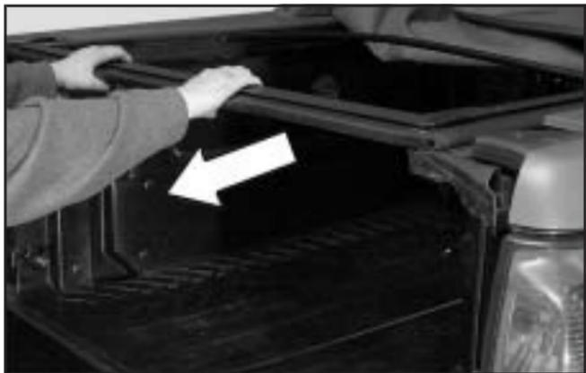
1. Remove the rear rail by pulling it straight out from the side rails. Set the rail aside.
