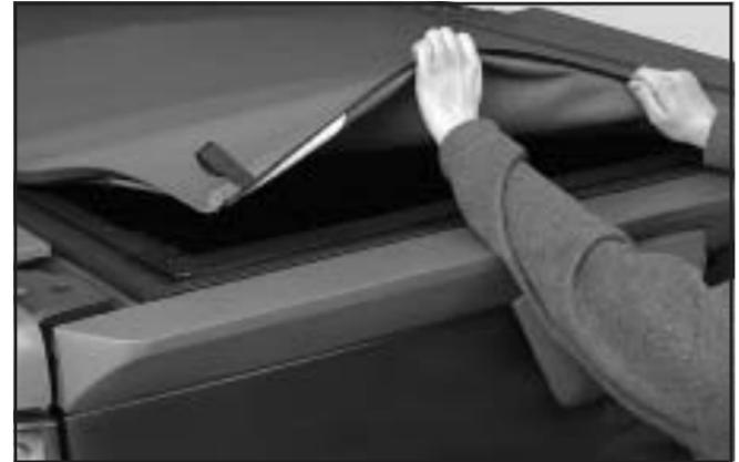
2. Pull the back of the cover out from the rear rail (D).
