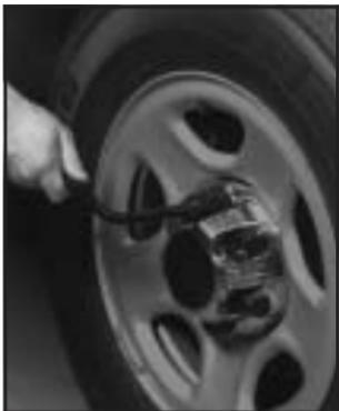
1. If your vehicle has wheel nut caps, loosen them by turning the wheel wrench counterclockwise. If the vehicle has a center cap with wheel nut caps, the wheel nut caps are designed to stay with the center cap after they are loosened. Remove the entire center cap.
