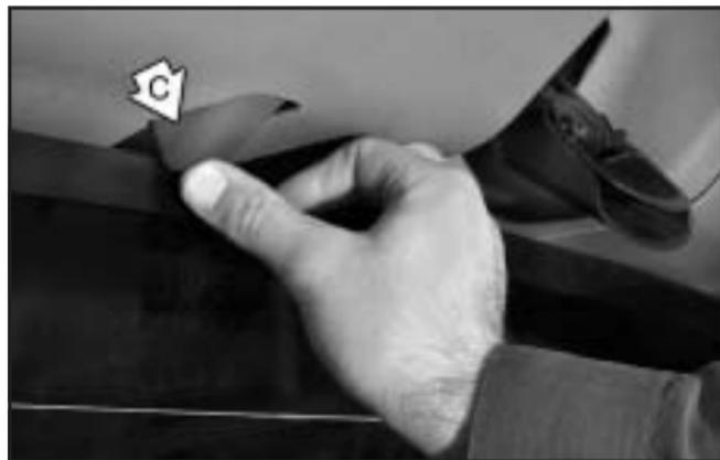
3. While holding the rear glass in place, press the glass-catch release button (C) and pull the top of the rear glass toward you using the grab handle(s) (B) located at the top of the rear glass.
