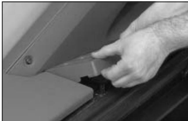
2. Grasp the edges of the grate and pull it out from the vehicle. Flush the drain with clean water.
