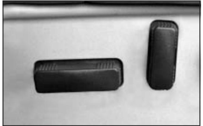
If your vehicle has power seat(s), the controls are located on the outboard edge of the front seats.
