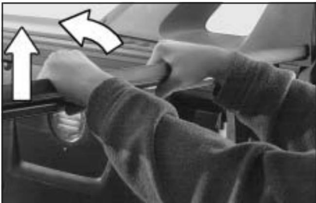
4. Remove the front rail by first twisting up the edge nearest you, to clear the midgate seals, and then pulling it out from the side rails.
