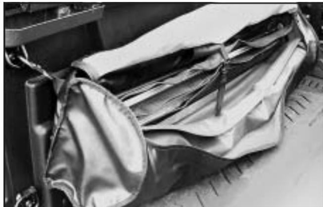
5. Stow both bows and the front and rear rails in the storage bag. When all components of the tonneau cover are secured in the bag properly, zip the bag shut.
