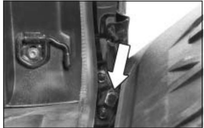
3. Raise the tailgate at a slight upward angle, pull back on the tailgate at the right edge so it releases from the block hinge and then move the tailgate to the right to release the left edge.
