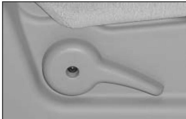
If you have manual reclining seatbacks, the lever is located on the outboard side of the seat cushion. To adjust the front seatback, lift the lever. Release the lever to lock the seatback where you want it. Lift the lever without pushing on the seatback and the seatback will go to an upright position.
