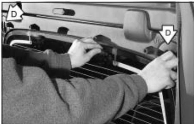
6. Turn both glass lock knobs (D), located at both top corners of the storage pocket, to the locked position. Push in on the corner of the rear glass to allow the lock knob to engage more easily.
