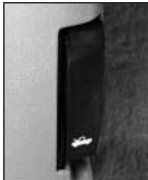
1. Pull the handle located inside the vehicle to the lower left of the steering wheel.
