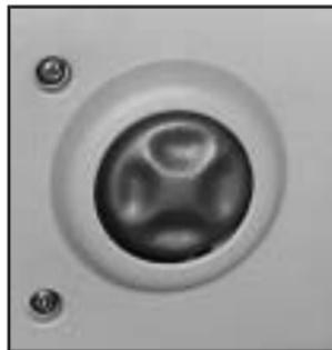
If your vehicle has power lumbar adjustment, you can use it to increase or decrease lumbar support in the lower seatback. The control is located on the outboard side of the seat cushion.
