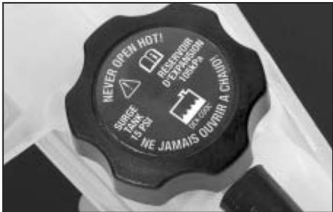
1. You can remove the coolant surge tank pressure cap when the cooling system, including the coolant surge tank pressure cap and upper radiator hose, is no longer hot. Turn the pressure cap slowly counterclockwise (left) about one full turn.
