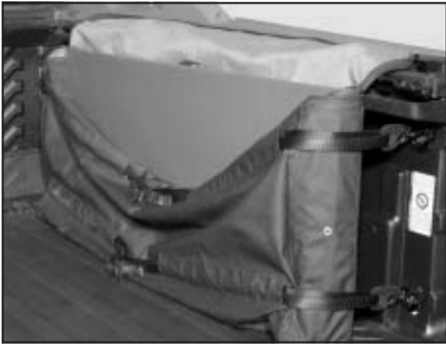
2. Starting with cargo panel 1, load the cargo panel with latches at the top of the bag and facing away from you.
