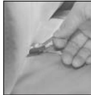
2. Pull the seat loop located where the seatback and seat cushion meet. The seat cushion will release and allow you to tilt it toward the front of the vehicle.
