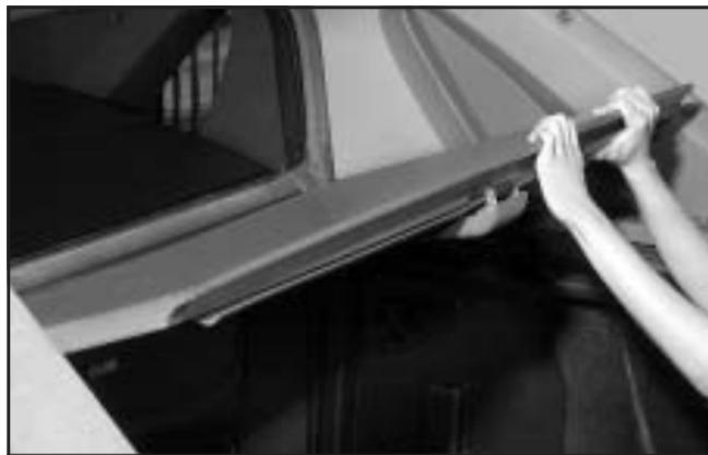
7. Close both top and bottom lever locks at the center of the bag to secure tightly.
