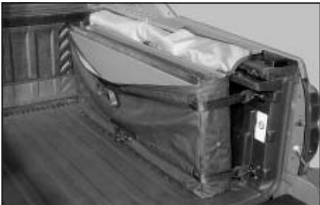
4. Store cargo panel 3 by loading the cargo panel with latches at the top of the bag and facing toward you.
