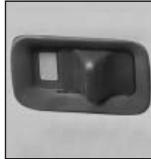
To unlock or lock the door from the inside, slide the manual lever forward or rearward.
