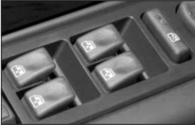
The controls for the power windows are located on the armrest on each of the side doors. The switches operate the windows when the ignition is in RUN, ACCESSORY or while Retained Accessory Power (RAP) is active. See *Retained Accessory Power (RAP)* on page 2-29.
