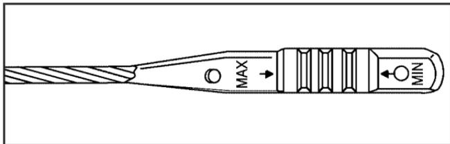
If the oil is at or below the MIN mark, then you will need to add at least one quart of oil. But you must use the right kind. This section explains what kind of oil to use. For engine oil crankcase capacity, see *Capacities and Specifications on page 5-97*.
