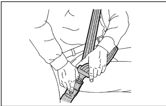
To unlash the belt, just push the button on the buckle. The belt should go back out of the way.
