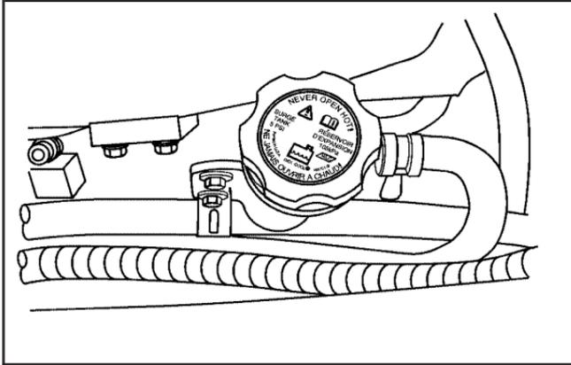
The intercooler system fill neck is located in the front of the engine compartment, near the center of the vehicle. See *Engine Compartment Overview on page 5-12* for more information on location.
