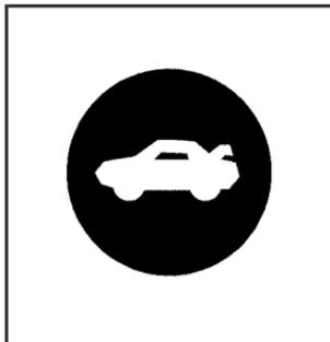
To open the trunk from inside the vehicle, press the remote trunk release button located inside the driver's storage compartment located on the lower left side of the instrument panel.
