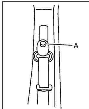
To move it down, push the release button (A) and move the height adjuster to the desired position. You can move the adjuster up just by pushing up on the shoulder belt guide.
