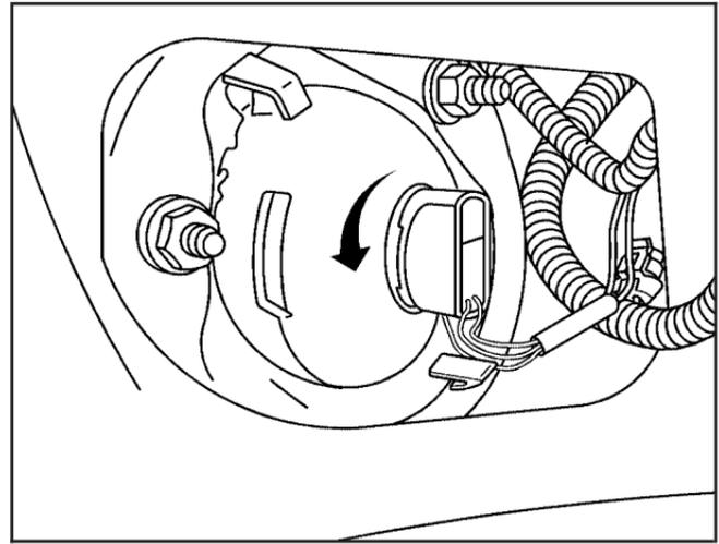
3. Remove the bulb socket by turning it counterclockwise.
