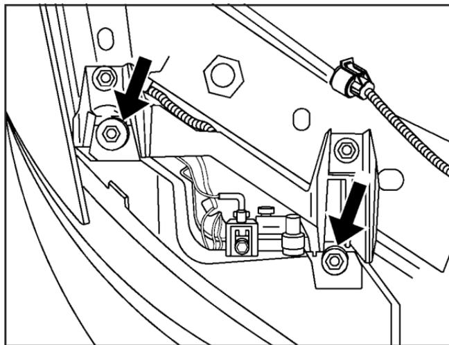
2. Remove the two wing bolts from the headlamp assembly.
