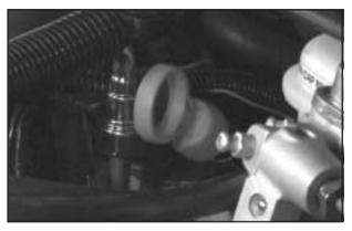
The automatic transaxle dipstick is located toward the back of the engine compartment, next to the brake master cylinder reservoir. The dipstick handle is a red loop. See *Engine Compartment Overview on page 5-12* for more information on location.
