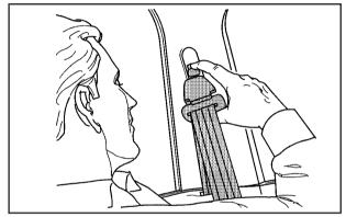
To move it down, push down on the button and move the height adjuster to the desired position. You can move the adjuster up just by pushing up on the shoulder belt guide. After you move the adjuster to where you want it, try to move it down without pushing the button down to make sure it has locked into position.
