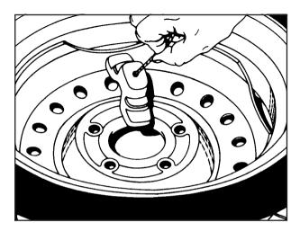
Tilt the retainer at the end of the cable to remove the compact spare tire from the cable, so it can be pulled up through the wheel opening. The hoist is used to store a full-size or a flat road tire under the vehicle. See *Storing a Flat or Spare Tire and Tools on page 5-80*.
