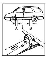
Near each wheel, there is a notch (A and B) in the vehicle's body. Position the jack and raise the jack head until it fits firmly into the notch in the vehicle's frame nearest the flat tire.
