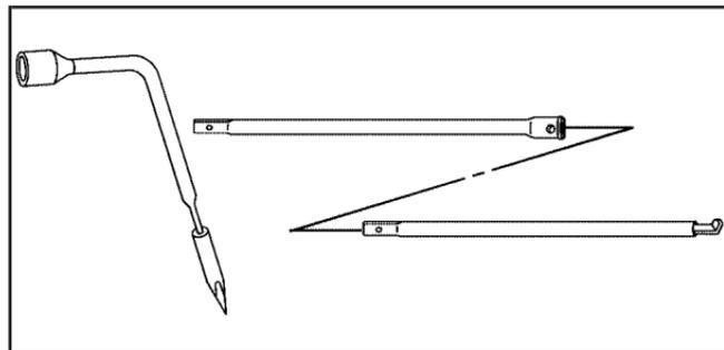
3. Attach the wheel wrench and extensions together.
