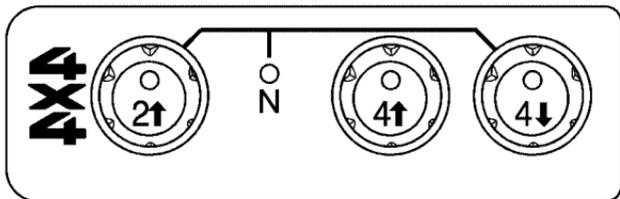
The transfer case buttons are located to the right of the steering wheel on the instrument panel.
