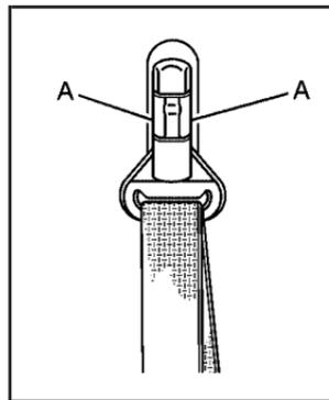
To move it up or down, squeeze the release buttons (A) together and move the height adjuster to the desired position. After you move the height adjuster to where you want it, try to move it down without squeezing the release buttons to make sure it has locked into position.
