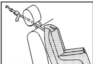
If the position you are using has an adjustable head restraint and you are using a single tether, route the tether under the head restraint and in between the head restraint posts.
