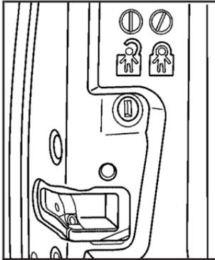
The rear door security lock is located on the inside edge of each rear door below the security lock label.
