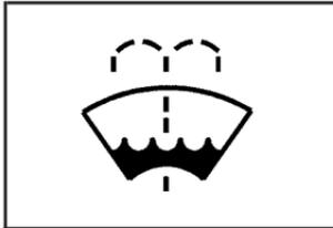
Open the cap with the washer symbol on it. Add washer fluid until the tank is full. See *Engine Compartment Overview* on page 5-12 for reservoir location.
