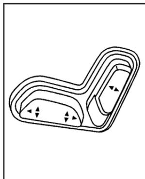
If your vehicle has power reclining seatbacks, use the vertical power seat control located on the outboard side of the seat.
