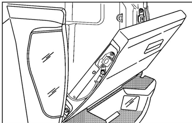
You can open the tailgate by pulling up on the outside handle while pulling the tailgate down.
