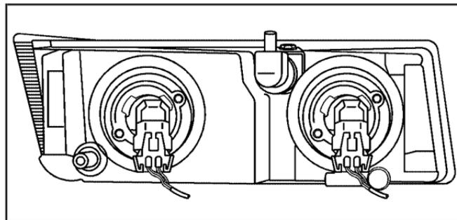
3. Turn the bulb socket counterclockwise and pull it straight out of the headlamp assembly.
