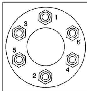
11. Tighten the wheel nuts firmly in a crisscross sequence as shown by turning the wheel wrench clockwise.
