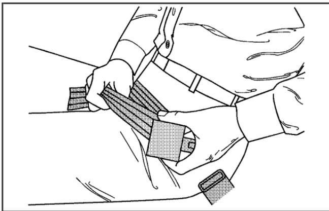
When you sit in the center front seating position, you have a lap safety belt, which has no retractor. To make the belt longer, tilt the latch plate and pull it along the belt.
