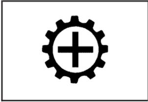
This light appears when you need to shift to the next higher gear on a manual transmission vehicle.
