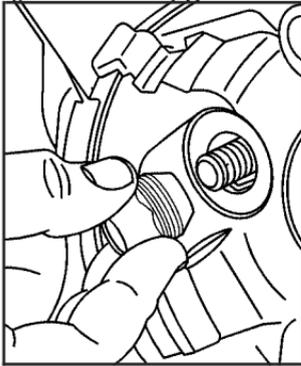
9. Put the wheel nuts back on with the rounded end of the nuts toward the wheel. Tighten each wheel nut by hand. Then use the wheel wrench to tighten the nuts until the wheel is held against the hub.
