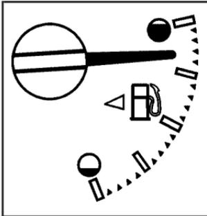
When the ignition is on, the fuel gage tells you about how much fuel you have remaining in the fuel tank.
