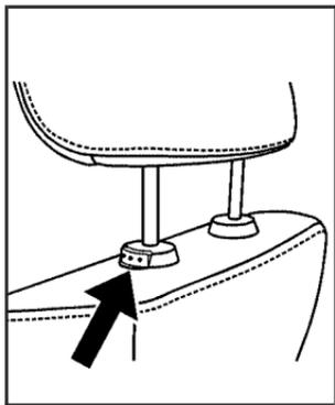
Pull up on the head restraint to raise it. To lower the head restraint, press the button located on top of the seatback and push down on the head restraint.
