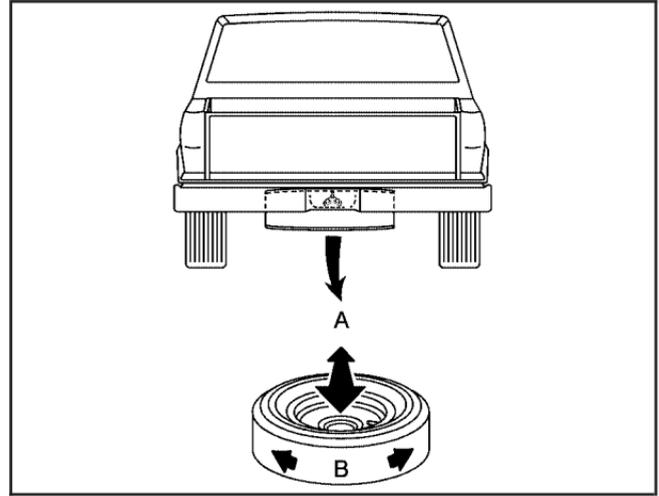
7. Make sure the tire is stored securely. Push, pull (A), and then try to turn (B) the tire. If the tire moves, check to make sure the tire valve stem is pointing down, then use the wheel wrench to loosen and then tighten the cable.
