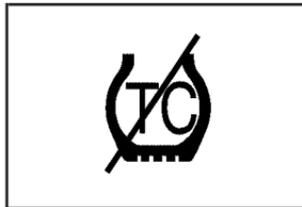
The TCS button is located on your instrument panel. Press this button to turn the TCS off and on.
