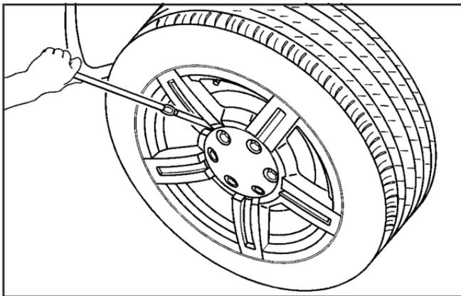
1. Remove the center cap by placing the chisel end of the wheel wrench (E) into one of the slots on the wheel and gently prying the cap out.
