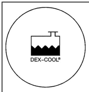
The coolant recovery tank cap has this symbol on it. It is located toward the rear of the engine compartment on the passenger's side of the vehicle. See *Engine Compartment Overview* on page 5-12 for more information on location.
