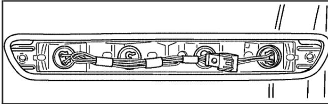
2. Turn the bulb socket counterclockwise and remove it from the housing.
