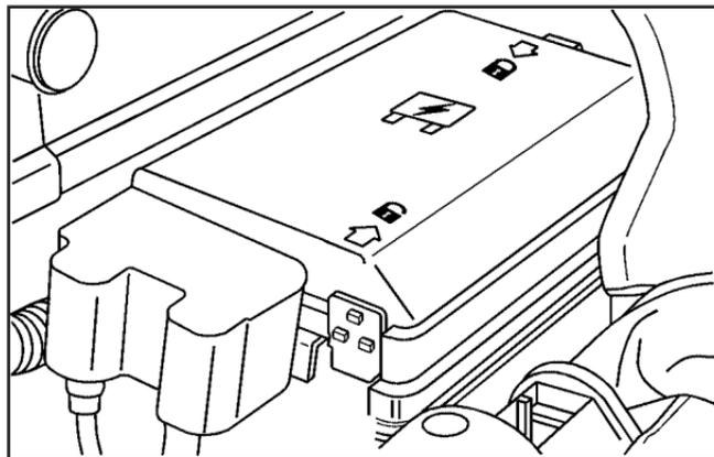
The engine compartment fuse block is located on the driver's side of the engine compartment. See *Engine Compartment Overview* on page 5-12 for more information on location.
