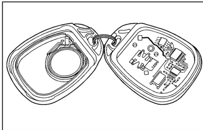
1. Insert a thin coin, or similar object, in the slot between the covers of the transmitter housing. Gently pry the transmitter apart.
