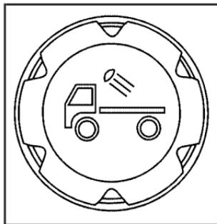
Press this button, located on the driver side of the instrument panel near the exterior lamp control to turn the cargo lamps on and off. You must have your dome lamps on for your cargo lamps to come on. See *Dome Lamp* on page 3-17.
