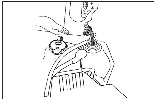
1. You can remove the radiator pressure cap when the cooling system, including the upper radiator hose, is no longer hot. Turn the pressure cap slowly counterclockwise about one full turn.
