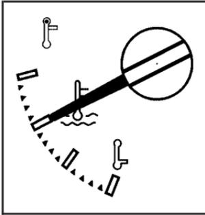
This gage shows the engine coolant temperature.
