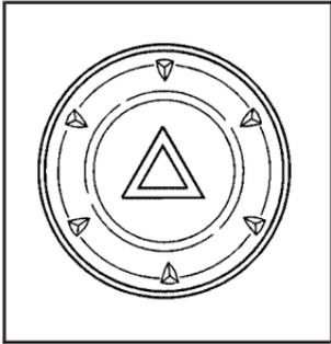
The hazard warning flasher button is located on the instrument panel, between the two air vents in the center.
