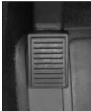
The parking brake pedal is located to the left of the regular brake pedal, near the driver's door.
