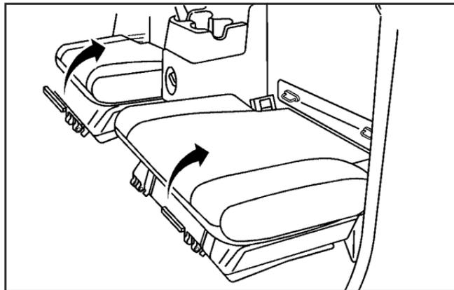
To access the storage compartments you will need to lift the cushion on the bottom of the rear seats. This will expose the storage boxes under the seat.
