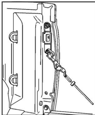
Remove the retaining cables from both sides of the tailgate by pulling the clips away from the bolt heads while pushing the cable bracket forward. When the larger part of the hole on the bracket is over the bolt, slide the bracket off of the bolt.
