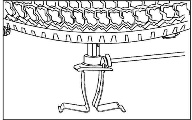
8. Attach the jack handle, extension, and wheel wrench to the jack and place it (with the wheel blocks) under the vehicle towards the front of the rear bumper. Position the center lift point of the jack under the wheel.
