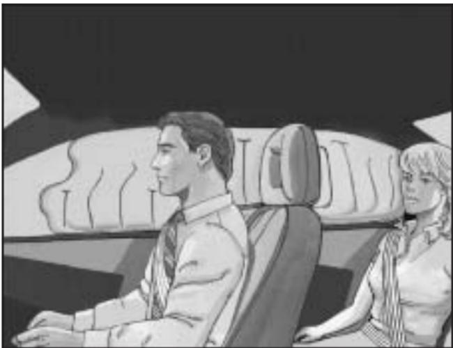
If your vehicle has a roof-mounted side impact airbag for the right front passenger and the person seated directly behind that passenger, it is located in the ceiling above the side windows.
