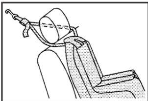
If the position you are using has a fixed or adjustable head restraint and you are using a dual tether, route the tether around the head restraint.
