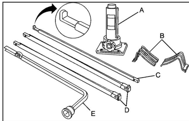
The tools you will be using include the jack (A), the wheel blocks (B), the extension tool (C), the jack handle extensions (D), and the wheel wrench (E).
