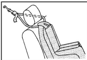
If the position you are using has a fixed or adjustable head restraint and you are using a dual tether, route the tether around the head restraint.
