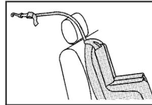
If the position you are using has a fixed head restraint and you are using a single tether, route the tether over the head restraint.
