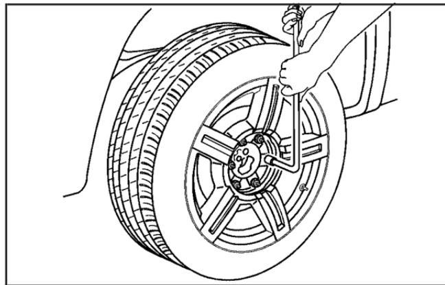
2. Use the wheel wrench to loosen all the wheel nuts by turning it counterclockwise. Do not remove the wheel nuts yet.
