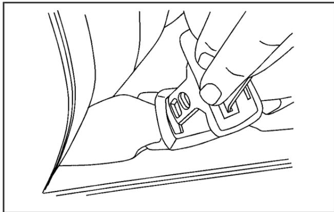
1. Disconnect the rear center safety belt latch from the mini buckle by inserting the tip of the safety belt tongue into the slot on the buckle. Let the belt retract.
