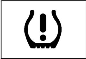
This light should come on briefly as you start the engine. It will then come on only when a flat or low tire pressure condition exists.
