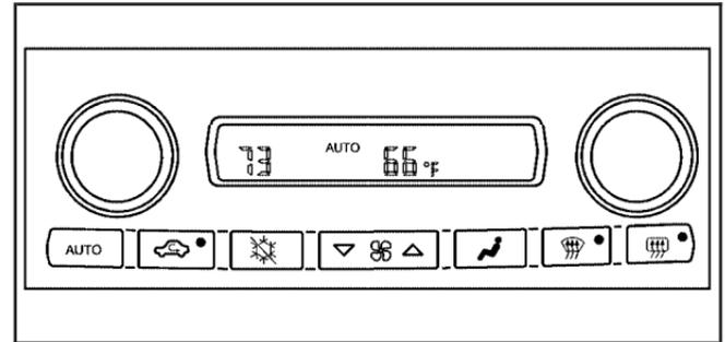
When your vehicle is first started, the display will show the driver's temperature setting, the outside temperature, the fan speed and the air delivery, for about 10 seconds.
