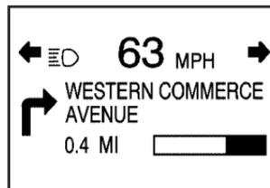
If your vehicle is equipped with a navigation radio, many of the turn-by-turn navigation features will also be displayed on the HUD if you are in Street Mode.
