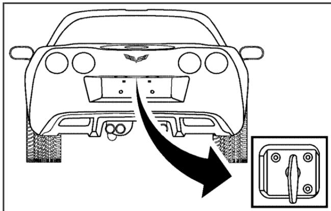
If your vehicle has lost battery power, open the hatch/trunk using the vehicle key. The key lock cylinder is located on the rear of the hatch/trunk lid above the license plate. Turn the vehicle key clockwise in the lock.
