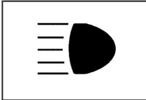
While the high beams are on, this light on the instrument panel cluster also will be on. To change the headlamps from high to low, pull the lever rearward.
