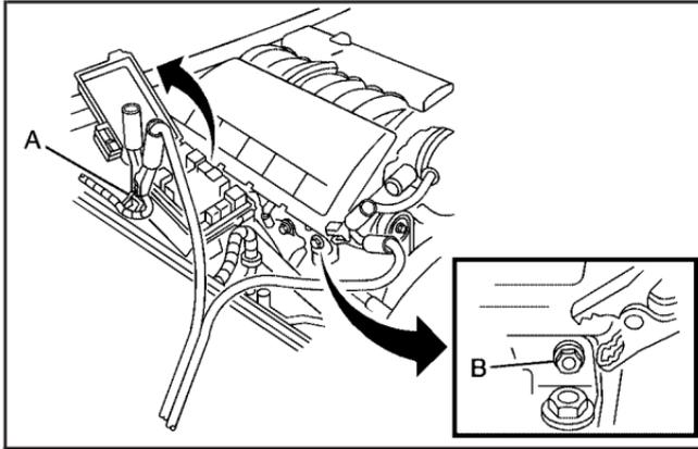
Your vehicle has a remote positive (+) terminal (A) and a remote negative (-) terminal (B), as shown in the illustration, which should be used to jump start your vehicle.
