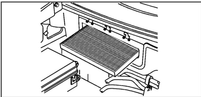
3. Remove the passenger compartment air filter from the housing.
