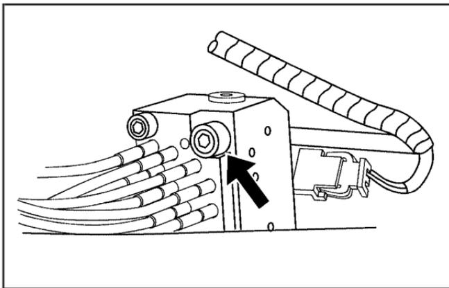
3. Locate the pressure release bolt on the front side of the hydraulic pump.
