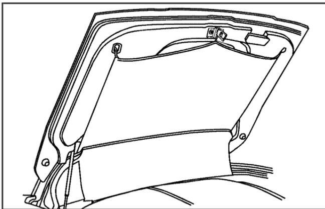
3. Grasp the loop at the rear center of the shade and wrap around the striker assembly.
