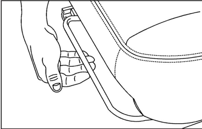
To move a manual passenger seat, pull up the bar located under the front of the seat to unlock it. Slide the seat to where you want it and release the bar. Then try to move the seat with your body to make sure it is locked into place.
