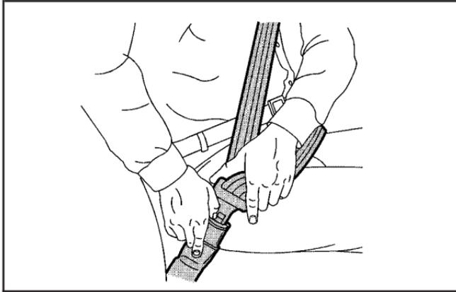
To unfasten the belt, just push the button on the buckle. The belt should go back out of the way.
