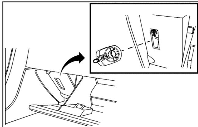
2. Place the new, unrecognized transmitter in the glove box transmitter pocket with the buttons facing towards the passenger's side.
