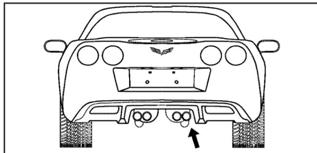
The rear lifting points can be accessed from the rear of the vehicle, on either the driver's or passenger's side.
