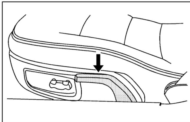
The lever for the reclining seatback is located on the outboard side of each seat.
