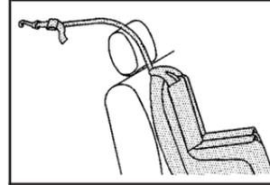
If the position you are using has a fixed head restraint and you are using a single tether, route the tether over the head restraint.
