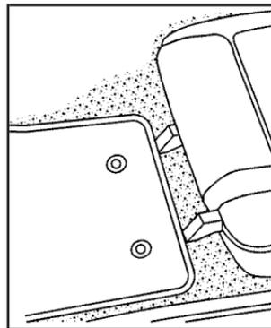
To remove the floor mats, pull up on the rear of the mat to disconnect from the locator pins.
