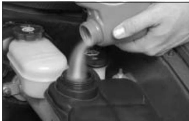
1. You can remove the coolant surge tank pressure cap when the cooling system, including the coolant surge tank pressure cap and upper radiator hose, is no longer hot. Turn the pressure cap slowly counterclockwise about one-quarter turn and then stop.
