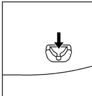
3. Gently place the roof panel down so that the back pins on the roof panel drop into the receivers in the back of the storage area. Press down firmly to seat the pins in the receivers.
