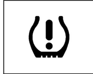
As an added safety feature, your vehicle has been equipped with a tire pressure monitoring system (TPMS) that illuminates a low tire pressure telltale when one or more of your tires is significantly under-inflated.
