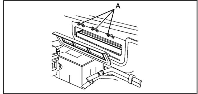
1. Disengage the passenger compartment air filter housing cover retainer clips (A).
