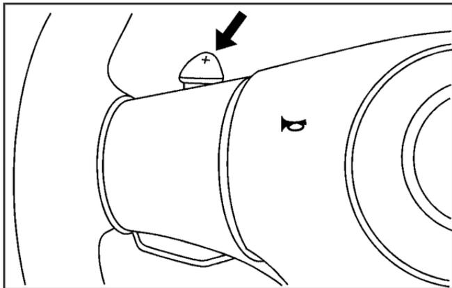
While in the SPORT MODE (S) mode, push the paddle above the steering wheel spokes to up-shift to the next gear, or pull on the paddle behind the steering wheel spokes to down-shift to the next gear.
