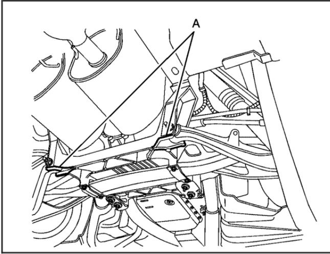
1. Locate the rear lifting points (A), according to the illustration shown.
