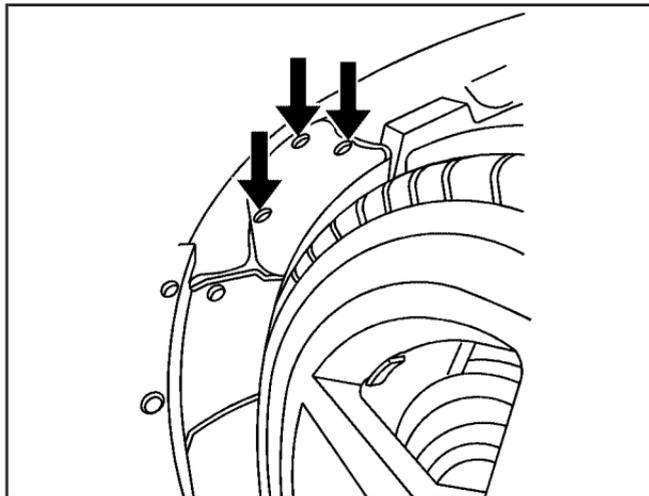
2. Access the high-beam or front parking/turn signal bulbs by removing the access panel. To do this, remove the three outer fasteners and flip back the cover.
