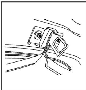
4. Push the loop to the top of the striker (base plate).
