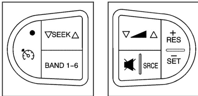
If your vehicle has this feature, some audio controls can be adjusted at the steering wheel.
