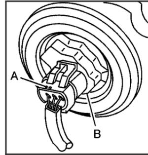
6. Press the clip (A) on the electrical connector when replacing the low-beam or high-beam bulb, then pull it straight off. Turn the bulb retaining ring (B) counterclockwise to remove it and then pull the bulb assembly straight out.
