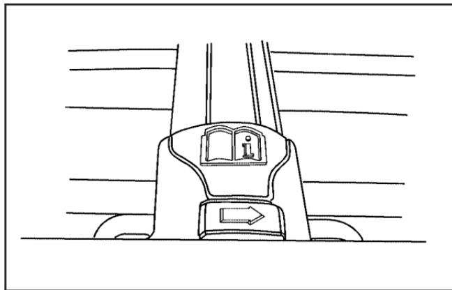
Press the lever down and align the crossrails on both sides with the holes on the siderails. Move the crossrail by hand. There will be a notable click as the pins align into the holes locking the crossrail into place.
