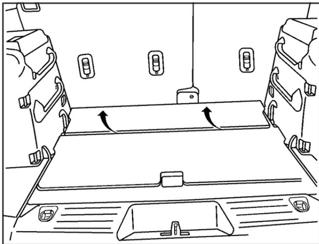
There is a flip panel towards the front of the cargo cover. You may have to flip this panel upward in order to gain access to the cargo cover.
