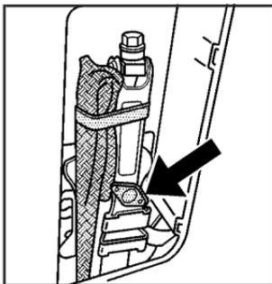
5. Remove the wing-bolt on the jack and then remove it.
