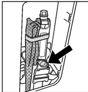
3. Install the jack in the left side panel of cargo area and secure with the wing bolt.
