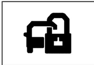
This light will come on for the theft-deterrent system and is located on the instrument panel cluster.
