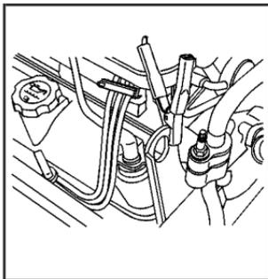
The remote negative (-) terminal is located in the front of the engine compartment, near the engine oil dipstick.
