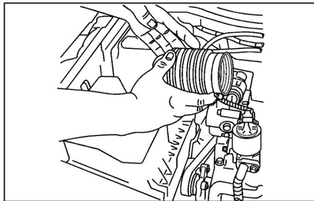
5. Remove the air outlet duct.
