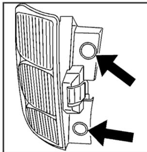
2. Remove the taillamp screw covers and then remove the two screws.
