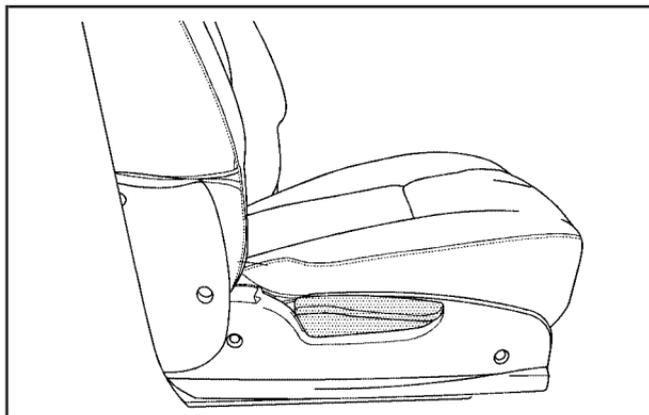
3. Lift the recliner lever, located on the outboard side of the seat, up fully and fold the seatback forward until it disengages.
