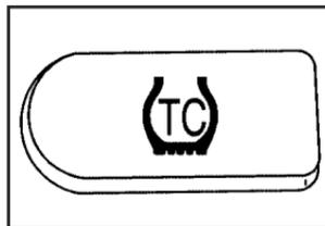
The traction control system can be turned off by pressing the traction control button, located on the instrument panel above the audio system.
