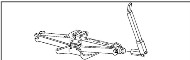
4. Attach the wheel wrench to the jack bolt head and rotate the wheel wrench clockwise. That will raise the lift head a little.
