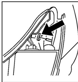
3. Carefully slide the taillamp assembly outward to clear the stud (see arrow) and then rearward and away from the body of the vehicle.
