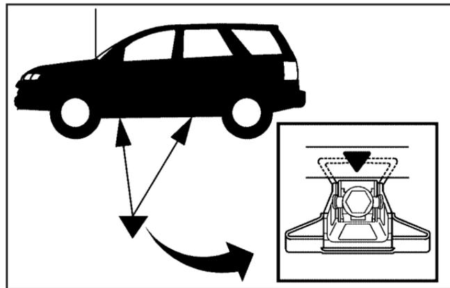
6. Find the arrow on the plastic lower body panel. Position the jack head under the metal jacking flange and not the plastic lower body panel.
