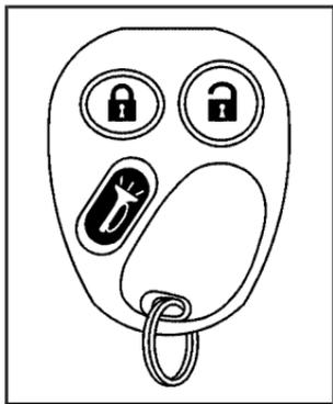
**🔒 (Lock):** Press this button on the remote keyless entry transmitter one time to lock the doors. The headlamps will flash once. This also arms the content theft-deterrent system.
