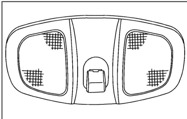
Your vehicle may have lamps located on the headliner above the rearview mirror. Push on the lens in the lamp to turn them on and off.
