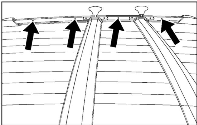
The roof rack crossrails can be locked in four positions only.
