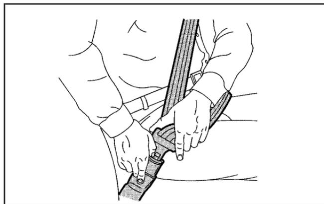
To unlatch the belt, just push the button on the buckle. For outboard seating positions, when the safety belt is not in use, slide the latch plate up the safety belt webbing. The latch plate should rest on the stitching on the safety belt, near the guide loop on the side wall.
