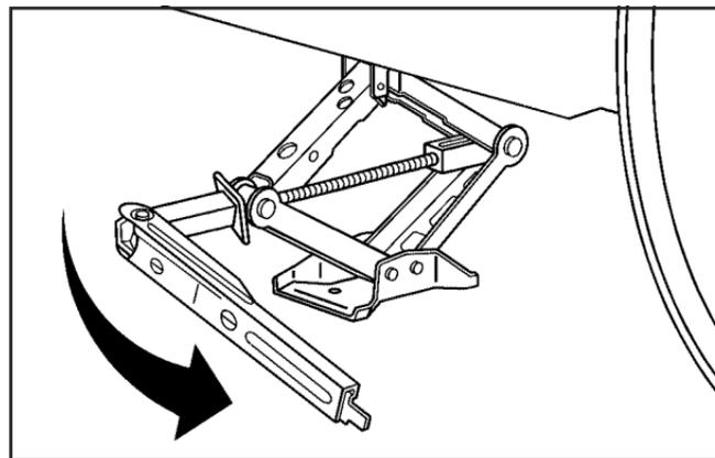
14. Lower the vehicle by turning the jack handle counterclockwise.
