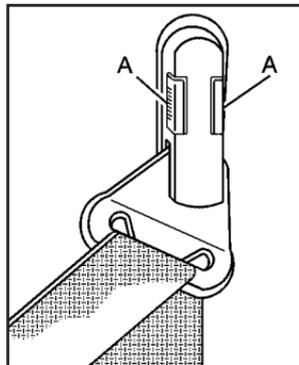
To move it up or down, squeeze the release buttons (A) together and move the height adjuster to the desired position. After you move the height adjuster to where you want it, try to move it up or down without squeezing the release buttons to make sure it has locked into position.
