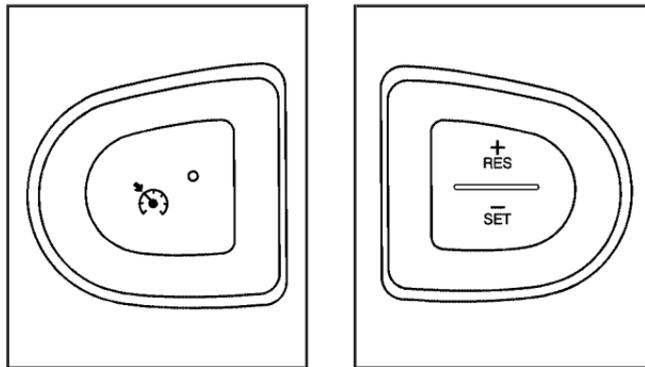
If your vehicle has cruise control, the buttons for the cruise control are located on the steering wheel.
