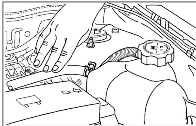
3. Fill the coolant surge tank with the proper DEX-COOL<sup>®</sup> coolant mixture, to the COLD FILL line.
