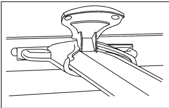
To reposition the crossrail, pull up on the end levers of the crossrail to the upright position. This will release the pins from the holes in the siderail. You will be able to move the crossrail into a new position.
