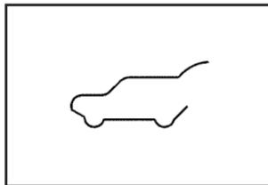
If this light comes on, your liftgate is not completely closed. Driving with the liftgate open can cause carbon monoxide (CO) to enter the vehicle.
