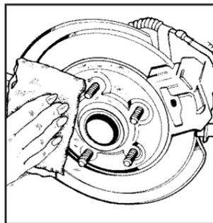
11. Remove any rust or dirt from the wheel bolts, mounting surfaces, and spare wheel.
