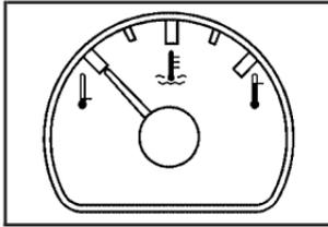
This gage measures the temperature of the vehicle's engine.
