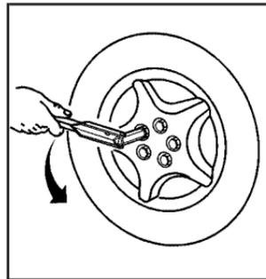
1. Loosen all five hex-shaped plastic caps by turning the wheel wrench counterclockwise. Do not try to remove plastic caps from the cover or center cap.
