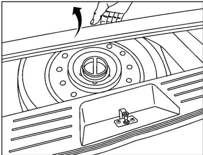
1. Lift the load floor up and pull it out of the vehicle and set it aside.
