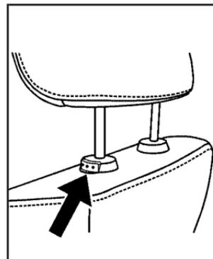
Press the button on the side of the head restraint to lower it.
