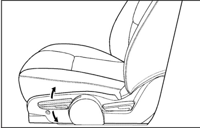
If your vehicle has a manual driver seat height adjuster, it is located on the outboard side of the seat near the front of the seat cushion. To raise the seat, move the lever upward repeatedly until the seat is at the desired height. To lower the seat, move the lever downward repeatedly until the seat is at the desired height.
