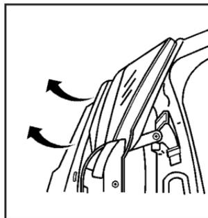
3. Gently pull the radiator cover/front grill toward you and pull the front grill trim bar away from the headlamp lens. The front grill bar is attached to the headlamp lens with a hidden clip.
