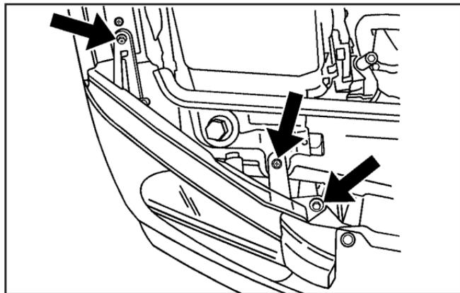
4. Remove the three headlamp assembly attachment screws.
