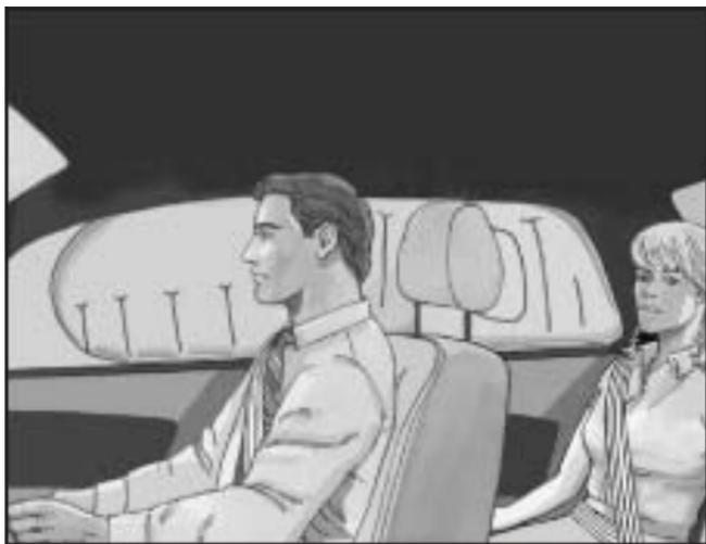
If your vehicle has a side impact airbag for the right front passenger and the person seated directly behind that passenger, it is in the ceiling above the side windows.
