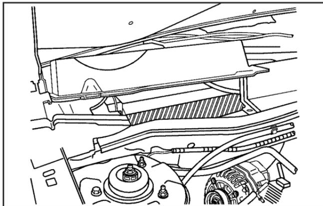
6. Remove the filter from the vehicle.
