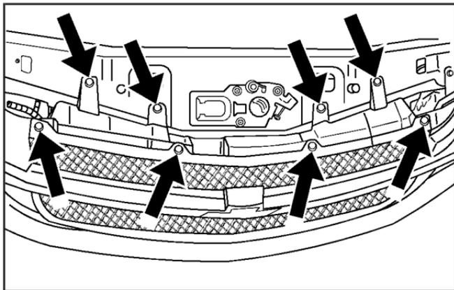
2. Remove the fastener plugs from the top of the radiator cover/front grill.
