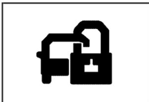
Your vehicle is equipped with a Passlock<sup>®</sup> theft-deterrent system. With this system, the security light will flash as you open the door if your ignition is off.
