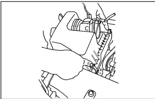
6. Undo the clamps on the filter cover. To remove the cover, pull up on the front and then pull the cover out.
