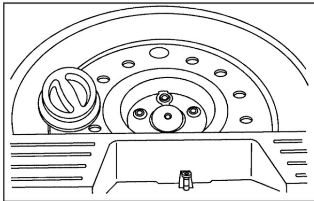
2. Remove the bolt retaining the spare tire.
