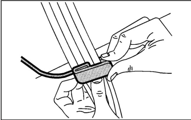
2. Slide the guide under and past the belt. The elastic cord must be under the belt.
