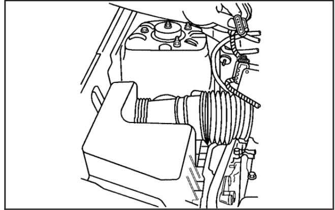
2. Disconnect the air flow sensor electrical connector.
