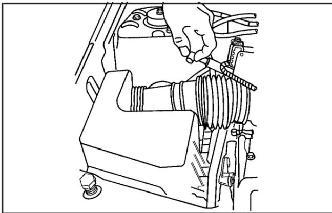
3. Disconnect the crank case ventilation tube.
