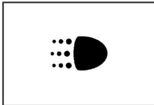
This light is located on the instrument panel cluster. It goes on whenever the Daytime Running Lamps are on.
