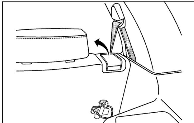
2. Lift the lever located on the top of the seatback to release the seatback.
