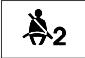
This light and chime reminder will be repeated if the passenger remains unbuckled and the vehicle is in motion.
