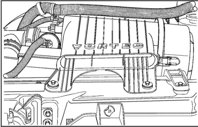
The engine air cleaner/filter is located near the center of the engine compartment. See *Engine Compartment Overview* on page 298 for more information on location.
