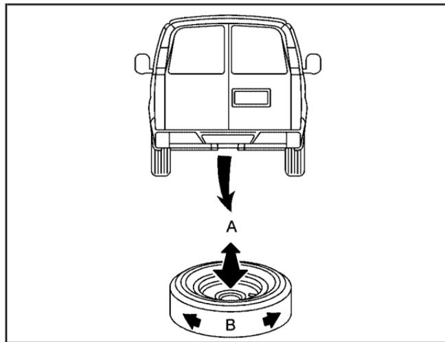
7. Make sure the tire is stored securely. Push, pull (A), and then try to turn (B) the tire. If the tire moves, use the ratchet to tighten the cable. You will hear two clicks when the tire is up all the way.
