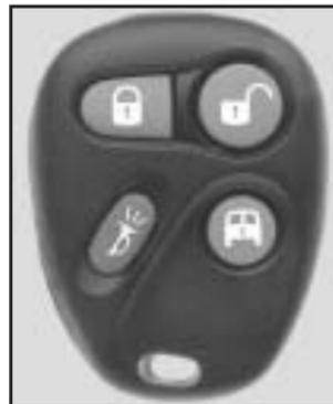
**🔒 (Lock):** Press this button once to lock all of the doors. The parking lamps will flash and the interior lamps will turn on briefly. Press the lock button again within five seconds and the parking lamps will flash and the horn will chirp briefly.
