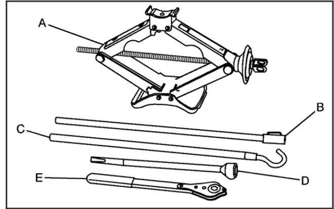
The tools you will be using include the jack (A), jack handle extension (B), jack handle (C), wheel wrench (D), and the ratchet (E).
