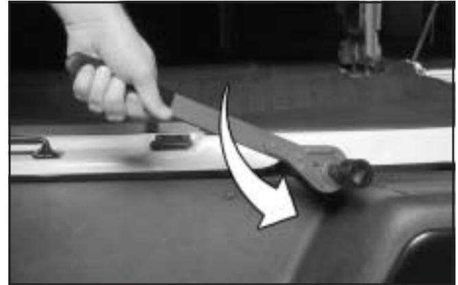
3. Turn the ratchet counterclockwise to lower the spare tire to the ground. If the spare tire does not lower to the ground, the secondary latch is engaged causing the tire not to lower. See *Secondary Latch System* on page 373.
