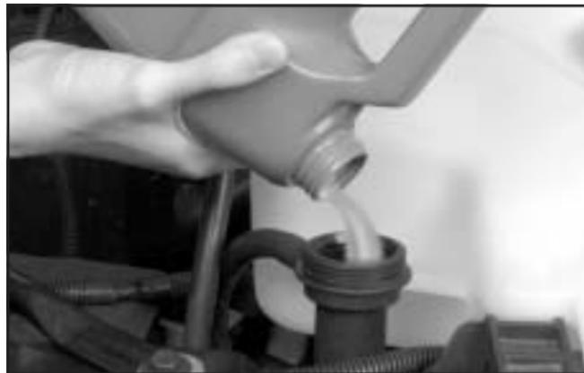
3. Fill the radiator with the proper DEX-COOL<sup>®</sup> coolant mixture, up to the base of the filler neck. See *Engine Coolant on page 308* for more information about the proper coolant mixture.
