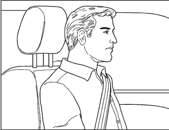
Adjust the head restraint so that the top of the restraint is at the same height as the top of the occupant's head. This position reduces the chance of a neck injury in a crash.
