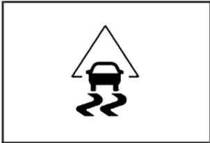
This light will flash when your traction control system is limiting wheel spin.
