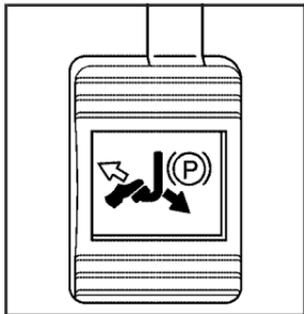
The parking brake is located to the left of the brake pedal, near the driver's door.
