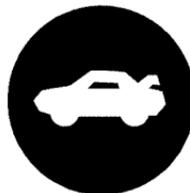
Press the remote release button, located on the lower edge of the driver's door, to open the trunk lid or the liftgate.
