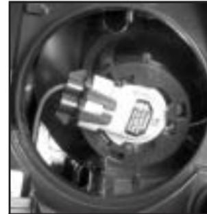
5. Disconnect the wiring harness, then turn the bulb socket counterclockwise to remove it.
