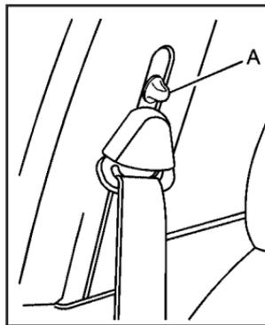
To move it down, push down the release button (A) and move the height adjuster to the desired position. You can move the height adjuster up by pushing the release button up.
