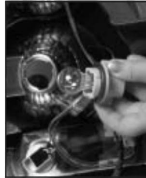
6. Pull the bulb to remove it from the socket. Replace the old bulb with a new one.
