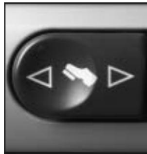
The switch used to adjust the pedals is located on the left side of the instrument panel.
