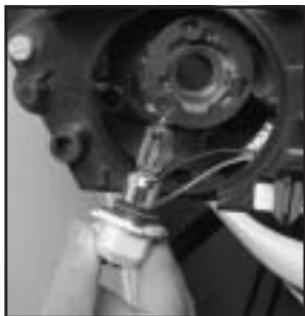
6. Remove the bulb from the bulb socket.
