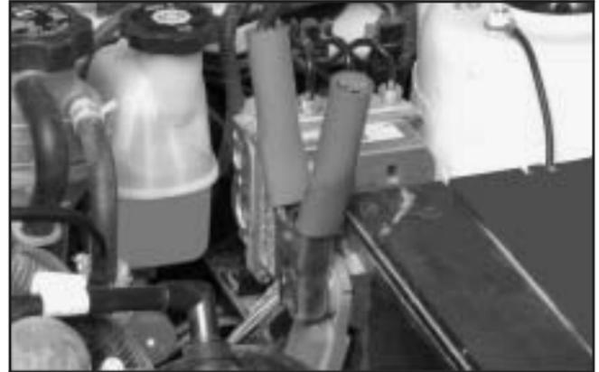
6. Connect the red positive (+) cable to the positive (+) terminal of the dead battery.
