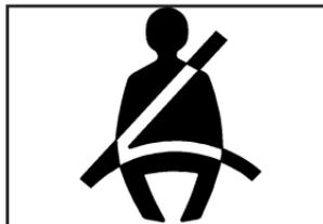
The safety belt light will come on and stay on until the driver's safety belt is buckled.
