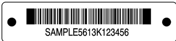
This is the legal identifier for your vehicle. It appears on a plate in the front corner of the instrument panel, on the driver side. You can see it if you look through the windshield from outside your vehicle. The VIN also appears on the Vehicle Certification and Service Parts labels and the certificates of title and registration.
