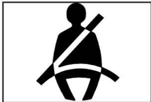
The safety belt light will come on when the engine is started and stay on until the driver's safety belt is buckled.
