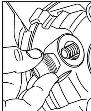
10. Put the wheel nuts back on with the rounded end of the nuts toward the wheel. Tighten each wheel nut by hand. Then use the wheel wrench to tighten the nuts until the wheel is held against the hub.
