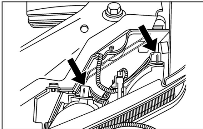
2. Reach in to access either one of the bulb sockets in the engine compartment.
