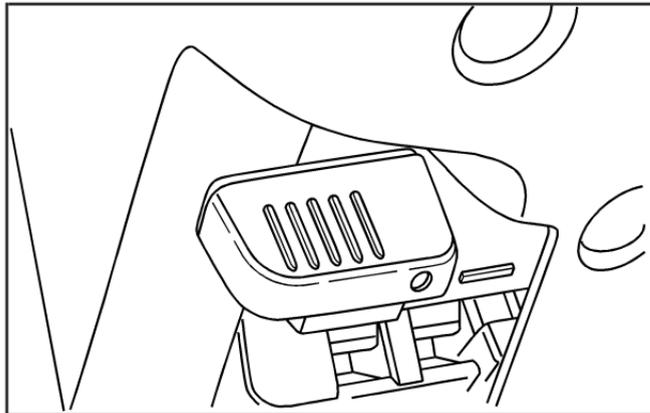
The tilt lever is located on the left side of the steering column, under the turn signal lever.
