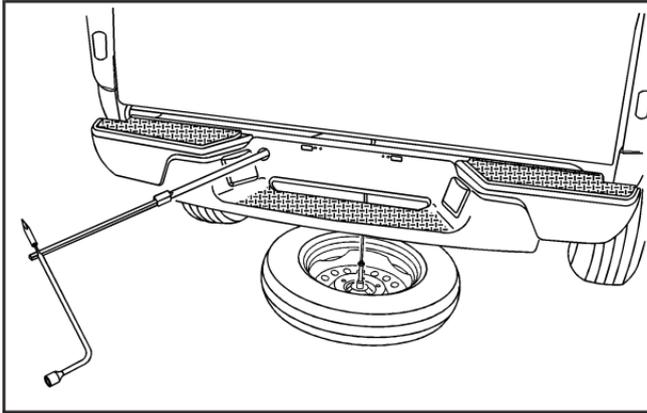
2. Insert the hoist end (chiseled end) of the extension tool (C) through the hole in the rear bumper and into the funnel-shaped guide. The chiseled end of the extension is used to lower the spare tire.
