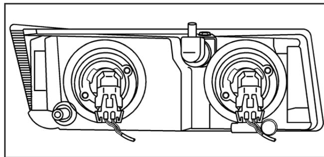
3. Turn the bulb socket counterclockwise to remove it from the headlamp assembly and pull it straight out.
