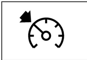
The cruise symbol on the instrument panel will be lit when the cruise control is engaged.
