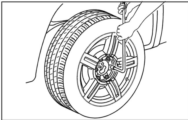
3. Use the wheel wrench to loosen all the wheel nuts by turning it counterclockwise. Do not remove the wheel nuts yet.
