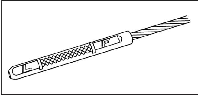
If the oil is below the cross-hatched area (L), add at least one quart/liter of the recommended oil. This section explains what kind of oil to use. For engine oil crankcase capacity, see *Capacities and Specifications* on page 5-120.
