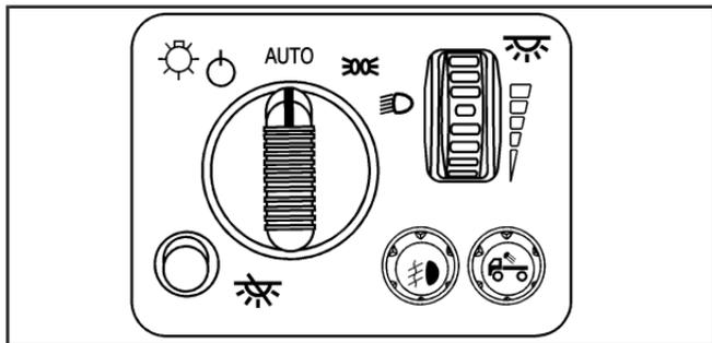
The control on the driver's side of the instrument panel operates the exterior lamps.
