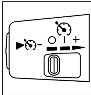
The cruise control set button is located at the end of the multifunction lever.
