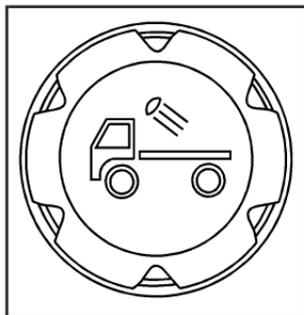
Press this button, located on the driver side of the instrument panel near the exterior lamp control, to turn the cargo lamps on and off.
