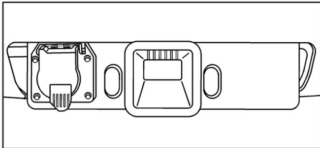
If your vehicle is equipped with a trailer towing package, the rear bumper harness will have a seven-pin universal heavy-duty trailer connector attached to a bracket on the hitch platform.
