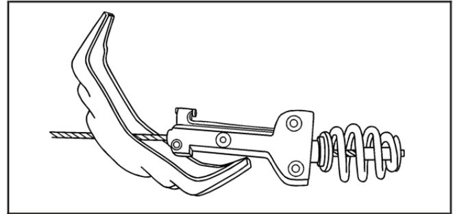
14. Tilt the tire retainer at the end of the cable and pull it through the wheel opening. Pull the tire out from under the vehicle.
