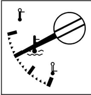
This gage shows the engine coolant temperature.
