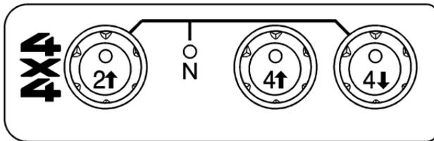
The transfer case buttons are located to the right of the steering wheel on the instrument panel.
