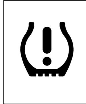
When a low tire pressure condition is detected, the TPMS illuminates the low tire pressure warning light located on the instrument panel cluster.
