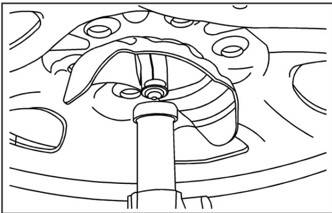
9. Position the center lift point of the jack under the center of the spare tire.
