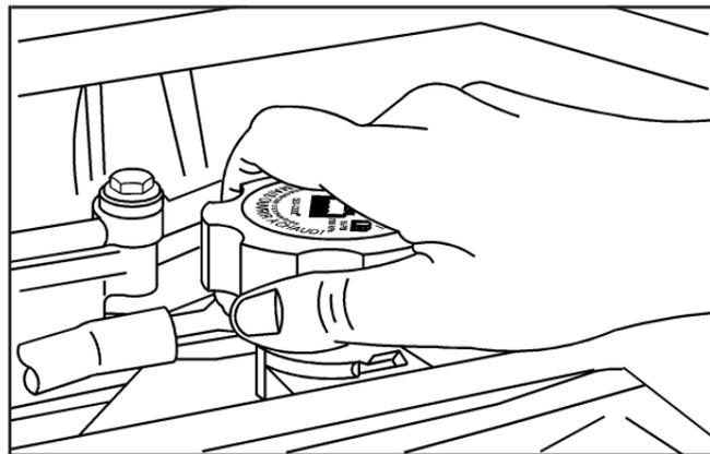
1. Remove the radiator pressure cap when the cooling system, including the upper radiator hose, is no longer hot. Turn the pressure cap slowly counterclockwise about one full turn.
