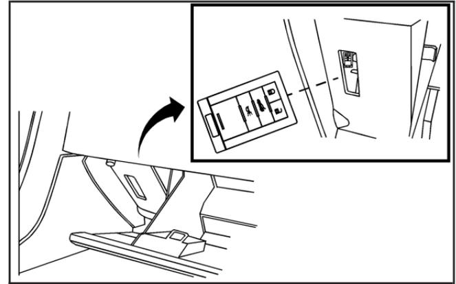
2. Place the new, unrecognized transmitter in the glove box transmitter pocket with the buttons facing towards the passenger side.
