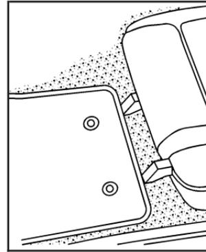
To remove a floor mat, pull up on the rear of the mat to disconnect it from the locator pins.
