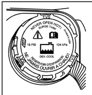
The engine coolant surge tank is located toward the rear of the engine compartment on the driver's side of the vehicle. See *Engine Compartment Overview on page 5-14* for more information on location.
