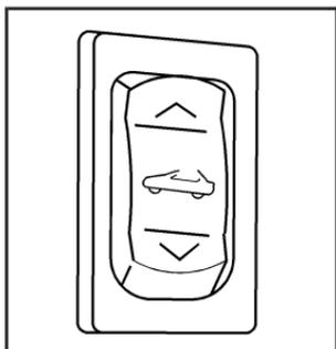
4. Push and hold the bottom of the power convertible top button, located to the left of the steering wheel, on the instrument panel.
