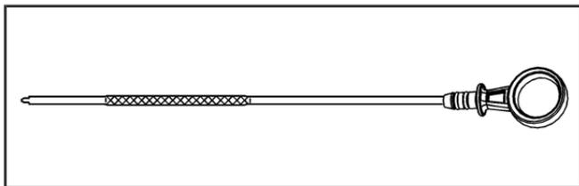
If the oil is below the cross-hatched area at the tip of the dipstick, add at least one quart/liter of the recommended oil through the oil fill cap opening in the oil tank. This section explains what kind of oil to use. For engine oil crankcase capacity, see *Capacities and Specifications on page 5-103*.
