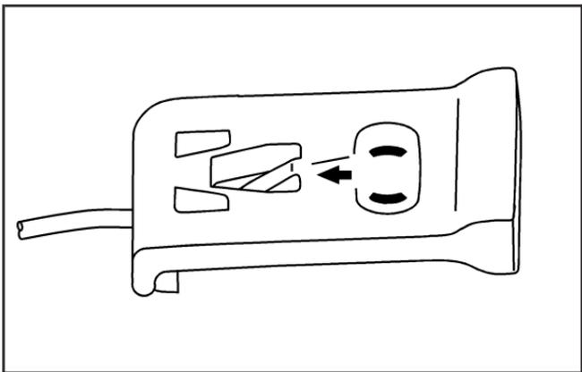
From outside the vehicle, use the key in the cylinder above the license plate to open the hatch then use the door release tab located on the carpet inside the trunk on the driver's side of the vehicle. Pull the tab to unlock and unlatch the driver's door. See *Keys on page 2-3* for information on opening the trunk during a loss of power.
