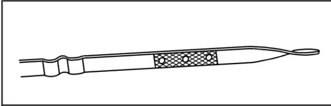
If the oil is below the cross-hatched area at the tip of the dipstick, add at least one quart/liter of the recommended oil. This section explains what kind of oil to use. For engine oil crankcase capacity, see *Capacities and Specifications on page 5-103*.
