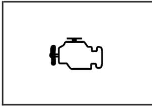
The check engine light comes on to indicate that there is an OBD II problem and service is required.
