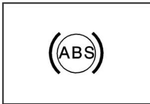
For vehicles with the Antilock Brake System (ABS), this light will come on briefly when you start the engine.
