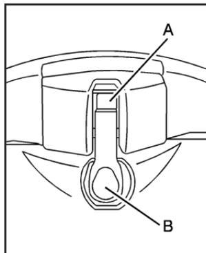
7. To unlock the rear of the roof panel's rear release latch, press the back of the release handle (B). Then press the button on the front of the release handle, (A) with your thumb.
