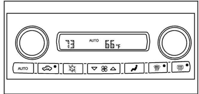
When the vehicle is first started, the display will show the driver's temperature setting, the outside temperature, the fan speed and the air delivery, for about 10 seconds.
