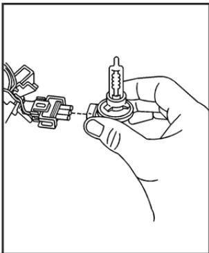
4. Remove the headlamp bulb by releasing the outer tabs from the socket.
