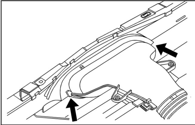
If you are cleaning your vehicle with the hood open, take care not to spray water directly near the filter opening of the air cleaner, as shown in the illustration, as this could damage your vehicle's engine.
