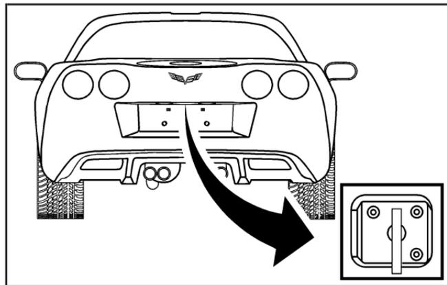
If your vehicle has lost battery power, open the hatch/trunk using the vehicle key. See *Keys* on page 2-3 for more information. The key lock cylinder is located on the rear of the hatch/trunk lid above the license plate. Turn the vehicle key clockwise in the lock.
