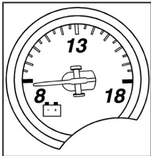
The voltmeter shows the voltage output of your battery. When the engine is running, it shows the voltage output of the charging system.
