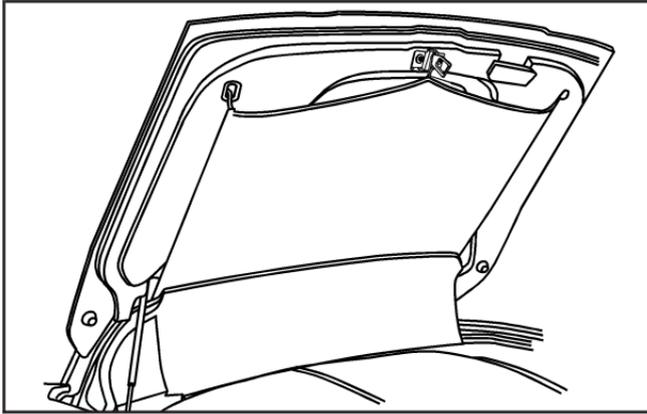
3. Grasp the loop at the rear center of the shade and wrap it around the striker assembly.
