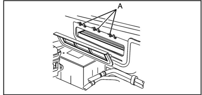
1. Undo the passenger compartment air filter housing cover retainer clips (A).
