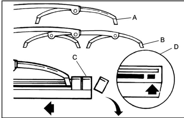
1. Slide the insert (D), notched end last, into the end with the two blade claws (A). Slide the insert all the way through the blade claws at the opposite end (B). Plastic caps (C) will be forced off as the insert is fully installed.
