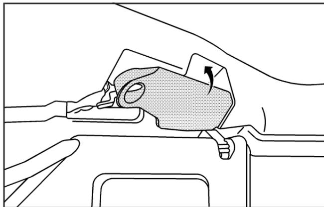
6. To unlock the release latches on the front of the roof panel, grasp each handle with your fingers and pull it outward.
