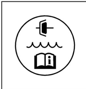
The hydraulic clutch fluid reservoir cap has this symbol on it. See *Engine Compartment Overview* on page 5-14 for reservoir location.
