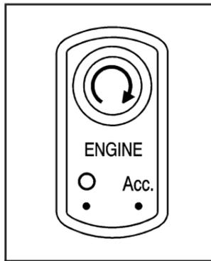
Your vehicle has an electronic keyless ignition with a pushbutton start.
