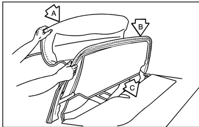
5. Lift upward on the front edge (A) of the convertible top off the windshield frame. Then lift upward on the rear edge (B) of the convertible top so it is vertical to the tonneau cover (C). The front edge (A) and rear edge (B) should be straight up.
