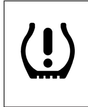
When a low tire pressure condition is detected, the TPMS illuminates the low tire pressure warning light, located in the instrument panel cluster.
