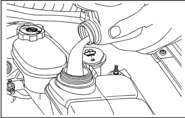
3. Fill the coolant surge tank with the proper mixture until the level inside stabilizes at the FULL COLD mark on the front of the surge tank.
