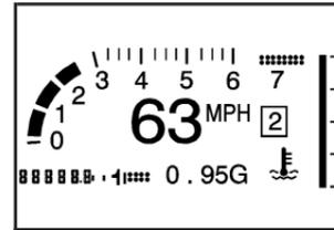
Track Mode 2 supports G-Force gages and minor gages with a linear tachometer.
