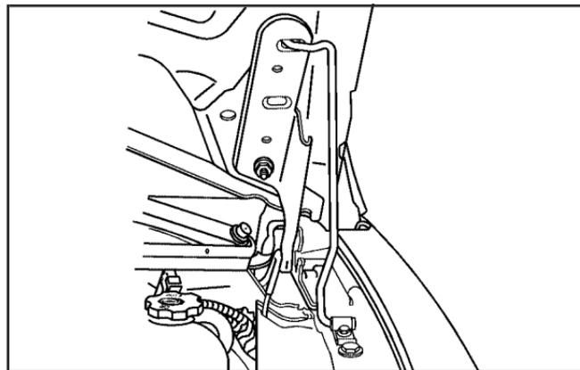
3. Lift the hood, release the hood prop from its retainer and put the hood prop into the slot in the hood.
