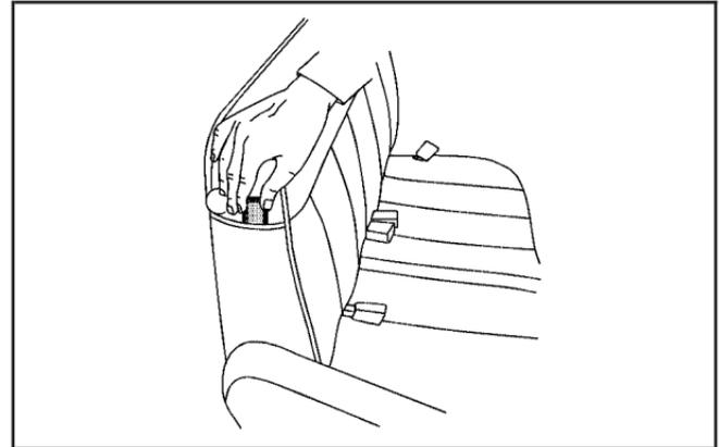
1. Locate the guide in a pocket on the side of the seatback.
