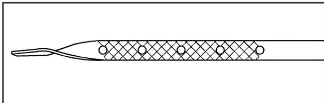
If the oil is below the cross-hatched area at the tip of the dipstick, add at least one quart/liter of the recommended oil. This section explains what kind of oil to use. For engine oil crankcase capacity, see *Capacities and Specifications on page 5-116*.
