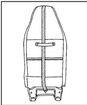
If the position you are using has an integrated headrest or head restraint and you are using a single tether, route the tether over the headrest or head restraint.
