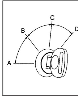
Use the key to turn the ignition switch to four different positions.
