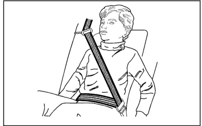
4. Buckle, position, and release the safety belt as described in previously in this section. Make sure that the shoulder belt crosses the shoulder.
