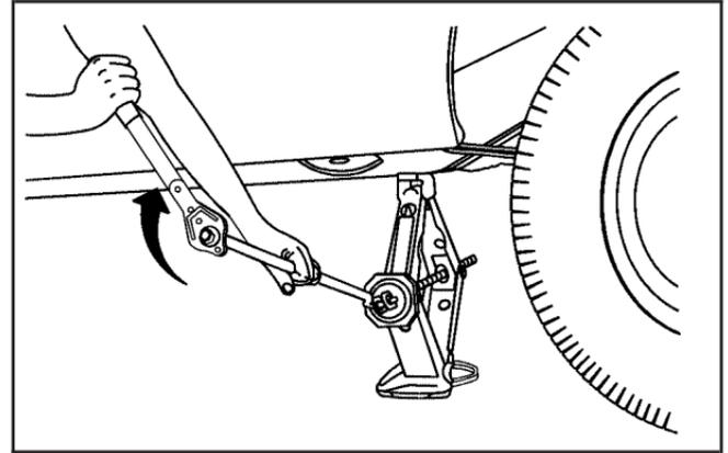
5. Raise the vehicle by turning the ratchet clockwise. Make sure the UP mark faces you. Raise the vehicle far enough off the ground so there is enough room for the spare tire to fit.
