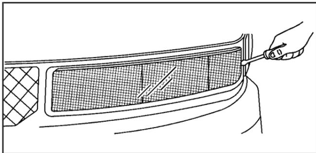
1. Use a small tool to unlatch the outboard clip on the lamp.
