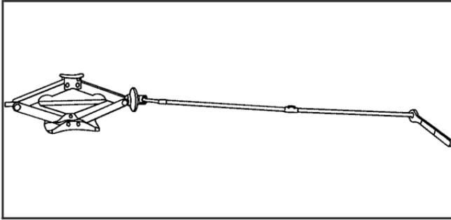
4. Attach the jack handle/jack handle extension to the jack. With the UP mark facing you, slide the ratchet onto the end of the jack handle extension.
