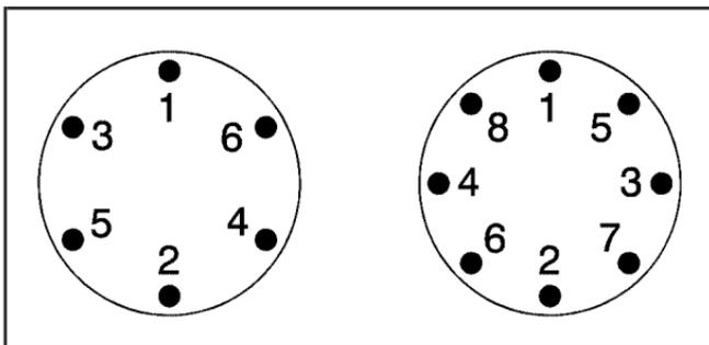
11. Use the wheel wrench to tighten the nuts firmly. Turn the wheel wrench clockwise and in a crisscross sequence as shown.
