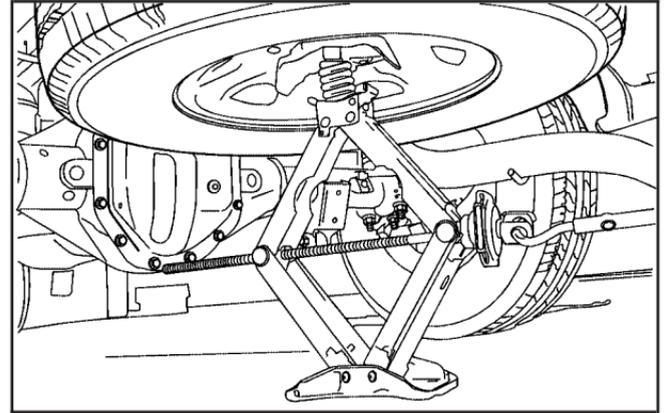
5. Place the jack under the vehicle, ahead of the rear bumper. Position the center lift point of the jack under the center of the spare tire and turn the handle clockwise to raise the jack until it lifts the secondary latch spring.
