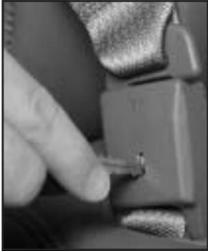
1. To do this, press the tip of a key into the release hole of the safety belt buckle while pulling up on the safety belt.
