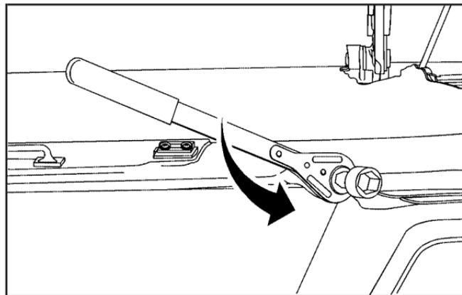
3. Turn the ratchet counterclockwise to lower the spare tire to the ground. If the spare tire does not lower to the ground, the secondary latch is engaged causing the tire not to lower. See *Secondary Latch System* on page 5-93.
