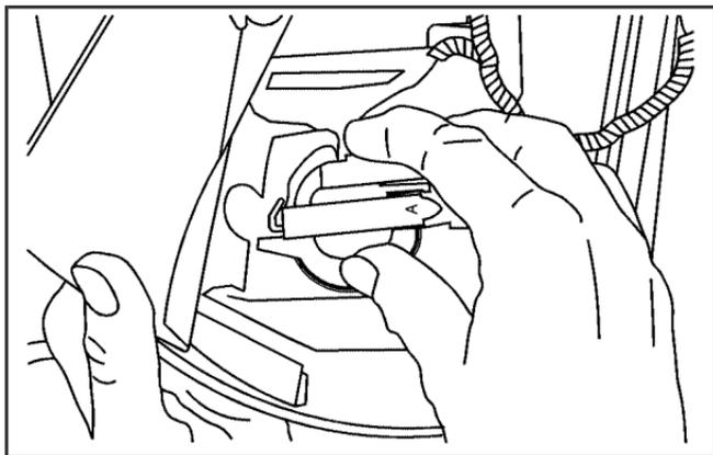
6. Remove the bulb socket by squeezing the tab on the side of the socket while turning it counterclockwise.
