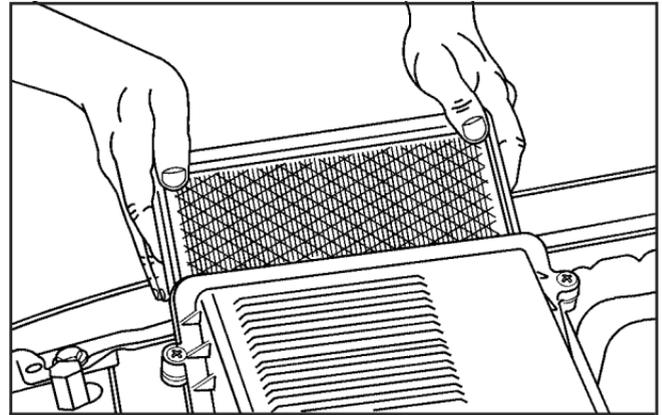
2. Loosen the four screws on the cover of the housing and lift up the cover.
