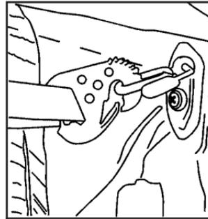
1. Secure the storage strap system in the cargo storage area by attaching the six clips included on the cargo strap system to the tie down locations on either side of the storage area.
