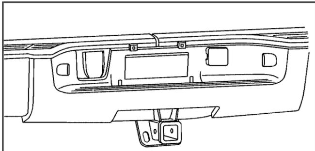
Your vehicle is equipped with the seven-wire trailer towing harness. This harness with a seven-pin universal heavy-duty trailer connector is attached to the rear bumper beam. It is located next to the integrated trailer hitch.
