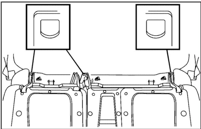
The top tether anchors are located on the back of the rear seat frame above the floor for each rear seating position. Fold down the rear seatback(s) to access the anchors. See *Rear Seat Operation* on page 1-13.
