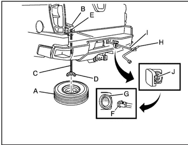
1. Put the tire (A) on the ground at the rear of the vehicle with the valve stem pointed down, and to the rear.
