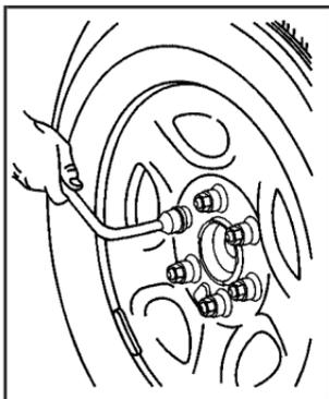
3. Use the wheel wrench to loosen all the wheel nuts. Turn the wheel wrench counterclockwise to loosen the wheel nuts. Do not remove the wheel nuts yet.
