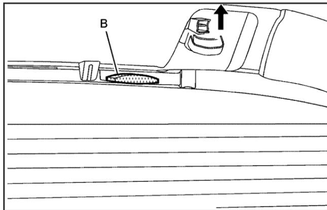
6. Push the rear glass flat against the window frame and push each latch lever up until it locks. You should hear a click when each latch lever locks correctly.
