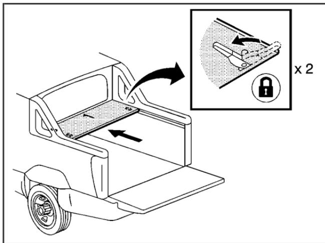
2. The driver side cargo cover panel latch must lock in place before the passenger side latch can be locked. If this procedure is not followed exactly, the cargo cover panels might not correctly lock in place. Push the driver side latch toward the front of the vehicle to lock the cover in position. A click sounds when each latch locks. Lock the remaining passenger side latch on panel 1.
