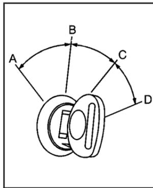
The ignition switch has four different positions.
