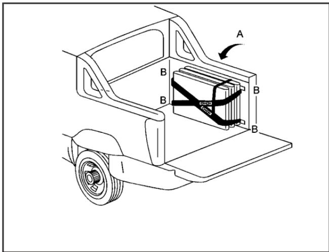
3. Place the primary straps over the three cargo covers (A). Fasten the four strap clips (B).
