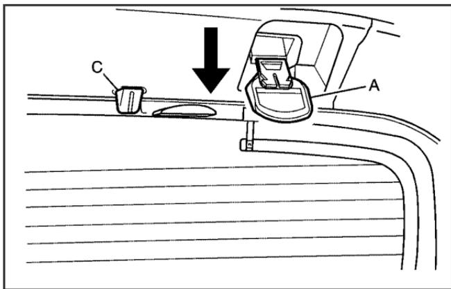
2. Squeeze and pull down the latch levers (A), located near the upper corners of the rear glass, to unlatch. Once unlatched, the glass-catch release button (C) will catch the rear glass and prevent it from falling forward.
