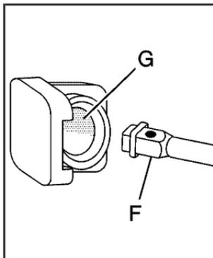
4. Insert the open end of the extension (F) through the hole in the rear bumper (G) (hoist shaft access hole).
