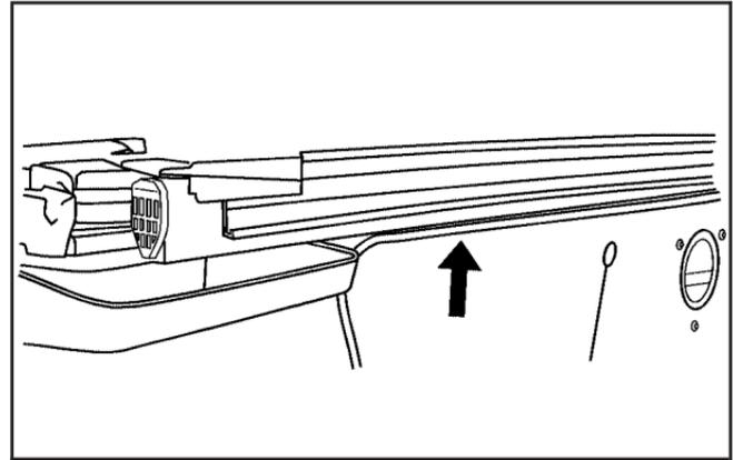
The side rail channels are located on top of both sides of the cargo area. Flush them out with clean water if debris collects inside of them.
