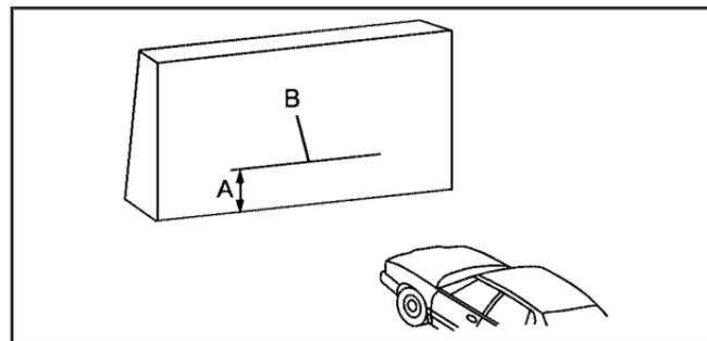
4. At a wall measure from the ground upward (A) to the recorded distance from Step 3 and mark it.
