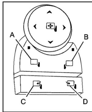
Vehicles with outside power foldaway mirrors have controls located on the driver door armrest.
