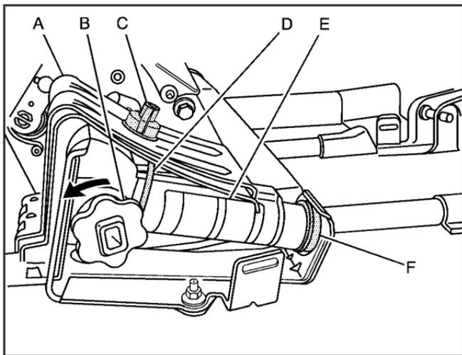
3. Remove the wheel blocks (A) attached to the jack (E) by turning the wing nut (C) counterclockwise. Place the wheel blocks where needed as indicated in previously in this section.
