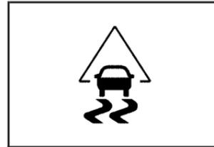
The StabiliTrak indicator light comes on briefly when the engine is started.
