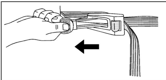
5. Close both cross locks at the center of the strap system to tightly secure.
