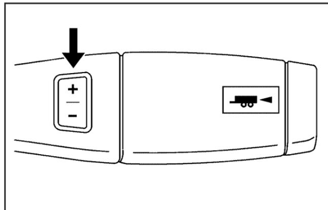
On vehicles with a Range Selection Mode, this feature may be used to control the vehicle's transmission.
