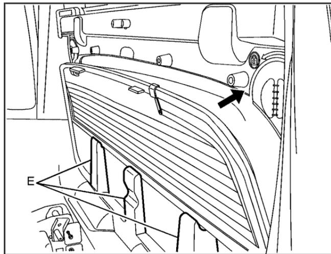
5. Load the rear glass into the storage pocket in the Midgate®, guiding the lower edge of the rear glass behind the three rear glass retaining tabs (E). Hold the rear glass flat against the storage pocket, with grab handles facing you, until the next step.
