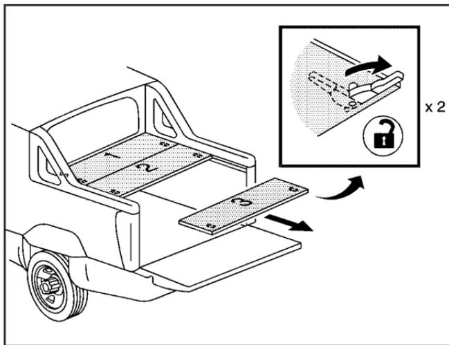
2. Unlock the cargo panel 3 by pulling forward on the driver side and passenger side cargo panel latches, located on the bottom of each cargo panel.
