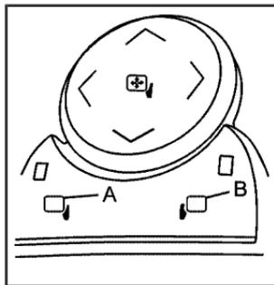
Vehicles with outside power mirrors have controls located on the driver door armrest.
