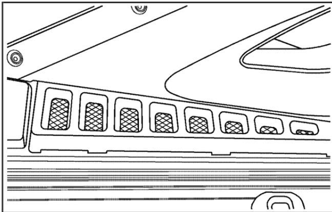
The top drain grates are located near the rear window on both sides of the vehicle. Clean the grates and drains if there is a blockage.
