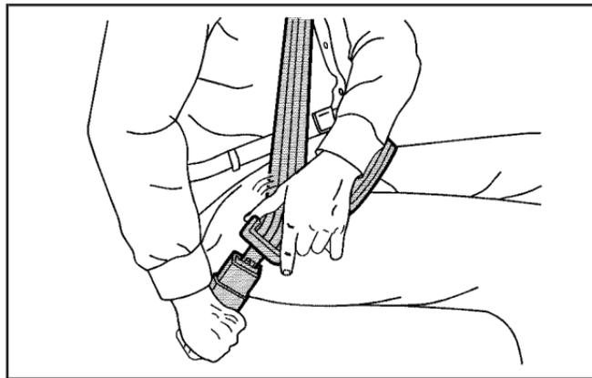
3. Push the latch plate into the buckle until it clicks. If you find that the latch plate will not go fully into the buckle, see if you are using the correct buckle. Pull up on the latch plate to make sure it is secure. If the belt is not long enough, see *Safety Belt Extender* on page 1-37. Position the release button on the buckle so that the safety belt could be quickly unbuckled if necessary.
