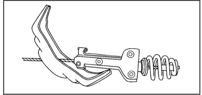
7. Tilt the tire with slack in the cable to access the tire/wheel retainer (D). Separate the retainer from the guide pin by sliding the retainer up the pin while pressing down on the latch. When the retainer is separated from the guide pin, tilt the retainer and pull it through the center of the wheel along with the cable and guide pin.
