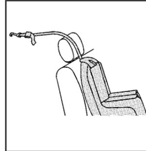
If the position you are using has a fixed headrest or head restraint and you are using a single tether, route the tether over the headrest or head restraint.
