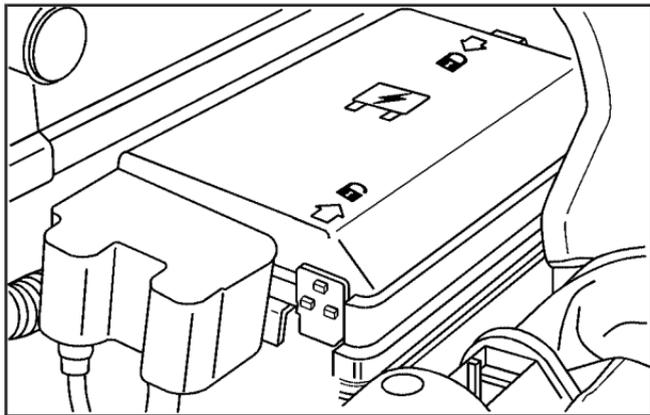
The engine compartment fuse block is located on the driver side of the engine compartment. See *Engine Compartment Overview* on page 5-12 for more information on location.
