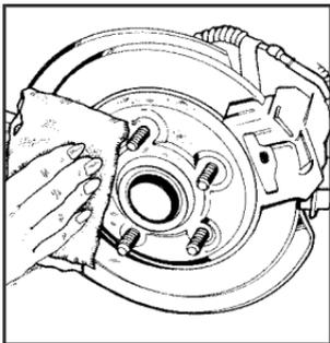
8. Remove any rust or dirt from the wheel bolts, mounting surfaces and spare wheel.
