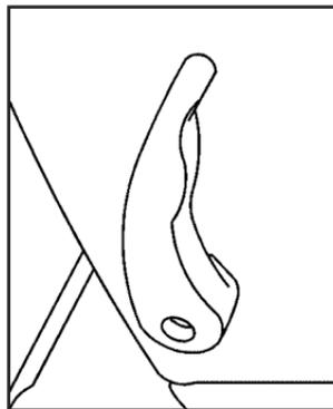
To fold the seatback forward, push the lever on the side of the seat rearward and pull the seatback forward.
