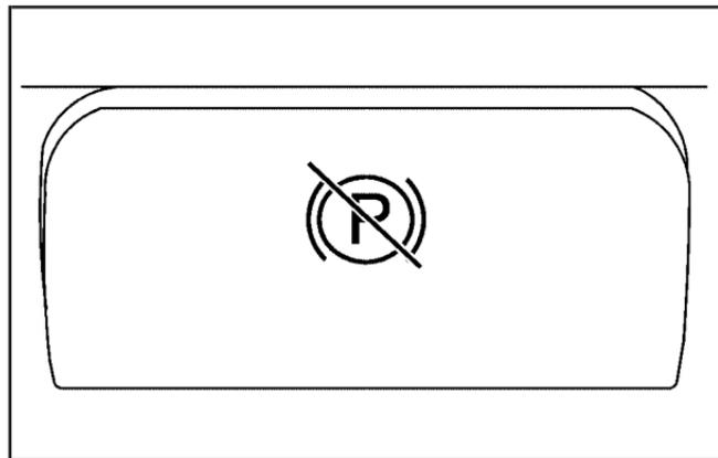
To release the parking brake, hold the regular brake pedal down. Pull the bottom edge of the lever, located above the parking brake pedal, with the parking brake symbol, directly rearward to release the parking brake.
