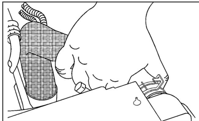
6. Start the engine and let it run until you can feel the upper radiator hose getting hot. Watch out for the engine cooling fan.
