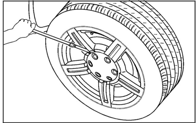
2. Remove the center cap by placing the chisel end of the wheel wrench (E) into one of the slots on the wheel and gently prying the cap out.
