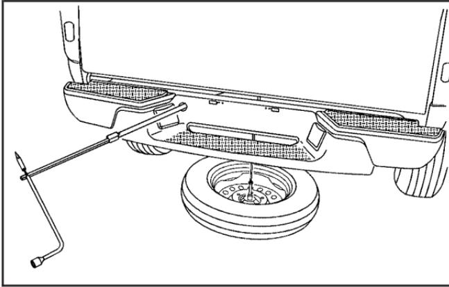
4. Insert the chiseled end of the jack handle at a slight angle through the hole in the rear bumper and into the funnel-shaped guide.
