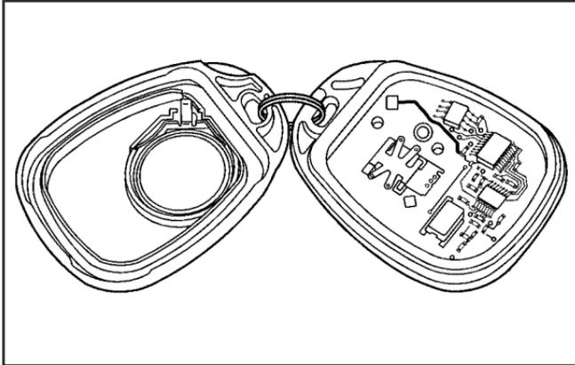
1. Separate the transmitter with a flat, thin object inserted in the slot between the covers of the transmitter housing.
