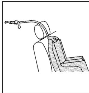
If the position you are using has a fixed headrest or head restraint and you are using a single tether, route the tether over the head restraint.
