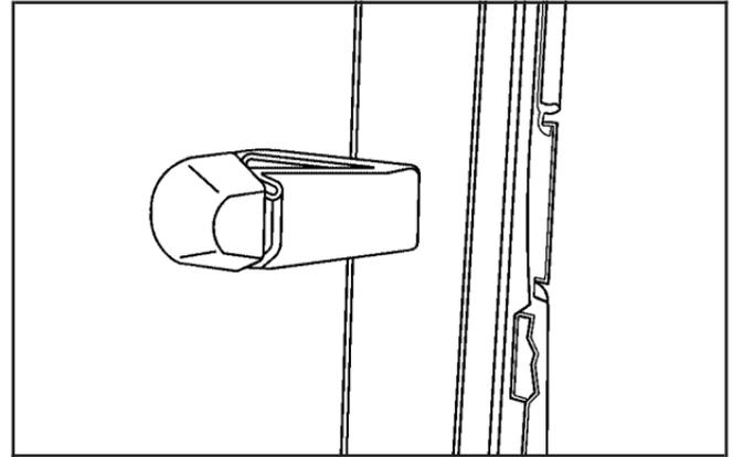
If the vehicle has this feature, squeeze the latch in the center of the window and slide the glass to open it. Be sure the latch is engaged when the window is closed.
