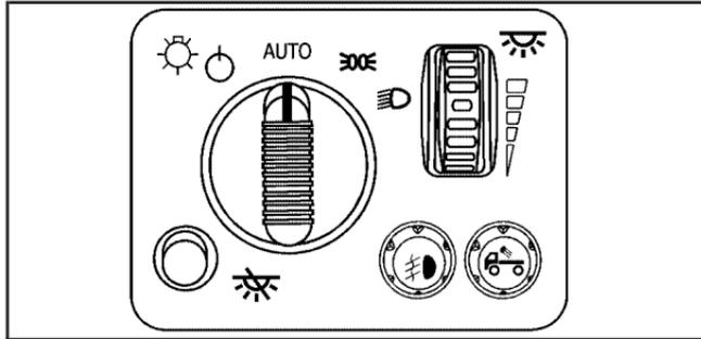
The exterior lamp control is located on the instrument panel on the left side of the steering wheel.
