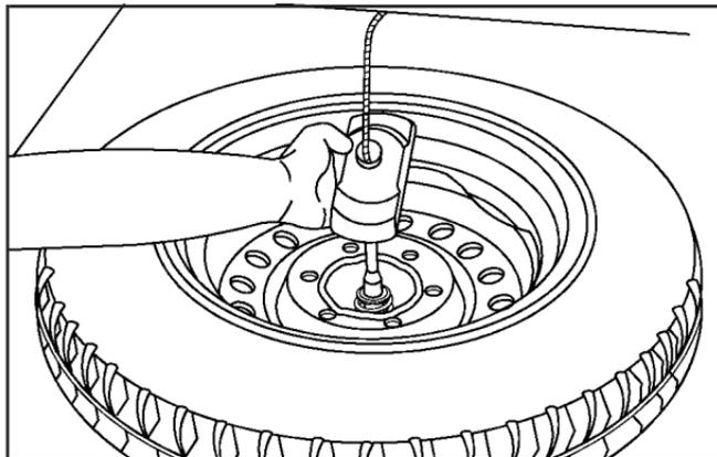
2. Tilt the retainer downward and through the center wheel opening. Make sure the retainer is fully seated across the underside of the wheel.
