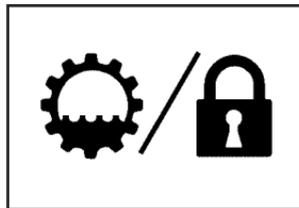
The automatic transmission dipstick handle with this symbol on it is located in the engine compartment on the passenger side of the vehicle.
