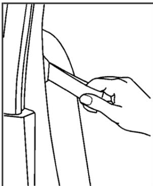
2. Pull the loop, located on the outboard side of the seatback, forward until you hear a click.
