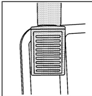
The parking brake pedal is located to the left of the brake pedal, near the driver door.
