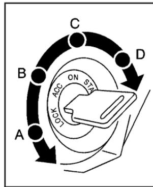
The ignition switch has four different positions.
