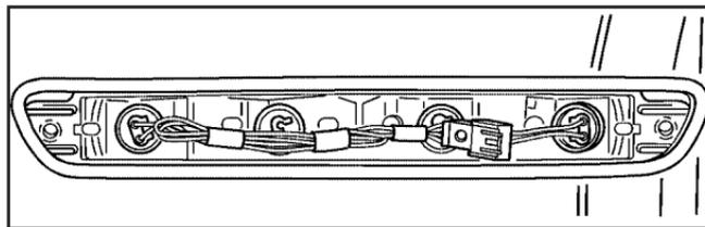
2. Turn the bulb socket counterclockwise and remove it from the lamp assembly.
