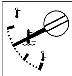
This gage shows the engine coolant temperature.
