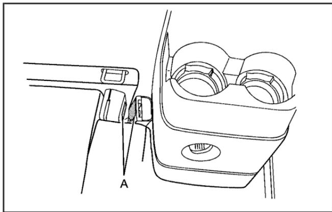
1. Secure the safety belt buckle to the inboard side of the seat with the hook and loop fastener (A), so that it does not move when not in use.
