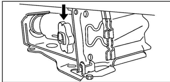
2. Turn the jack knob counterclockwise to lower the jack all the way and release it from the bracket.
