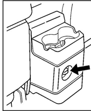
1. Turn the wing nut on the cover counterclockwise to remove it.
