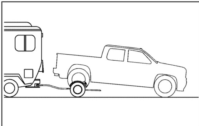
Use the following procedure to dolly tow a four-wheel-drive vehicle from the rear:
