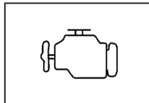
This light should come on when the ignition is on, but the engine is not running, as a check to show it is working. If it does not, have the vehicle serviced by your dealer/retailer.
