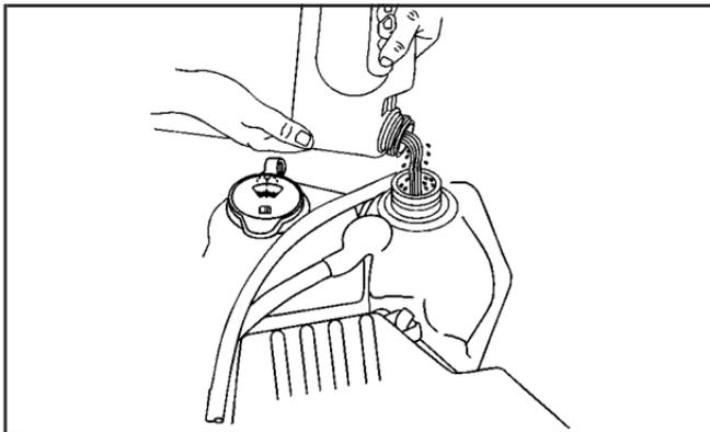
4. Fill the coolant recovery tank to the FULL COLD mark.
