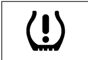
For vehicles with a tire pressure monitoring system, this light comes on briefly when the engine is started.
