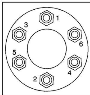
12. Tighten the wheel nuts firmly in a crisscross sequence as shown by turning the wheel wrench clockwise.
