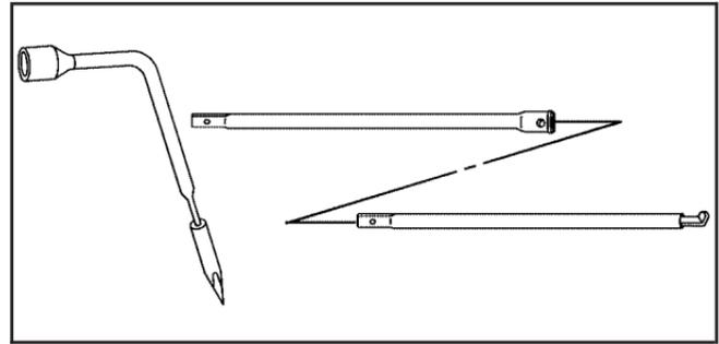
1. Assemble the wheel wrench (D), the jack handle extensions (A) and the jack handle (C) as shown.
