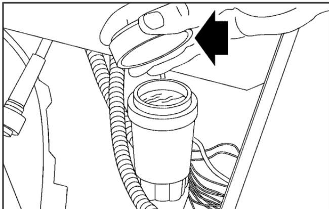
Refer to the Maintenance Schedule to determine how often to check the fluid level in the clutch master cylinder reservoir and for the proper fluid. See *Recommended Fluids and Lubricants* on page 6-12.
