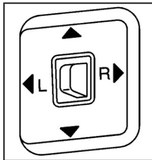
Vehicles with outside power mirrors have controls on the driver door armrest.
