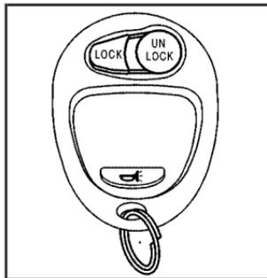
**UNLOCK:** Press to unlock the driver door and turn on the interior lamps. The parking lamps may flash and the horn may sound.
