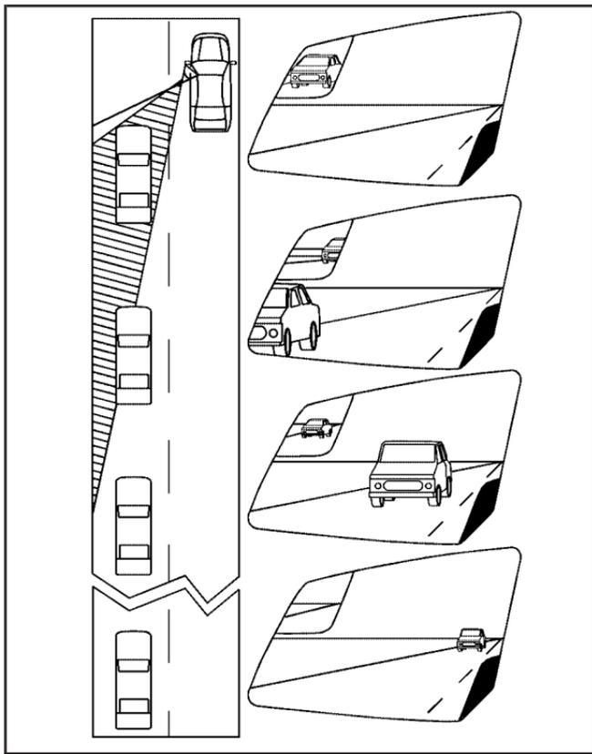
1. When the approaching vehicle is a long distance away, the image in the main mirror is small and near the inboard edge of the mirror.
