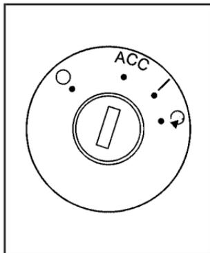
The ignition switch has four different positions.
