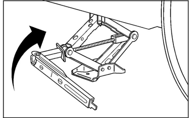
4. Raise the vehicle by turning the jack handle clockwise. Raise the vehicle far enough off the ground so there is enough room for the tire.
