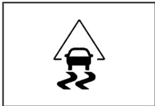
This light flashes while the traction control system is limiting wheel spin.
