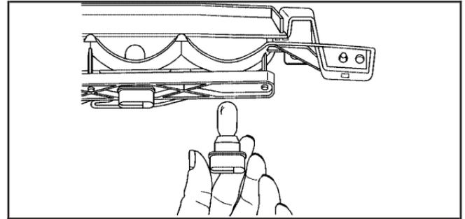
4. Pull the old bulb straight out of the bulb socket.
