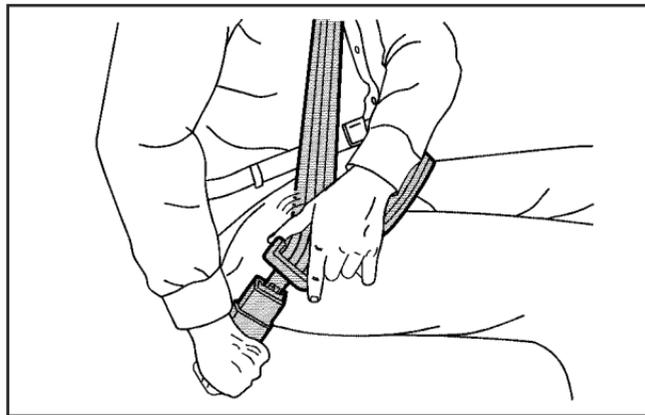
3. Push the latch plate into the buckle until it clicks. Pull up on the latch plate to make sure it is secure. If the belt is not long enough, see *Safety Belt Extender* on page 1-31. Position the release button on the buckle so that the safety belt could be quickly unbuckled if necessary.
