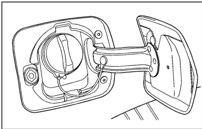
The tethered fuel cap is located behind a hinged fuel door on the passenger side of the vehicle. If the vehicle has E85 fuel capability, the fuel cap will be yellow and state that E85 or gasoline can be used. See *Fuel E85 (85% Ethanol)* on page 5-7.
