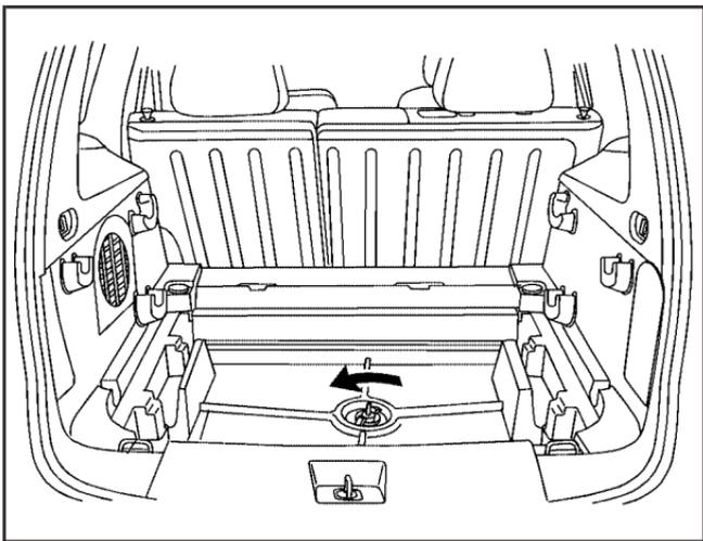
3. Turn the retainer counterclockwise to remove the tire cover.
