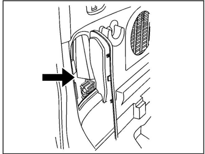
2. Remove the cover in the rear cargo area of the vehicle to access the bulbs.
