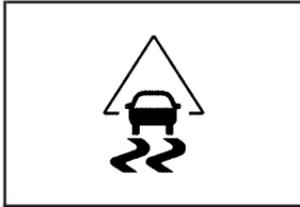
The Electronic Stability Control (ESC) system or the Traction Control System (TCS) indicator/warning light comes on briefly when the engine is started.
