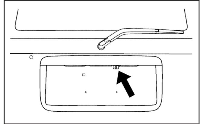
The area displayed by the camera is limited and does not display objects that are close to either corner or under the bumper. The area displayed can vary depending on vehicle orientation or road conditions. The distance of the image that appears on the screen differs from the actual distance.
