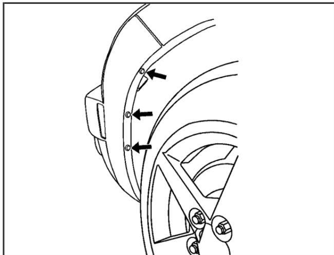
2. Remove the fasteners located on the wheel liner.
