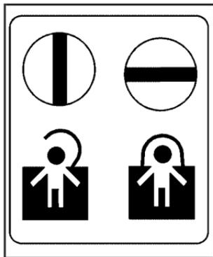
On vehicles with this feature, the rear door security locks are located on the inside edge of each rear door. You must open the rear doors to access them.
