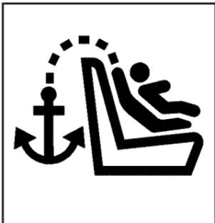
To assist you in locating the top tether anchors, this symbol will be located on the lower side quarter panels for the rear outboard positions, on the storage compartment for the rear center position and on the cargo mat behind the rear seats.
