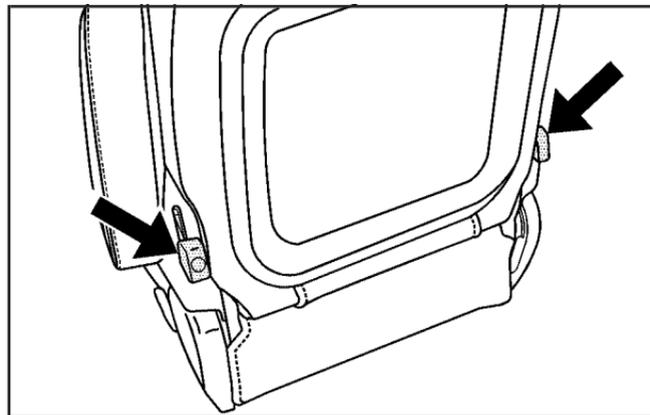
3. To fold the seat flat, pull up on either lever located toward the rear of the seatback. Fold the seat forward until the seatback disengages.
