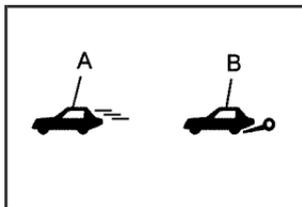
This indicator comes on when Competitive Driving Mode (A) has been set using the traction control switch. This telltale comes on whenever conditions are right for the Launch Mode (B) to activate.
