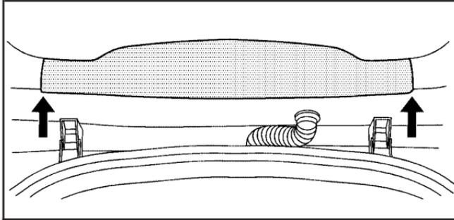
2. Remove the center trim located near the top of the liftgate.
