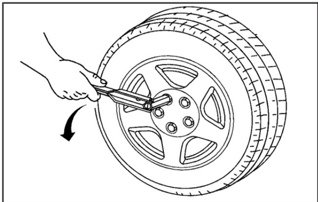
2. Using the wheel wrench, loosen all the wheel nuts. Do not remove them yet.
