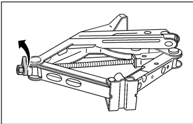
Turn the plastic wheel nut counterclockwise to loosen the wheel wrench from the jack.
