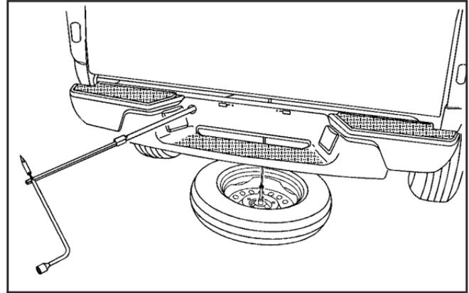
2. Insert the chiseled end of the jack handle (C) at a slight angle through the hole in the rear bumper and into the funnel-shaped guide.
