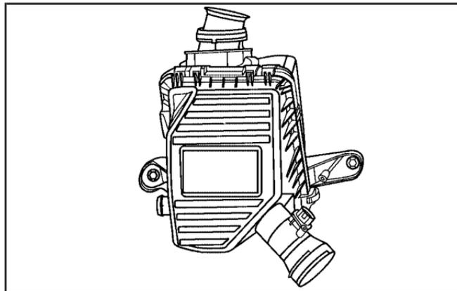
The engine air cleaner/filter is located in the engine compartment on the passenger's side of the vehicle. See *Engine Compartment Overview on page 6-12* for more information on location.
