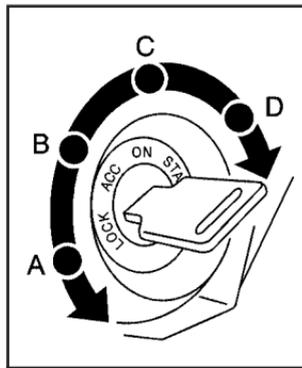
The ignition switch has four different positions.
