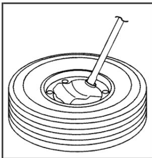
4. Tilt the retainer when the tire has been lowered, and slide it up the cable so it can be pulled up through the wheel opening.
