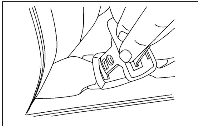
1. Disconnect the rear center safety belt latch from the mini buckle by inserting the tip of the safety belt retract into the slot on the buckle. Let the belt retract.
