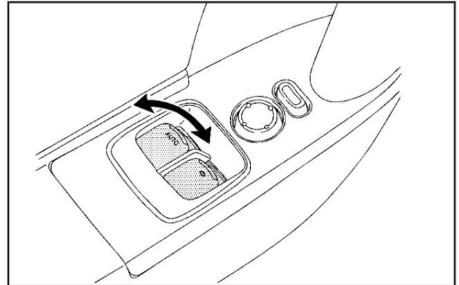
On vehicles with power windows, the switches on the driver's door armrest control both windows.
