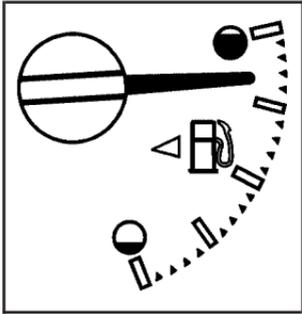
When the ignition is on, the fuel gage shows how much fuel the vehicle has remaining in the fuel tank.
