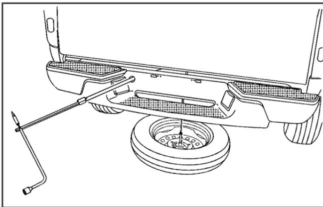
11. Remove the jack handle and insert the hoist end of the extension through the hole in the rear bumper. Turn the wheel wrench counterclockwise one turn or until the wheel retainer assembly is disengaged.
