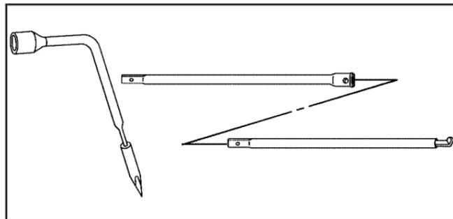
3. Assemble the wheel wrench, the jack handle extensions, and the jack handle as shown.
