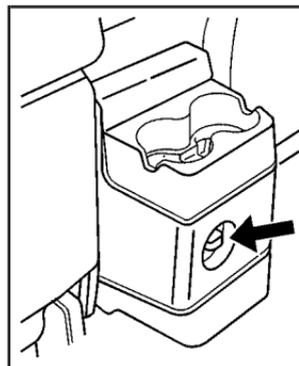
5. Put the cover in position and insert and tighten the wing nut to secure it.
