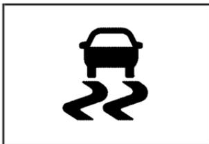
The StabiliTrak/TCS light will flash on the instrument panel cluster when the TCS system or StabiliTrak is both on and activated.
