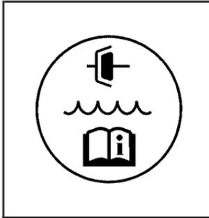
The hydraulic clutch fluid reservoir cap has this symbol on it. See *Engine Compartment Overview* on page 6-12 for reservoir location.
