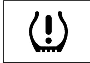
For vehicles with a tire pressure monitoring system, this light comes on briefly when the engine is started. It provides information about tire pressures and the Tire Pressure Monitoring System.
