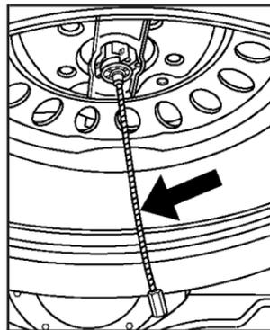
1. Check under the vehicle to see if the cable end fitting is visible.
