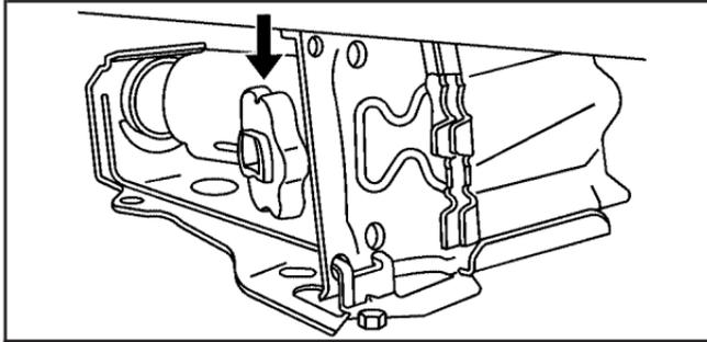
2. Turn the jack knob counterclockwise to lower the jack all the way and release it from the bracket.
