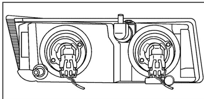
3. Turn the bulb socket counterclockwise to remove it from the headlamp assembly and pull it straight out.
