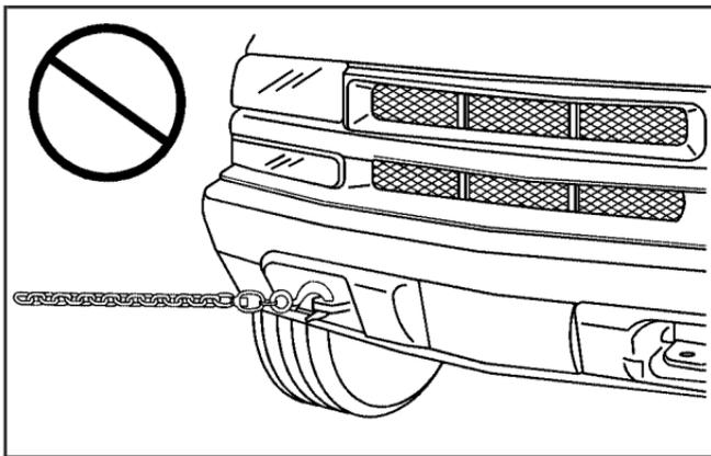
**Notice:** Never use recovery hooks to tow the vehicle. Your vehicle could be damaged and it would not be covered by warranty.
