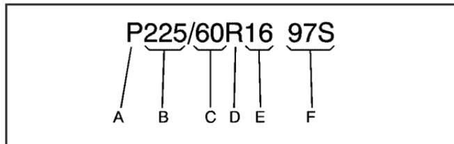
**(A) P-Metric Tire:** The United States version of a metric tire sizing system. The letter P as the first character in the tire size means a passenger vehicle tire engineered to standards set by the U.S. Tire and Rim Association.
