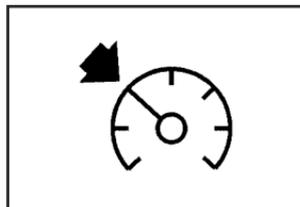
This light on the instrument panel cluster comes on while the cruise control is on.
