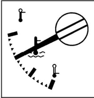
This gage shows the engine coolant temperature.
