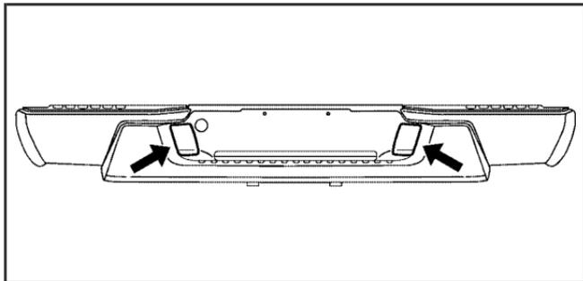
1. Reach under the rear bumper for the bulb socket.
