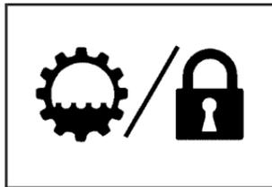
The automatic transmission dipstick handle with this symbol on it is located in the engine compartment on the passenger side of the vehicle.
