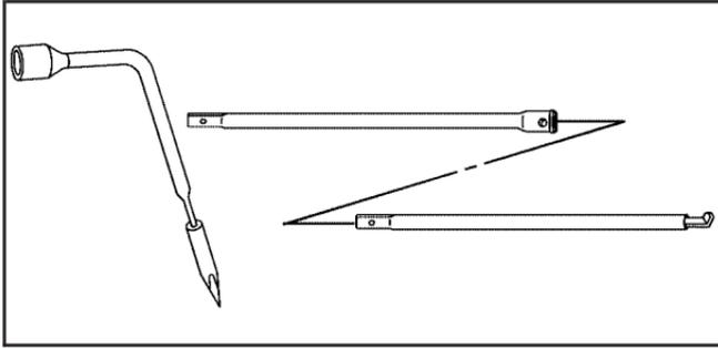
1. Assemble the wheel wrench (D), the jack handle extensions (A) and the jack handle (C) as shown.
