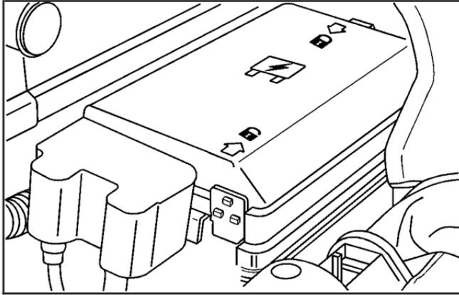
The engine compartment fuse block is located on the driver side of the engine compartment. See *Engine Compartment Overview* on page 6-12 for more information on location.
