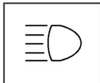
This indicator light turns on in the instrument panel cluster when the high beam headlamps are on.
