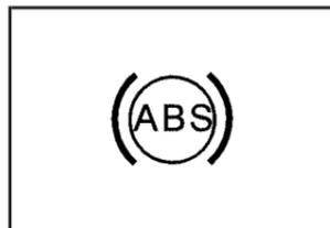
The Antilock Brake System (ABS) light comes on briefly when the engine is started.
