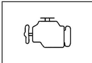
This light should come on when the ignition is on, but the engine is not running, as a check to show it is working. If it does not, have the vehicle serviced by your dealer/retailer.
