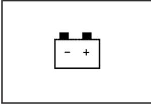
This light comes on briefly when the ignition key is turned to START, but the engine is not running, as a check to show it is working.
