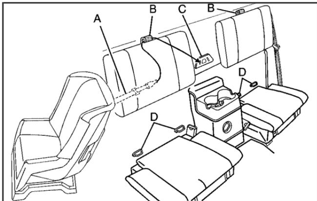
1. Attach and tighten the lower attachments to the lower anchors. If the child restraint does not have lower attachments or the desired seating position does not have lower anchors, secure the child restraint with the top tether and the safety belts. Refer to your child restraint manufacturer instructions and the instructions in this manual.
