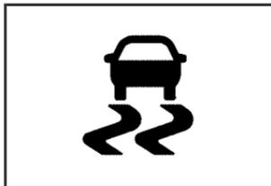
The StabiliTrak and Traction Control System (TCS) indicator/warning light comes on briefly while starting the engine.
