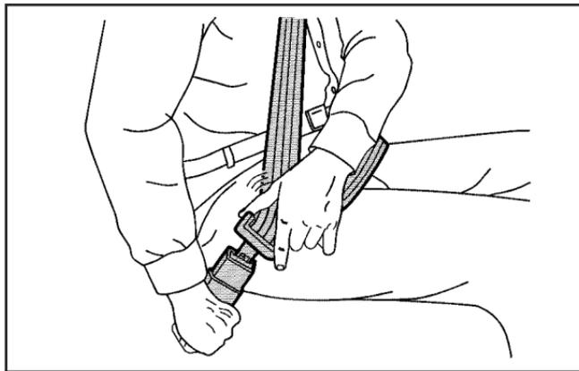
3. Push the latch plate into the buckle until it clicks. Pull up on the latch plate to make sure it is secure. If the belt is not long enough, see *Safety Belt Extender on page 2-33*.
