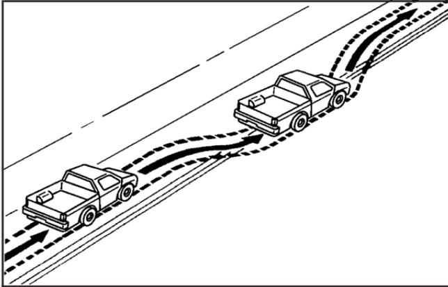
If the level of the shoulder is only slightly below the pavement, recovery should be fairly easy. Ease off the accelerator and then, if there is nothing in the way, steer so that the vehicle straddles the edge of the pavement. Turn the steering wheel 8 to 13 cm, 3 to 5 inches, (about one-eighth turn) until the right front tire contacts the pavement edge. Then turn the steering wheel to go straight down the roadway.
