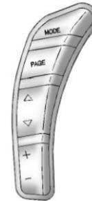
The HUD controls are located to the left of the steering wheel.
