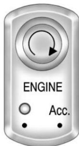
The vehicle has an electronic keyless ignition with a push-button start.
