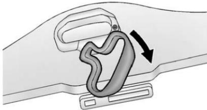
3. Release the convertible top front latch, located above the inside rearview mirror,
