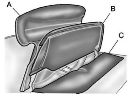
5. Lift upward on the front edge (A) of the convertible top to remove it from the windshield frame. Then lift upward on the rear edge (B) of the convertible top so it is vertical to the tonneau cover (C). The front edge (A) and rear edge (B) should be straight up.
