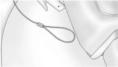
1. Open the tonneau cover by pulling the manual release cable.
