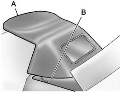
9. Push forward on the front edge (A) of the convertible top to allow the rear edge (B) of the convertible top to be moved to its full-down position.
