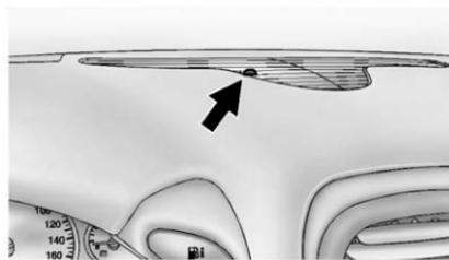
Be sure not to cover the light sensor on the top of the instrument panel.
