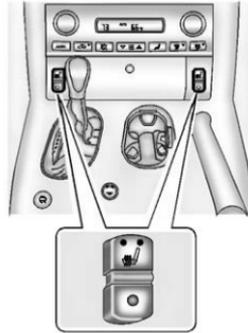
If available, the buttons are on the center stack. The ignition must be on for this feature to work.
