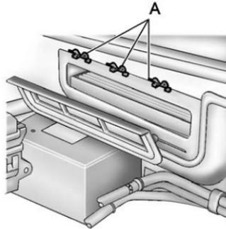
1. Remove the cover retainer clips (A) from the passenger compartment air filter cover.
