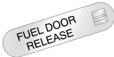
There is also a manual fuel door release tab. It is located against the upper trim in the rear compartment on the driver side of the vehicle. Pull the tab to release the fuel door.
