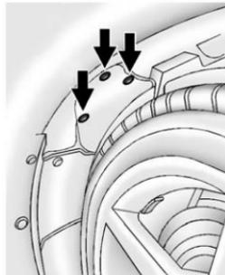
2. Remove the three outer fasteners to move the access panel back.
