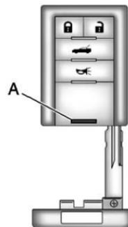
Press the button (A) near the bottom of the RKE transmitter to remove the key. Never pull the key out without pressing the button.
