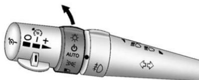
The exterior lamp control is located to the left of the steering wheel on the multifunction lever.
