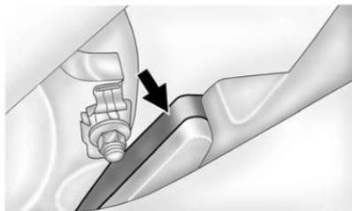
The ZR1, Z06, and Grand Sport models also have an electronic brake pad wear sensor system. When pads are worn, the CHANGE BRAKE PADS message displays in the Driver Information Center. See *Brake System Messages* on page 5-36.
