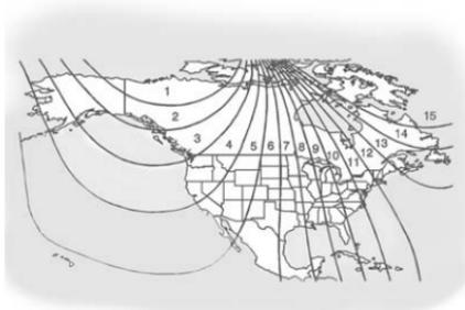
2. Press and hold
