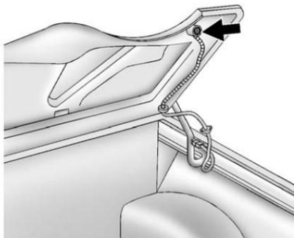
7. Tilt the driver seatback forward and press the tonneau cover release button located on the underside of the tonneau cover (C) behind the driver seat. After pressing the release button, the driver and passenger door glass will retract to the full-down position. Then raise the tonneau cover (C).
