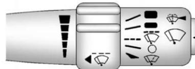
The windshield wiper/washer lever is located on the right side of the steering column.
