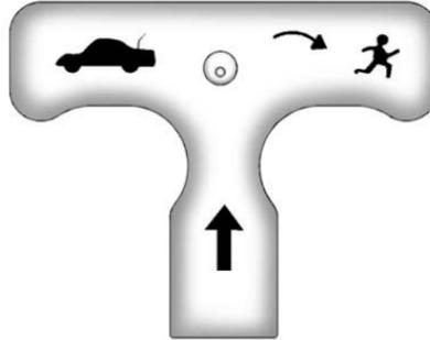
**Notice:** Do not use the emergency trunk release handle as a tie-down or anchor point when securing items in the trunk as it could damage the handle.
