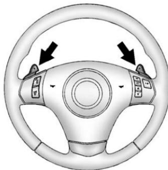
The Manual Paddle Shift system is activated from S (Sport Mode) by pushing the paddle, above the steering wheel spokes, to up-shift to the next gear, or pulling on the paddle, behind the steering wheel spokes, to down-shift to the next gear.
