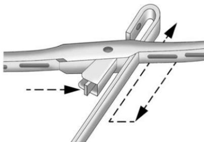
2. Lift up on the plastic latch in the middle of the wiper blade where the wiper arm attaches.
