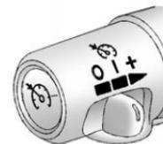
The cruise controls are located at the end of the multifunction lever.
