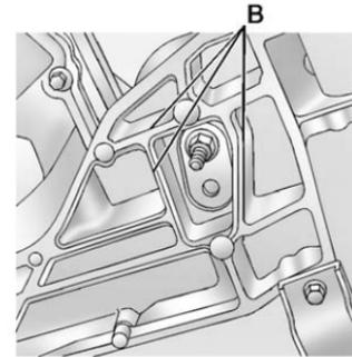
3. Lift the vehicle with the jack, making sure the jack spans at least two of the crossmember ribs (B).
