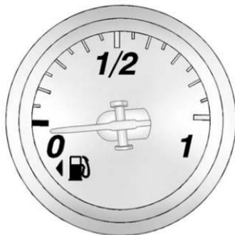
The fuel gauge shows how much fuel the vehicle has left while the engine is on.
