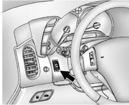
3. Push and hold  $\wedge$  on the convertible top switch. The convertible top will raise and the windows will lower if they were in the raised position. A chime will sound when the convertible top is raised completely.
