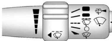
The windshield wiper/washer lever is located on the right side of the steering column.
