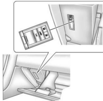
7. Place the new transmitter in the glove box transmitter pocket with the buttons facing the passenger side.
