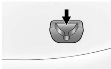
3. Gently place the roof panel down so that the back pins on the roof panel drop into the receivers in the back of the storage area.
