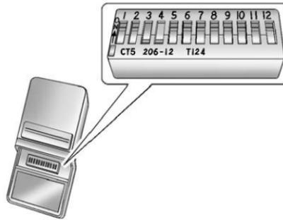
2. To verify that the garage door opener is a Fixed Code unit, remove the battery cover on the hand-held transmitter supplied by the manufacturer of the garage door opener motor. If there is a row of dip switches similar to the graphic above, the garage door opener is a Fixed Code unit. If you do not see a row of dip switches, return to the previous section, "Programming Universal Home Remote – Rolling Code."
