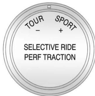
To select a mode while in Performance Traction Management, turn the knob located on the center console.
