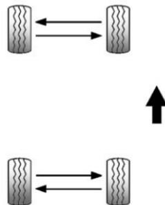
Use this rotation pattern if the vehicle has different size tires on the front and rear and they are non-directional.
