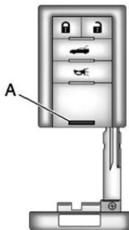
Press the button (A) to remove the key. The key can be used to lock and unlock the glove box and to open the hatch/trunk lid if power to the vehicle is lost. See *Hatch* on page 2-11 for more information.
