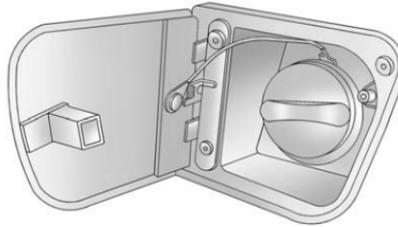
The tethered fuel cap is located behind a hinged fuel door on the driver side of the vehicle.
