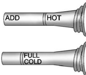
When the engine compartment is hot, the level should be at the HOT mark.
