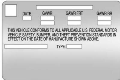
A vehicle-specific Certification label is attached to the rear edge of the driver door.
