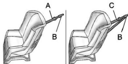
A top tether (A, C) anchors the top of the child restraint to the vehicle. A top tether anchor is built into the vehicle. The top tether attachment (B) on the child restraint connects to the top tether anchor in the vehicle in order to reduce the forward movement and rotation of the child restraint during driving or in a crash.
