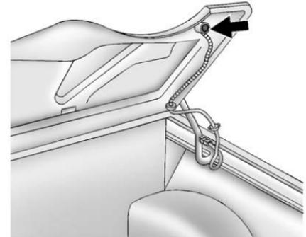
4. Tilt the driver seat forward and press the tonneau cover release button.
