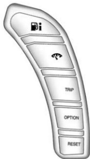
The DIC buttons are located on the instrument panel to the right of the instrument panel cluster.
