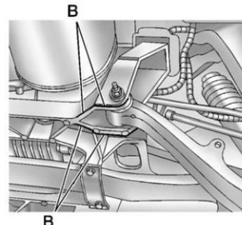
3. Lift the vehicle with the jack, making sure the jack spans at least two of the crossmember ribs (B).
