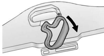
4. Release the convertible top front latch, located above the inside rearview mirror, by pulling and turning it clockwise.
