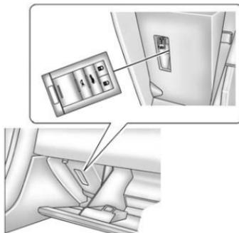
2. Place the new transmitter in the glove box transmitter pocket with the buttons facing the passenger side.
