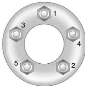
Tighten the wheel lug nuts firmly in a crisscross sequence.
