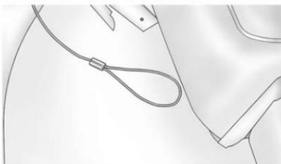
The tonneau cover manual release cable is located underneath the carpeting behind the passenger seat head restraint, on the underside forward edge of the tonneau cover. To access the cable, lift and pull back the carpeting.
