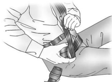
3. If the belt stops before it reaches the buckle, tilt the latch plate and keep pulling the safety belt until it can be buckled.
