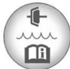
The hydraulic clutch fluid reservoir cap has this symbol on it. See *Engine Compartment Overview* on page 10-8 for reservoir location.
