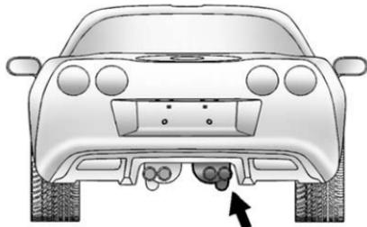
The rear lifting points can be accessed from the rear of the vehicle, on either the driver's or passenger's side.
